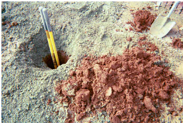
Figure 5-3. Installation of Thermocouples
