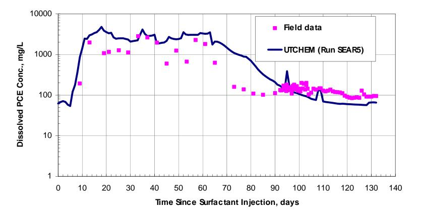
Figure 5-16. Comparison of Field and History Match Simulation Result of PCE Concentration for EX01
