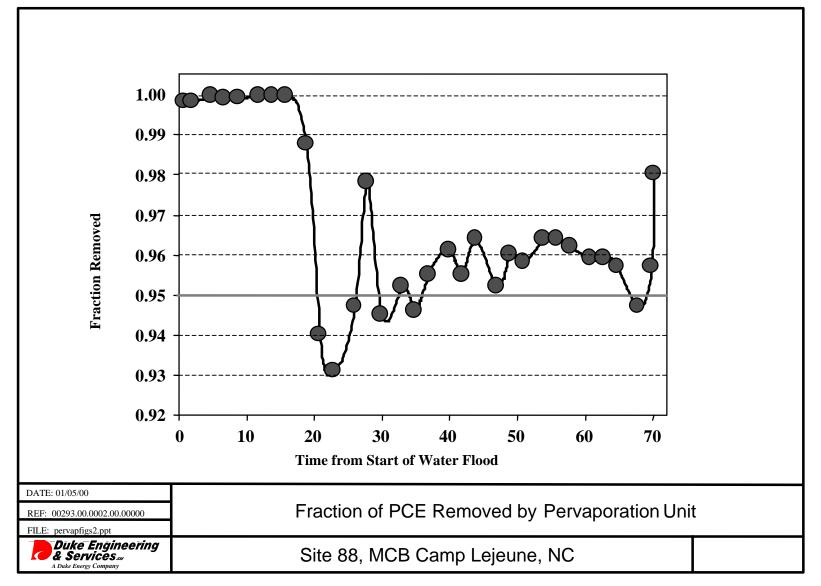
Figure 5-19. Fraction of PCE Removed by Pervaporation Unit
