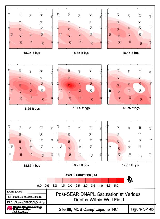
Figure 5-14b. Post-SEAR DNAPL Saturations at Various Depths Within the Well Field at Site 88, MCB Camp Lejeune, NC
