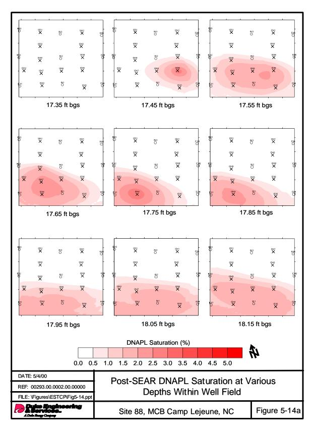
Figure 5-14a. Post-SEAR DNAPL Saturations at Various Depths Within the Well Field at Site 88, MCB Camp Lejeune, NC
