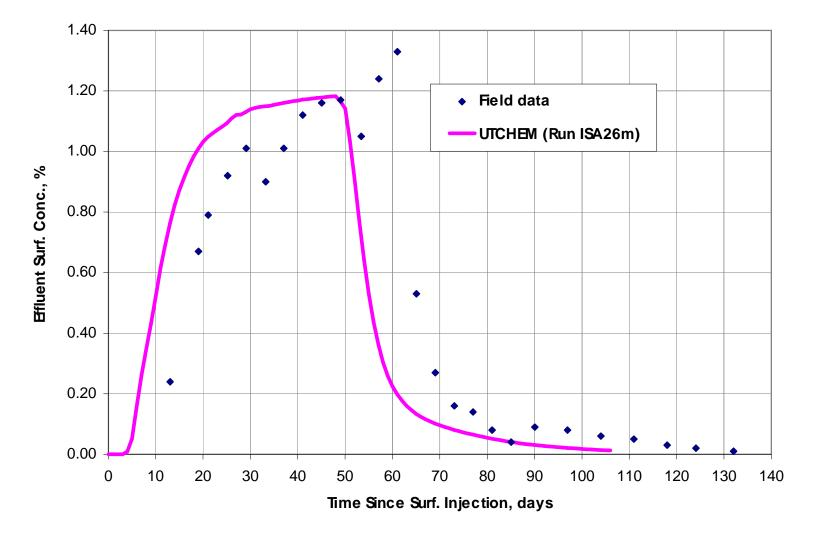
Figure 5-8. Comparison of Predicted and Field Surfactant Concentrations From EX01
