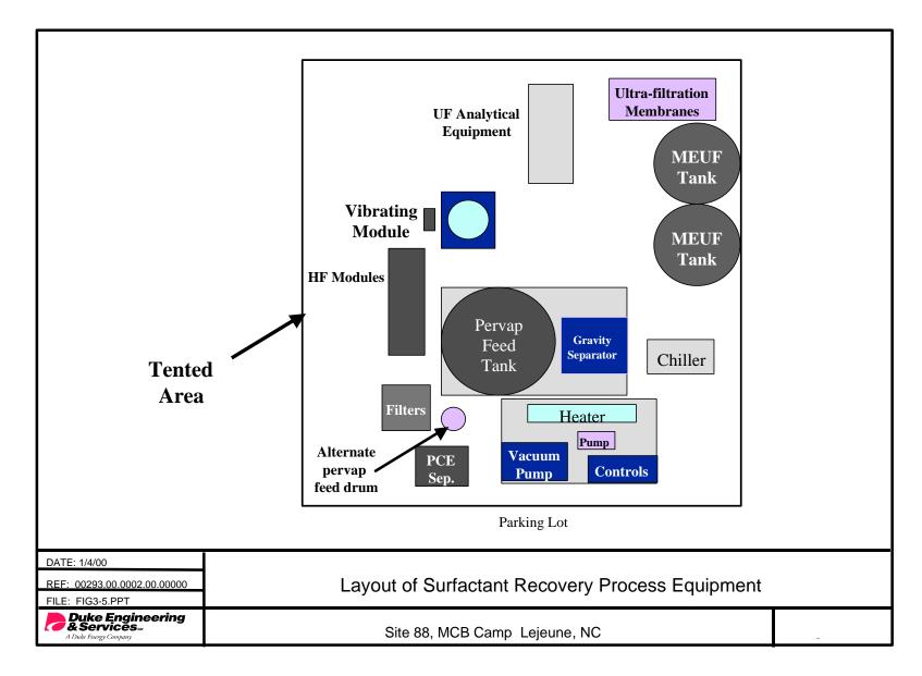
Figure 4-3. Layout of Surfactant Recovery Process Equipment
