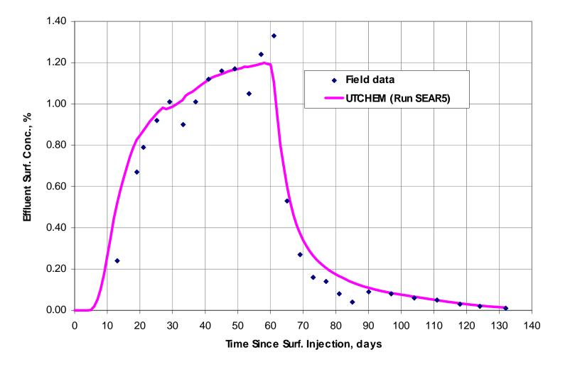
Figure 5-17. Comparison of Field and History Match Simulation Result of Surfactant Concentration for EX01
