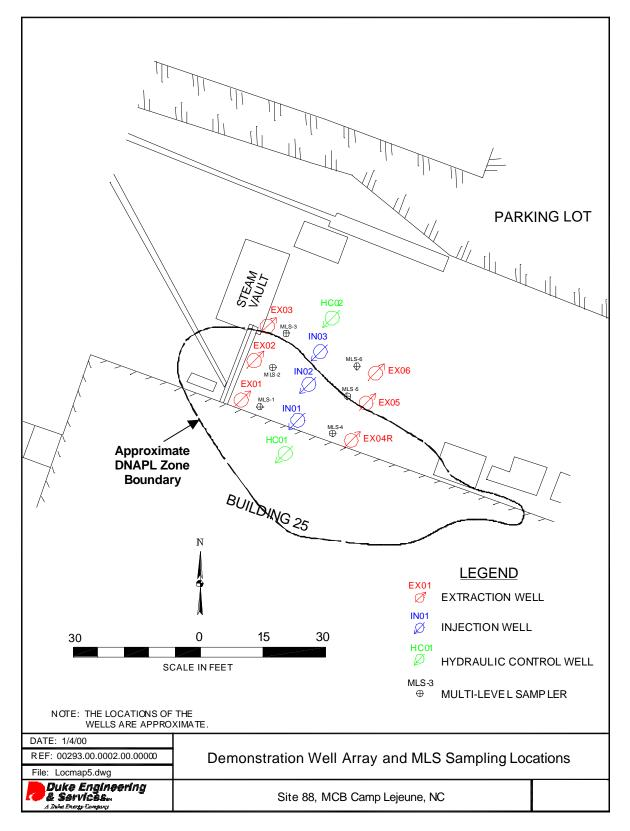
Figure 3-2. Demonstration Well Array and MLS Sampling Locations
