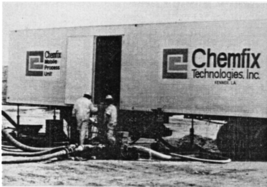
Figure 6-10. Enclosed mobile mixing plant (Courtesy Chemfix).
