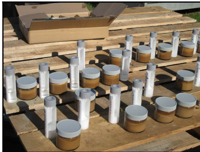
Figure 6.1: On-Site Gel Tests with Site Soils
