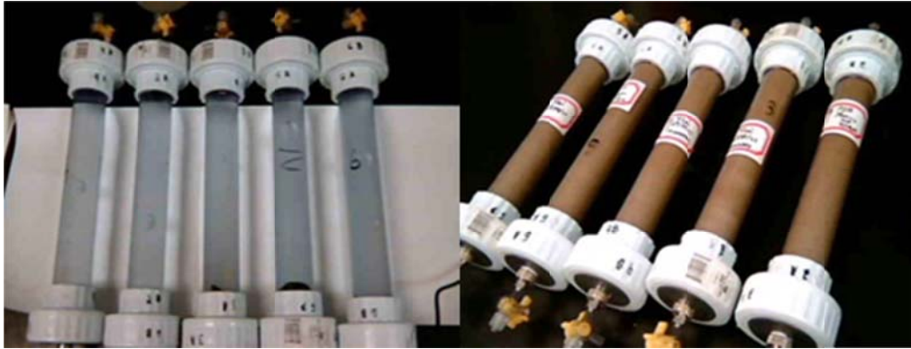
Figure 4. Empty and packed PVC columns used for injection tests.
