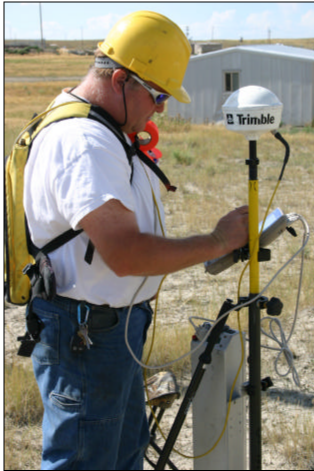
Figure 9. Taking measurements of the magnetic fields generated by current induced into the subsurface Shannon formation.
