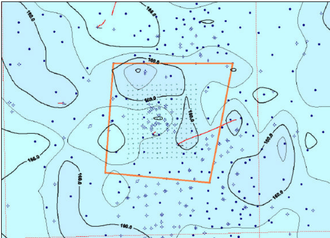
Figure 6. Isochore map showing the combined thickness of the upper and lower Shannon Sandstone members of the Steele Shale formation.
