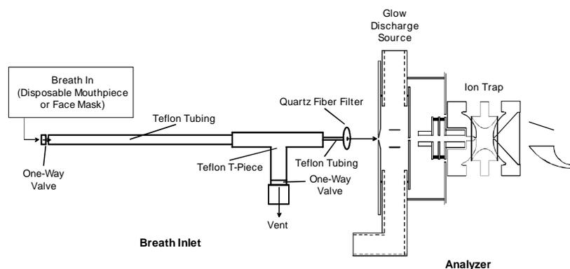
**Figure 4-3. Continuous real-time breath analyzer (RTBA), consisting of breath inlet (breath holding volume) attached to direct breath sampling interface (glow discharge ionization source) and ion trap mass spectrometer (GD/ITMS).**
