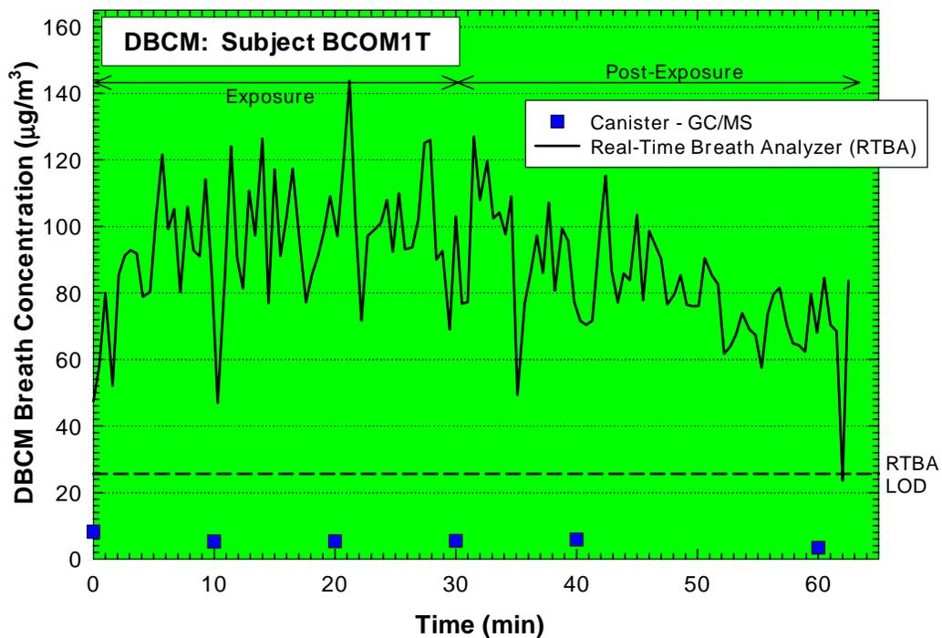
**Figure 5-4. Continuous exhaled breath concentrations for MTBE-d<sub>12</sub> (upper plot) and DBCM (lower plot) as a function of time for Subject BCOM1T during and following dermal exposure while bathing. Exposure duration was 34.1 min; post-exposure monitoring continued for another 31.0 min. Water temperature was 39.7°C. Nominal concentrations were 150 µg/L for MTBE-d<sub>12</sub> and 40 µg/L for DBCM. RTBA LOD designates detection limit with real-time breath analyzer.**
