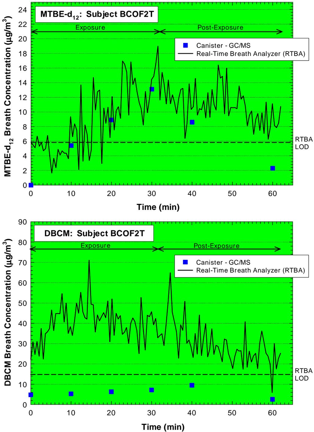
**Figure 5-7. Continuous exhaled breath concentrations for MTBE-d<sub>12</sub> (upper plot) and DBCM (lower plot) as a function of time for Subject BCOF2T during and following dermal exposure while bathing. Exposure duration was 33.0 min; post-exposure monitoring continued for another 29.5 min. Water temperature was 39.8°C. Nominal concentrations were 150 µg/L for MTBE-d<sub>12</sub> and 40 µg/L for DBCM. RTBA LOD designates detection limit with real-time breath analyzer.**
