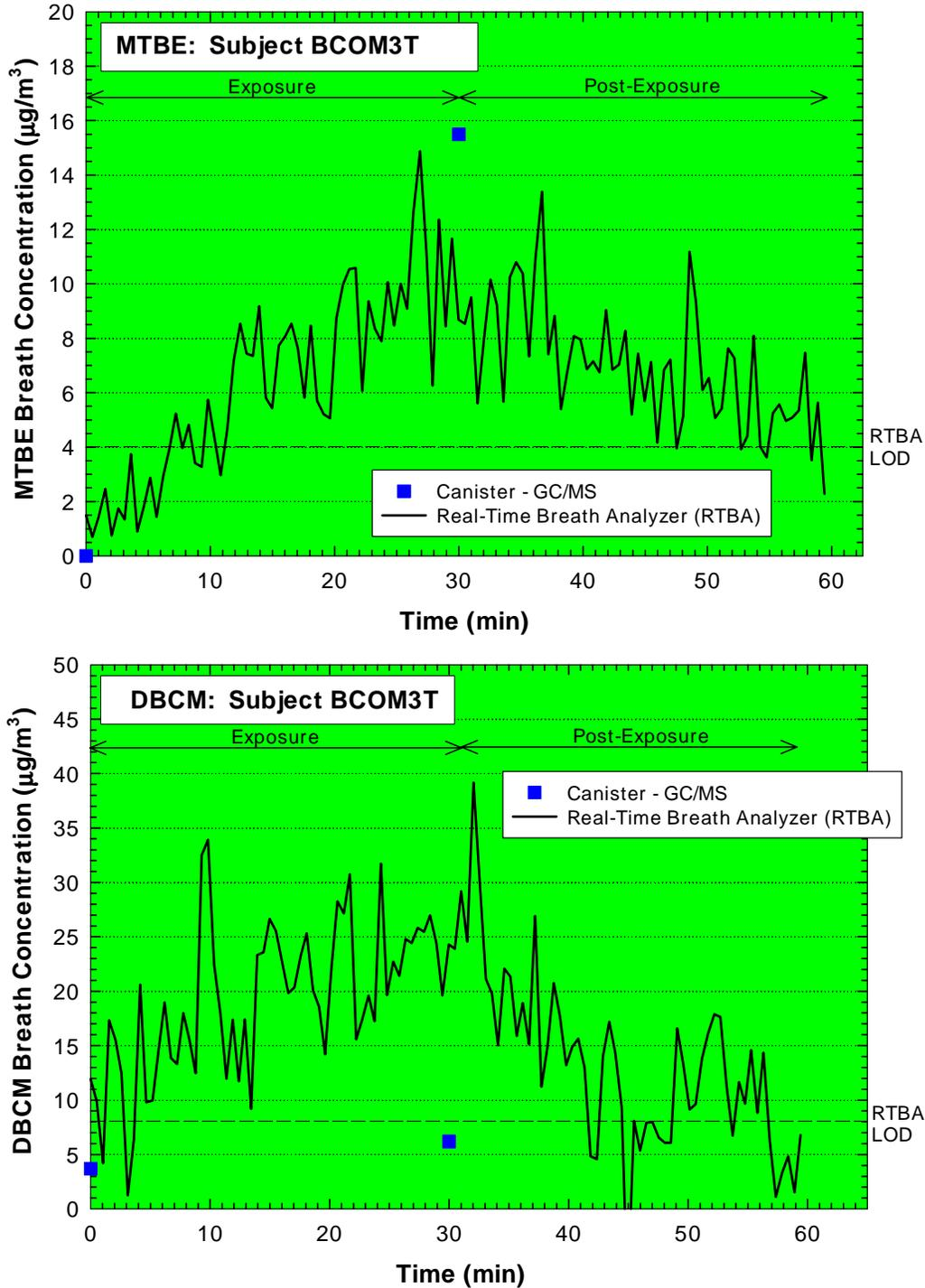
**Figure 5-8. Continuous exhaled breath concentrations for MTBE (upper plot) and DBCM (lower plot) as a function of time for Subject BCOM3T during and following dermal exposure while bathing. Exposure duration was 29.5 min; post-exposure monitoring continued for another 30.4 min. Water temperature was 40.4°C. Nominal concentrations were 150  $\mu\text{g}/\text{L}$  for MTBE and 40  $\mu\text{g}/\text{L}$  for DBCM. RTBA LOD designates detection limit with real-time breath analyzer.**
