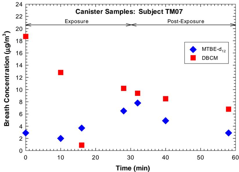
**Figure 5-2. Exhaled breath concentrations of MTBE-d<sub>12</sub> and DBCM as a function of time for Subject TM07 during and following dermal exposure while bathing. Data obtained from canister samples collected from real-time breath analyzer system. All samples analyzed by GC/MS. Nominal water concentration was 150 µg/L for MTBE-d<sub>12</sub> and 40 µg/L for DBCM; water temperature was 40°C.**
