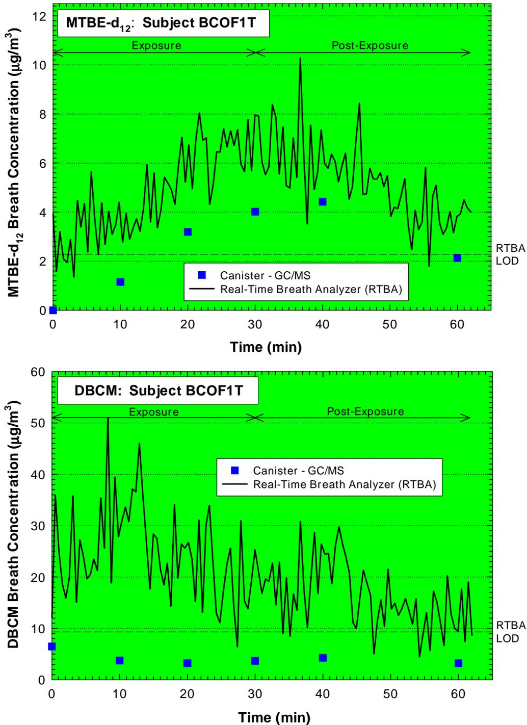
Figure 5-5. Continuous exhaled breath concentrations for MTBE-d<sub>12</sub> (upper plot) and DBCM (lower plot) as a function of time for Subject BCOF1T during and following dermal exposure while bathing. Exposure duration was 33.0 min; post-exposure monitoring continued for another 33.1 min. Water temperature was 39.0°C. Nominal concentrations were 150 µg/L for MTBE-d<sub>12</sub> and 40 µg/L for DBCM. RTBA LOD designates detection limit with real-time breath analyzer.
