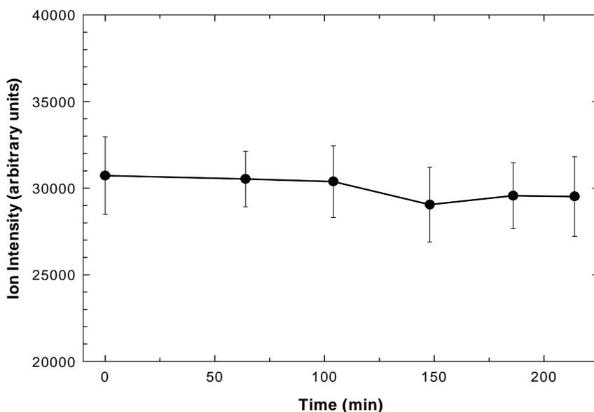
**Figure 5-19.** Plot of average ion signal (and standard deviation) at  $m/z$  55 as a function of time, obtained from constant source of 2-butanone in glass chamber at a concentration of  $866 \mu\text{g}/\text{m}^3$  in zero-grade air.
