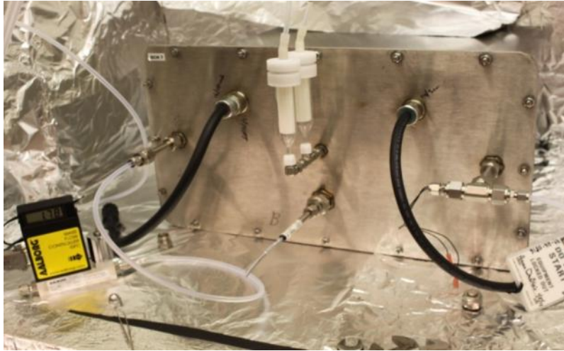
Figure 4.22. PUF sampling from the sealed 53-L chamber containing the burst ballast
