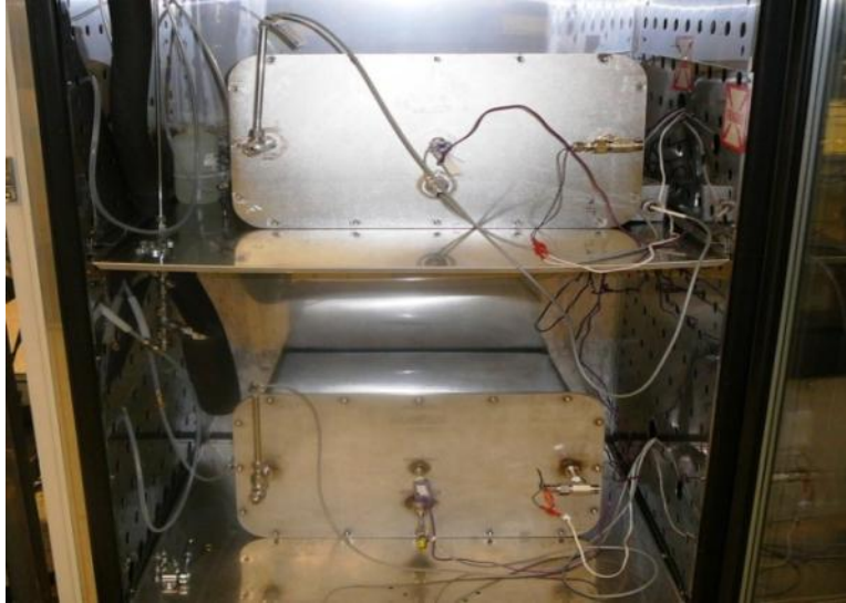
Figure E.2. Two 53-liter environmental chambers in the temperature-controlled incubator
