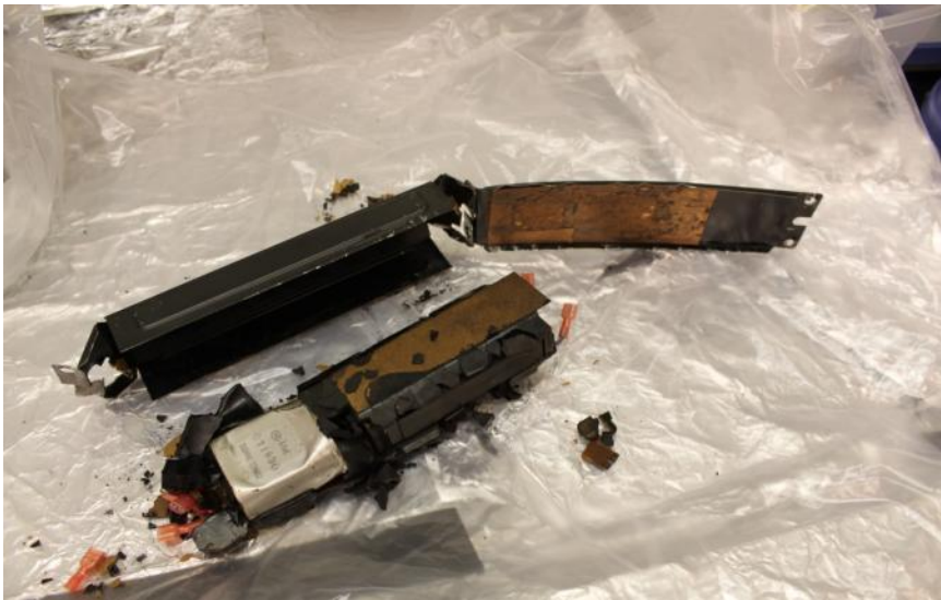
Figure 4.27. Ballast BL-12 after removing the casing (the capacitor is on the left)
