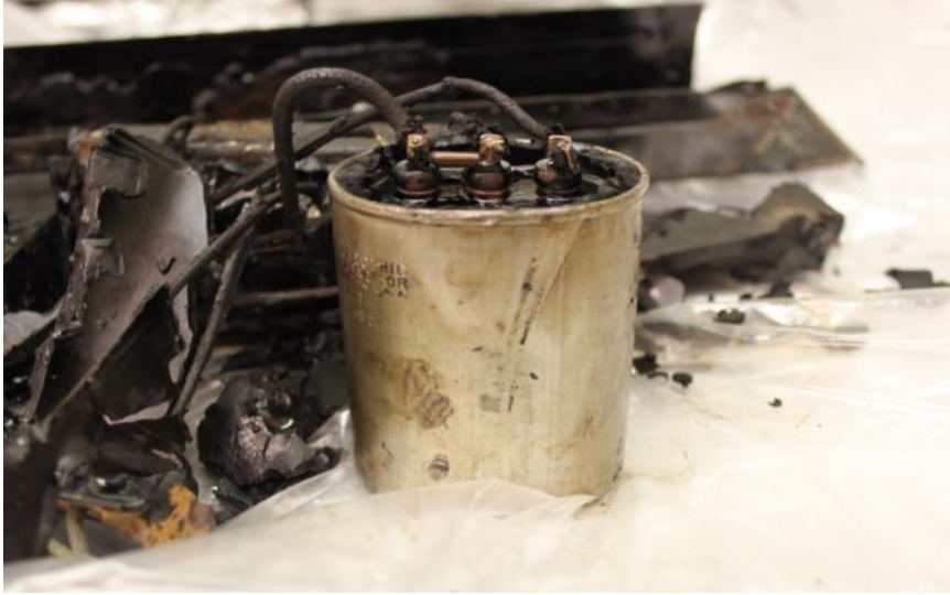
Figure 4.26. Capacitor in ballast BL-02
