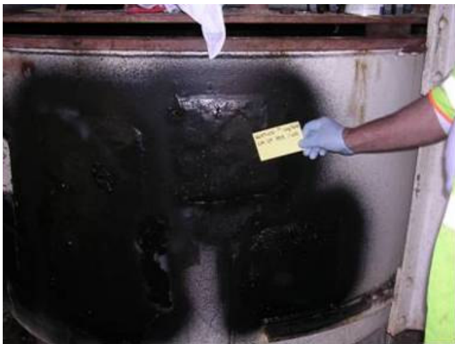
Figure 49. Large tank treated with MgPd-VP and NM-VP one week after application.
