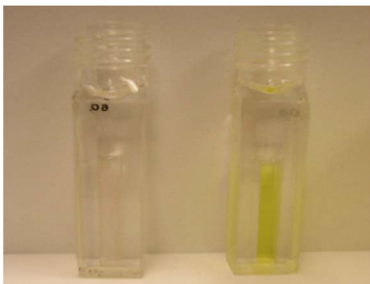
Figure 28. Mineral oil prevents the abiotic oxidation of NADH in the bioassay system by molecular oxygen
