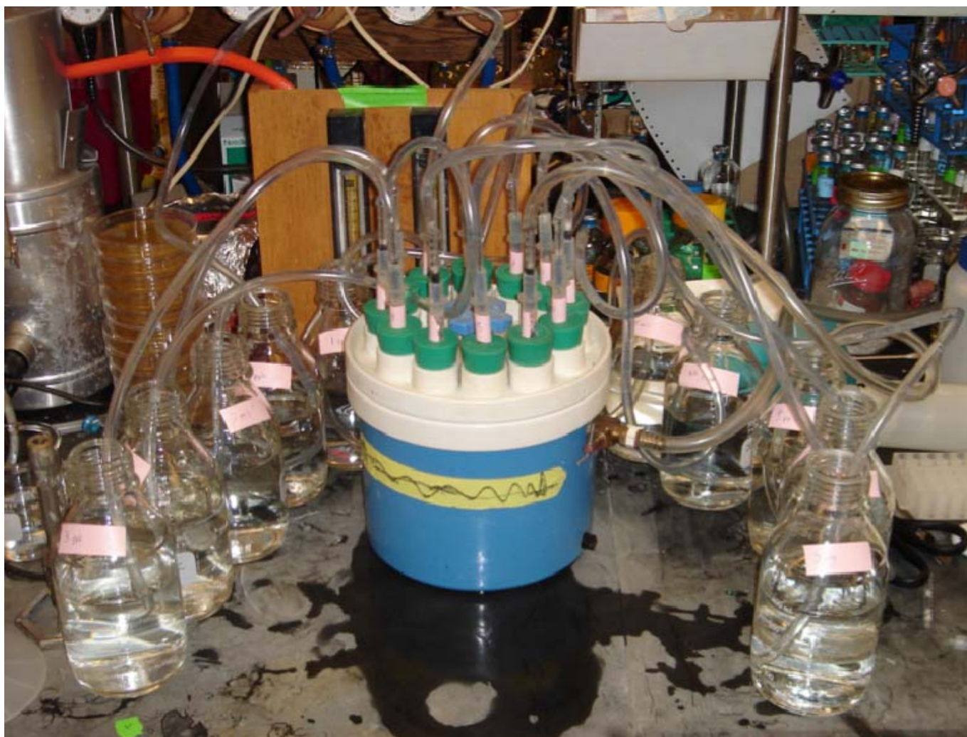
Figure 35. Millipore ultrafiltration device: A vacuum line was used to pull liquid through SDVB columns (in green stoppers). The liquid was collected in the bottom of the device and removed the black plug at the bottom of the apparatus.
