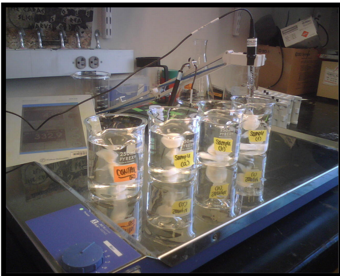
Figure 45. Extraction of perchlorate from 200ml samples using 1g of DTAB treated SDVB resin in teabags.
