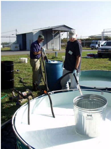
PHOTOGRAPH 1 Mixing of dilute EOS ® for injection.
