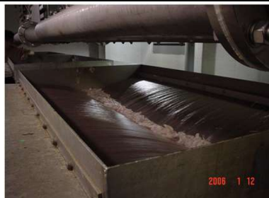
Figure 60. Picture of the electron beam accelerator and water interaction area for an industrial accelerator.
