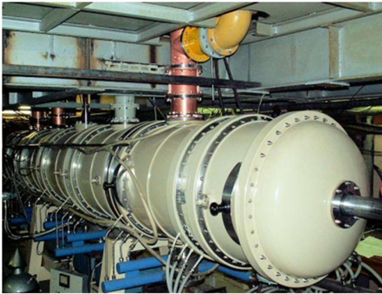
Figure 41. Industrial accelerator ILU-14. Electron beam energy is up to 10 MEV, beam power is 50 kW.
