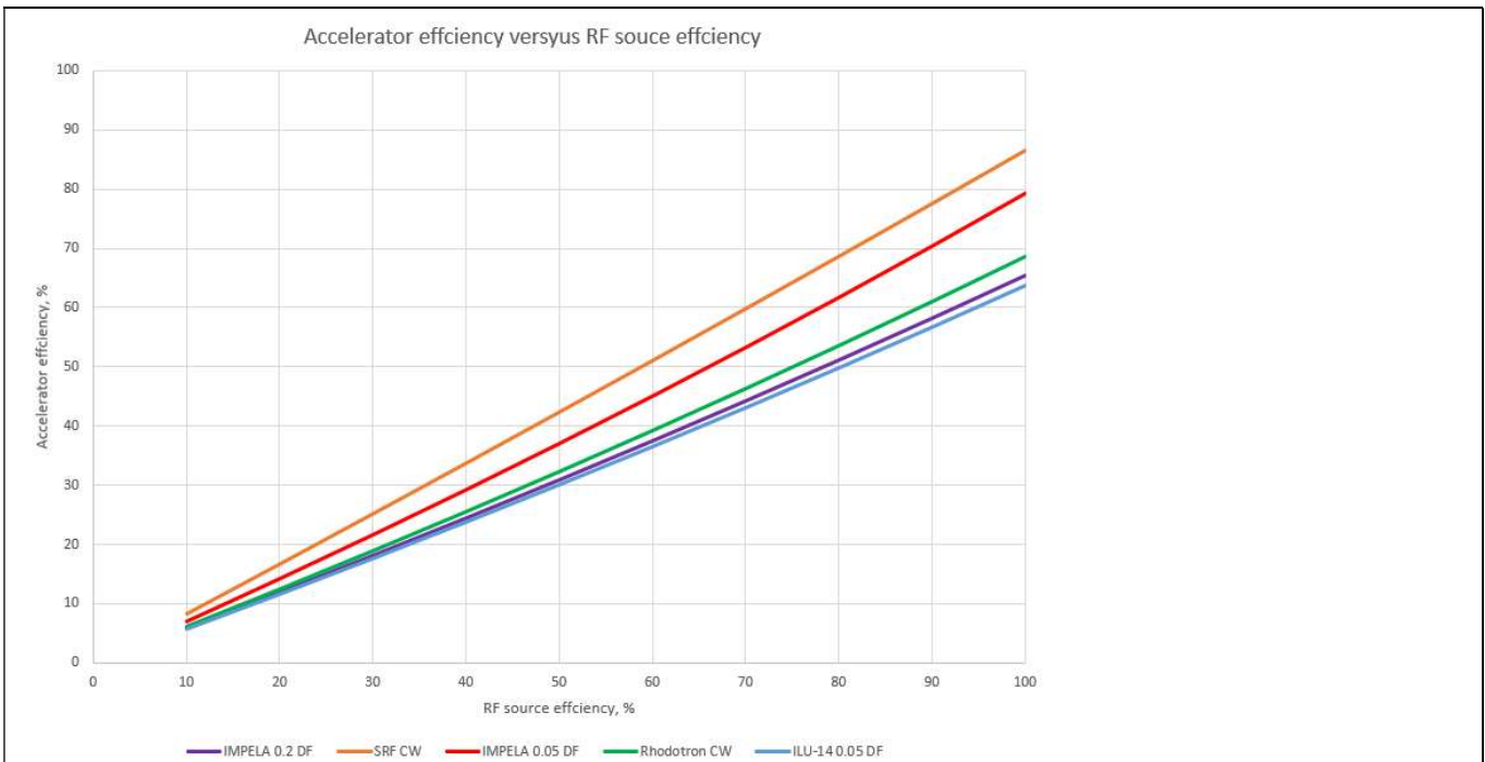
Figure 45. Wall-plug efficiency versus RF source efficiency for 400 kW
