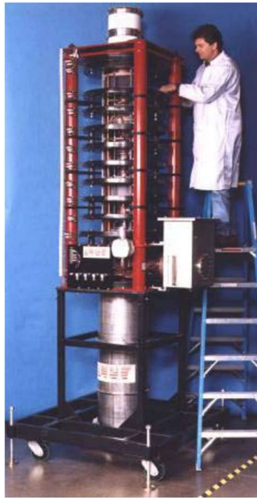
Figure 47. VKP-7958A 1MW CW 700 MHz Klystron for DESY 100
