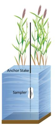
Figure 3. Depiction of Passive Sampler Deployed in an Example Surface Water Location.
