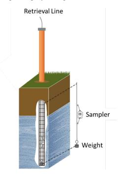
Figure 2. Depiction of Passive Sampler Deployed in a Groundwater Well.
