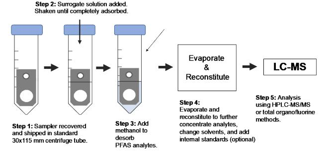
Figure 4. Diagram of the Extraction Process.
