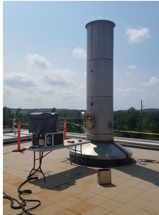
OTM-45 in use at incinerator stack
