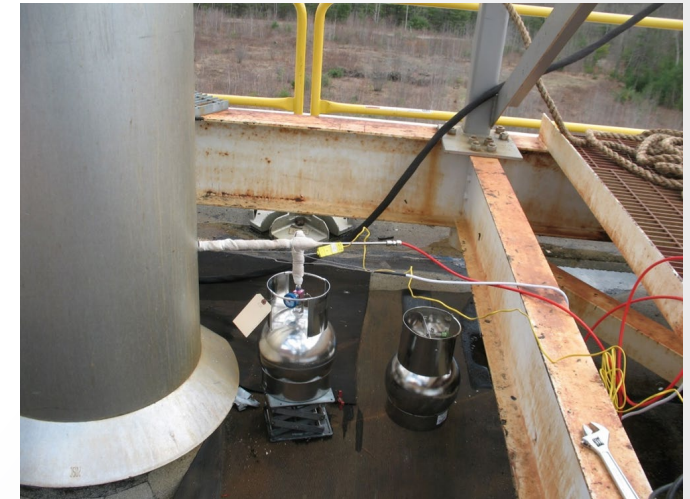
OTM-50 in use at incinerator stack
