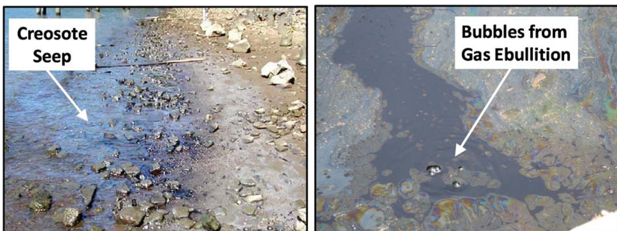
Figure 10. Illustrations of NAPL Pools or Sheens at Sites with Subsurface Discharge/Release of NAPL with Associated Hydrophobic Organic Contaminant (HOC). (Left Panel) Transport due to groundwater discharge (Oregon DEQ, 2006) and (Right Panel) transport due to gas ebullition (photo courtesy of Steve Mangion, U.S. EPA).
