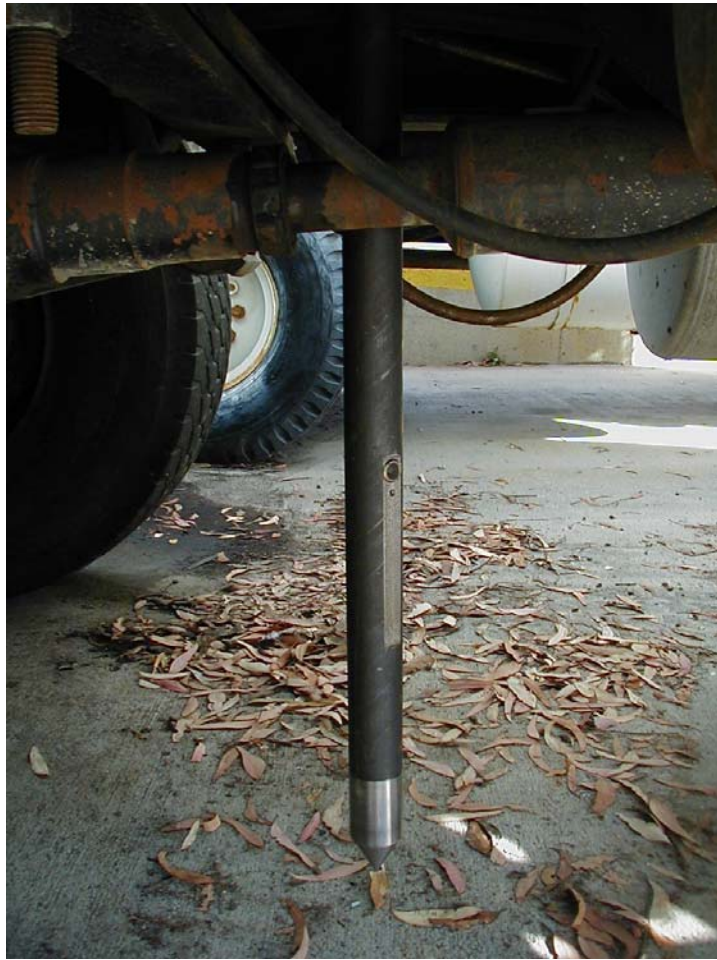
Figure 30. Probe in position ready for ground penetration.
