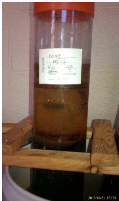
Figure 16. Laboratory set-up for intact cores from UCC. Strips of POM are used to assess the vertical gradient in resultant porewater concentrations.
