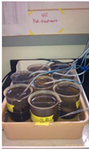
Bioaccumulation test set-up for exposure of Lumbriculus to wetland soils from UCC
