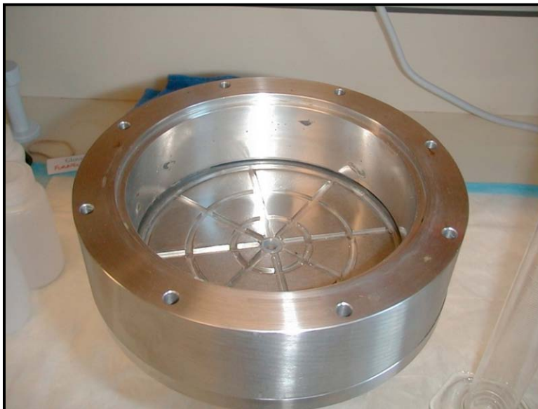
Figure 4.1-1. Experimental column for reactive mat flow-through testing.
