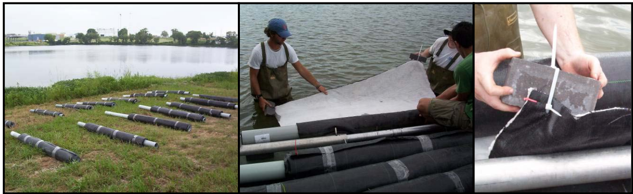
Figure 4.3-2. Small-scale geotextile test mat deployment.
