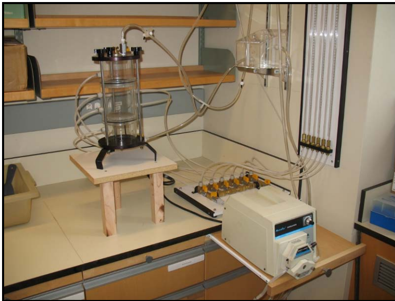
Figure 4.3-4. Geotextile sediment gradient ratio column experimental setup.
