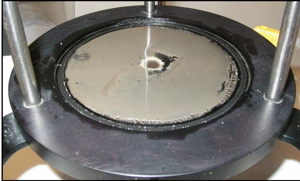
Figure 4.3-7. Sediment that has passed through the geotextile during a gradient ratio test.
