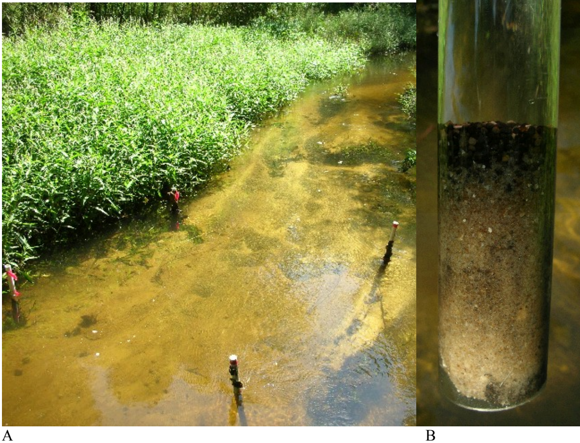
Picture 22. One Layer Cap Composed of Apatite (50%) and Sand (50%) in Creek Channel with High Flow One Month after Deployment. Erosion of the plot was visible within the first week (Picture A). After one month the cap material was transported up to 20 feet (Picture B) and about one or two inches of native sediment was deposited on the top of cap.
