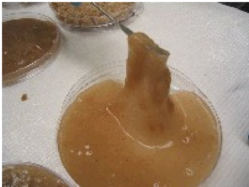
Picture 15. Adhesive Product of Sand Coated with Guar Gum Cross-linked by Borax.
