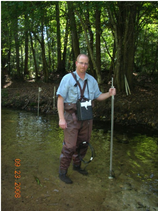
Picture 4. Measurement of Water Flow with Portable Water Flow Meter (Marsh-McBirney, Inc., Model 201).
