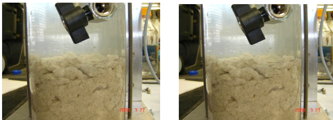
Figure 76. Coated Sand with Xanthan and Guar Gum did not Erode at 3.7 m/s (A) or 11m/s (B).
