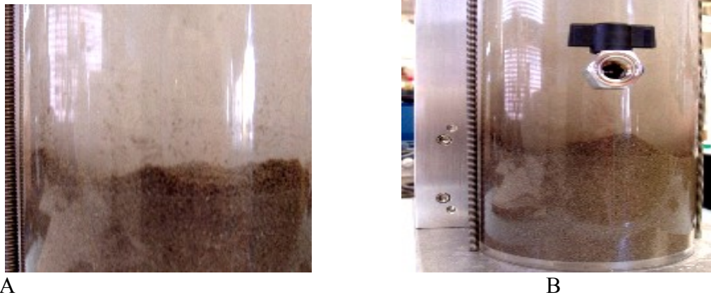
Figure 78. Resuspension of Organoclay (PM-199) leading to Cloudiness (A) and Surface Suspension (B).
