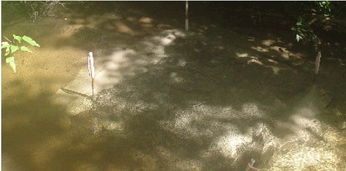
Picture 17. Plot 3 -- One-layer Cap Composed of Apatite (50%) and Sand (50%) with a Sand Transition Zone. Two sets of pore water sampler tubes were located near the top of the cap (white tubes for samplers beneath the cap and black tubes for samplers in the middle of the cap).
