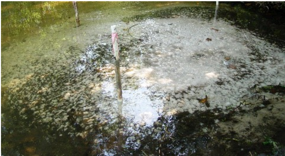
Picture 18. Plot 4 Cap Composed of Two Layers including a Two Inch Layer of Biopolymer/Sand Slurry over a Four Inch Layer of 50% Apatite and 50% Sand.
