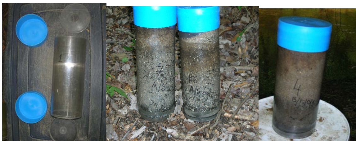
Picture 10. Coring Tubes and Sediment Cores used for Evaluation of Erosion Resistance by an ASSET Flume.
