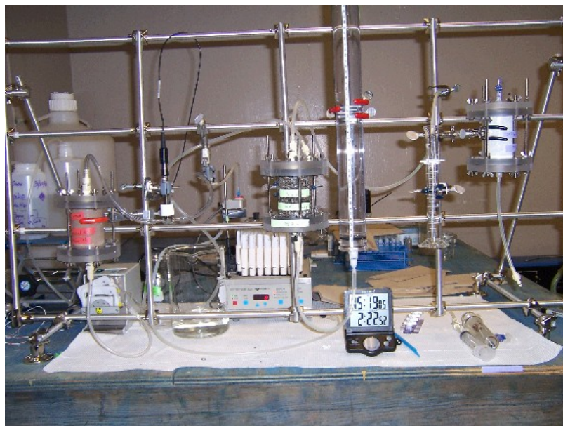
Picture 1. Setting of the Experiment on Advective Transport of Metals through Cap Materials.
