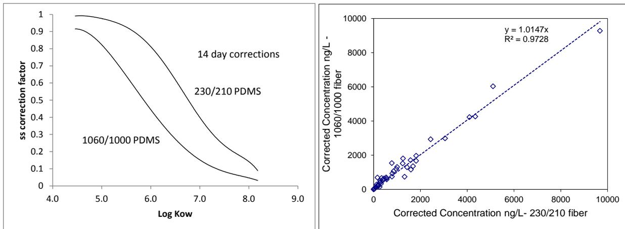
**Figure 9. Hunters Point 14-day corrections for steady state PDMS uptake and comparison of correction porewater concentrations (ng/L).**
