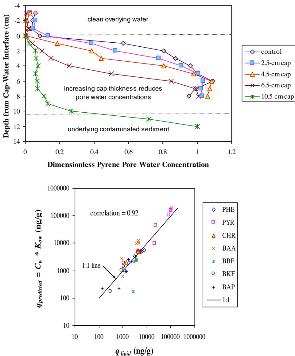
**Figure 5. Observed pyrene concentration profiles as a function of cap thickness, illustrating rapid mixing of contaminants in a thin layer cap when depth of organism interaction is greater than cap thickness.**
