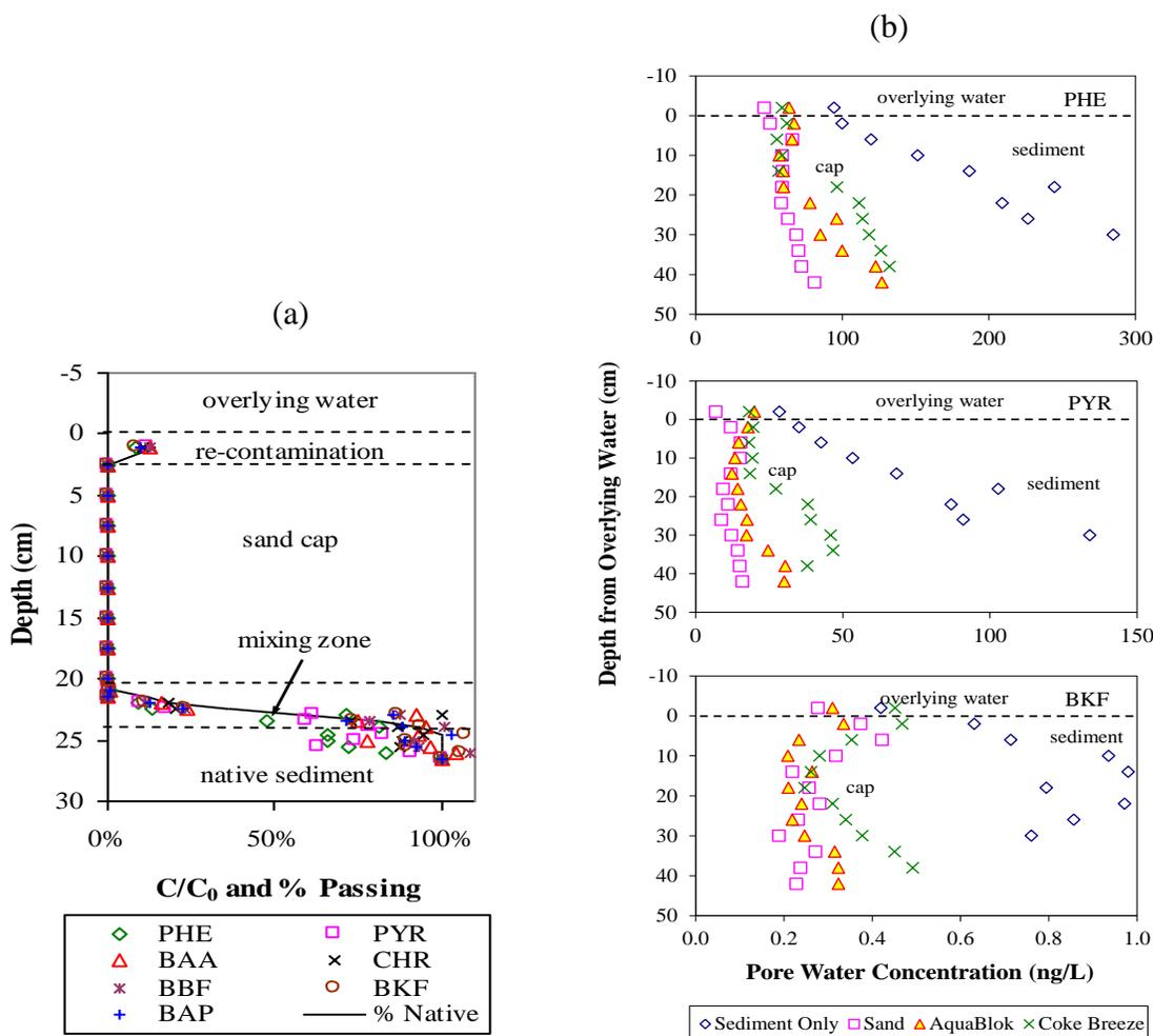
**Figure 6. (a) Bulk solid concentrations of selected PAHs in the sand cap, (b) Porewater concentration of three PAHs in the sediment and in a sand, sand and AquaBlok, and sand and coke breeze layer caps.**
