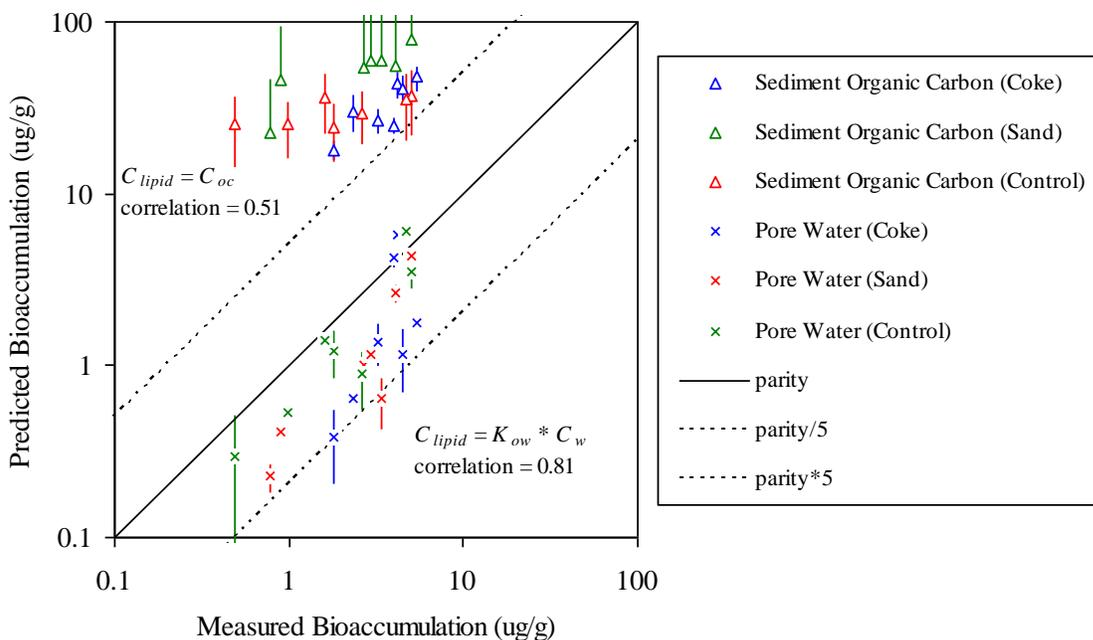
**Figure 8. Correlation of predicted and observed lipid normalized bioaccumulation assuming BSAF=1 (using solid concentration as predictor) or BAF= $K_{ow}$  (using porewater concentration as predictor) for all measured PAH compounds (phenanthrene, pyrene, chrysene, benzo(a)anthracene, benzo(b)fluoranthene, benzo(k)fluoranthene, and benzo(a)pyrene).**
