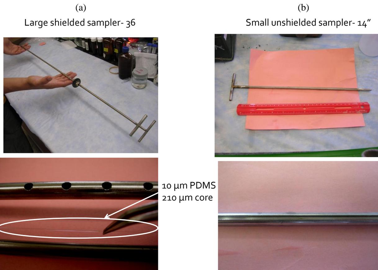
**Figure 1. Shielded and unshielded holders for SPME fiber.**
