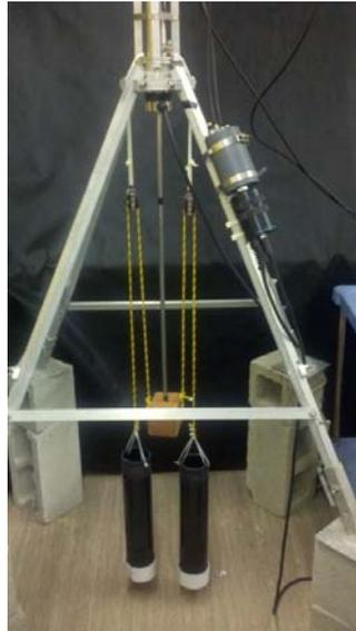
Figure 8. Pressure measurement calibration setup.
