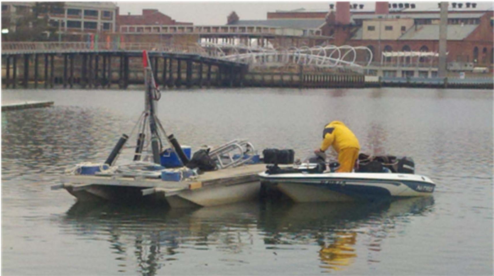
Figure 26. Pontoon platform with SED-FSP system assembly and locally rented support boat.
