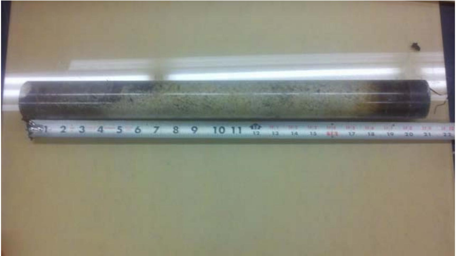
Figure 28. Sediment core sample collected during sand cap survey.
