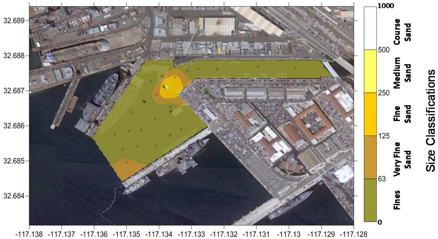
Figure 19. SED-FSP survey results for mouth of Chollas Creek at NBSD.
