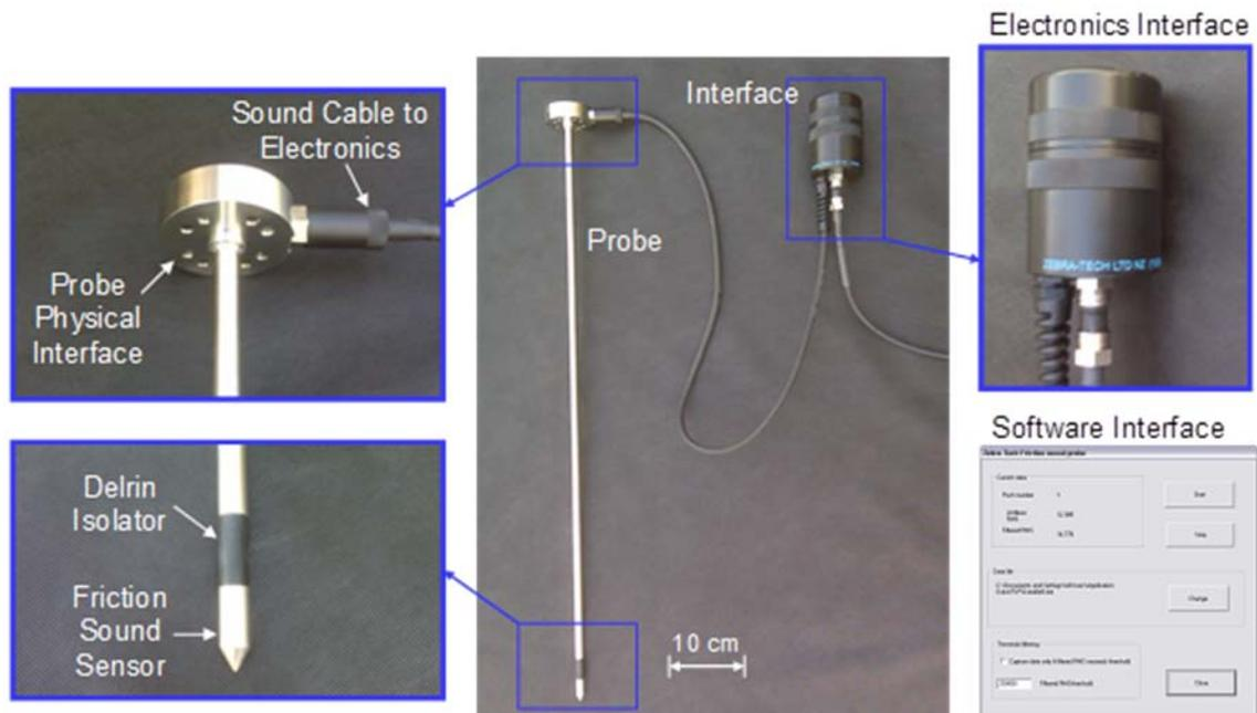
Figure 2. Commercial prototype sediment friction-sound probe (SED-FSP).
