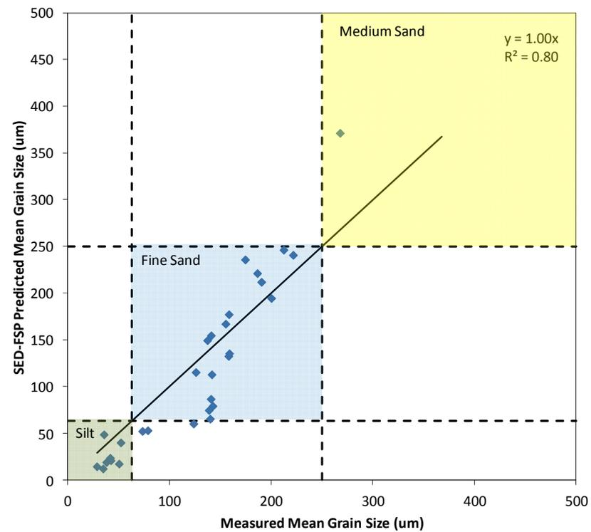
Figure 20. SED-FSP results for IR Site 9 validation survey showing linear (left) and power-law fit (right) including data (left) that is excluded from calculations. The dashed line in the left-side plot indicates the data trend and is not a fit of the data.
