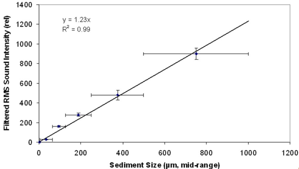
Figure 4. SED-FSP acoustic responses to laboratory prepared samples.
