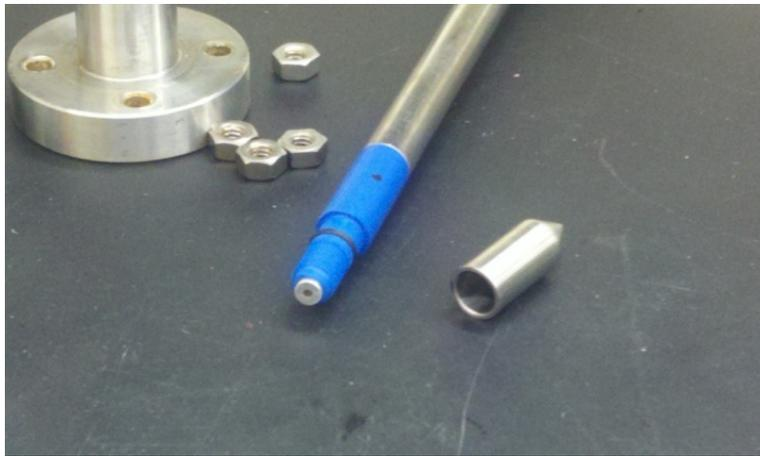
Figure 1. Probe-tip microphone in Delrin isolator.
