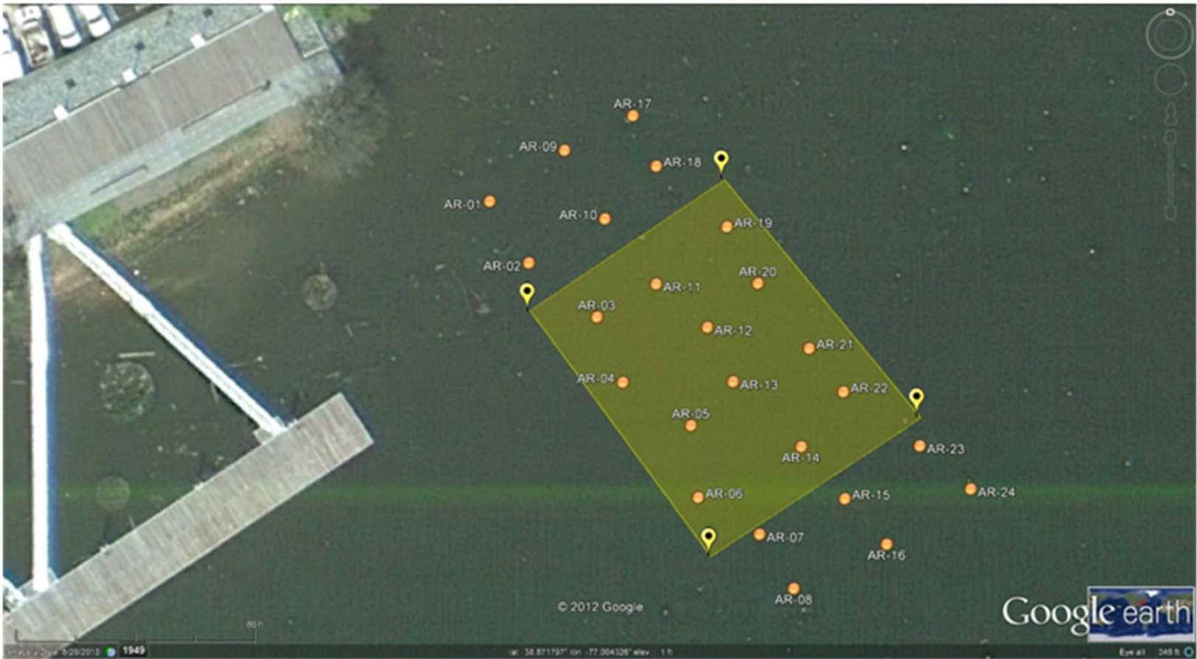
Figure 25. Anacostia River thin-layer sand cap site identifying the cap placement (yellow/green polygon) and SED-FSP deployment locations (orange symbols).
