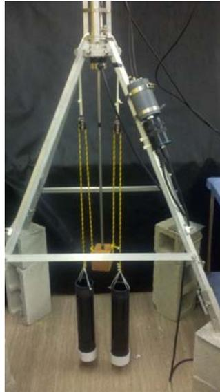
Figure 8. Pressure measurement calibration setup.
