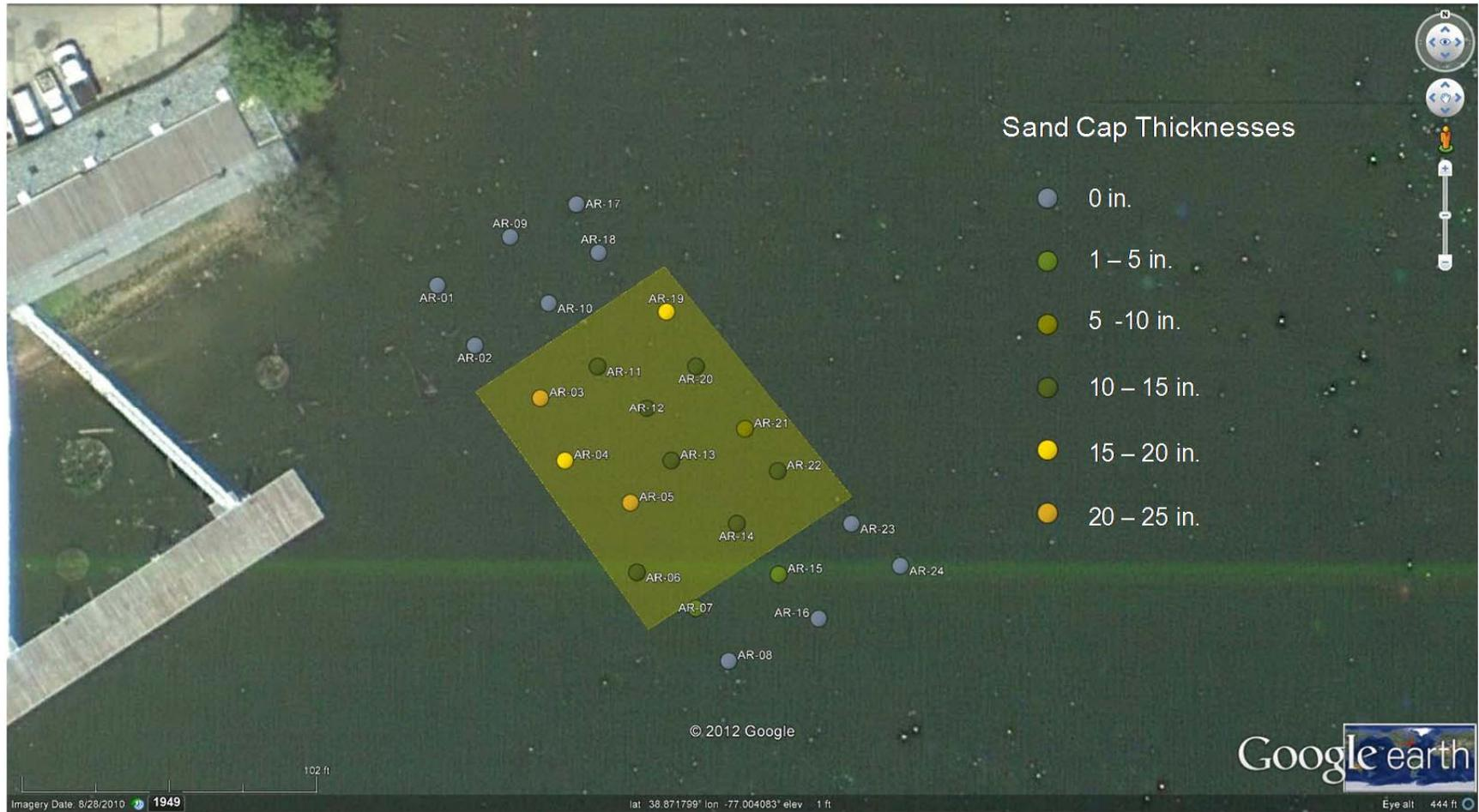
Figure 27. SED-FSP grain size survey results for Anacostia River sand cap field deployment. Rectangular area is cap location according to the placement contractor. Symbols represent depth horizons of cap material as measured by the SED-FSP system; the legend on the right side of the figure indicates the depth of cap material.
