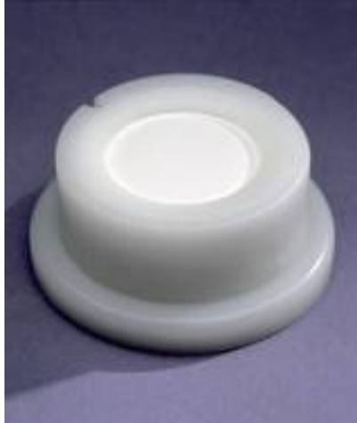
Figure 2-21. Commercially available Diffusive Gradients in Thin-film (DGT).
