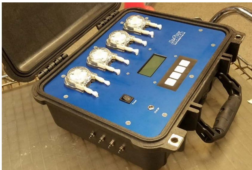
Figure 6: Side view with inlet/outlet ports corresponding to pumps.
