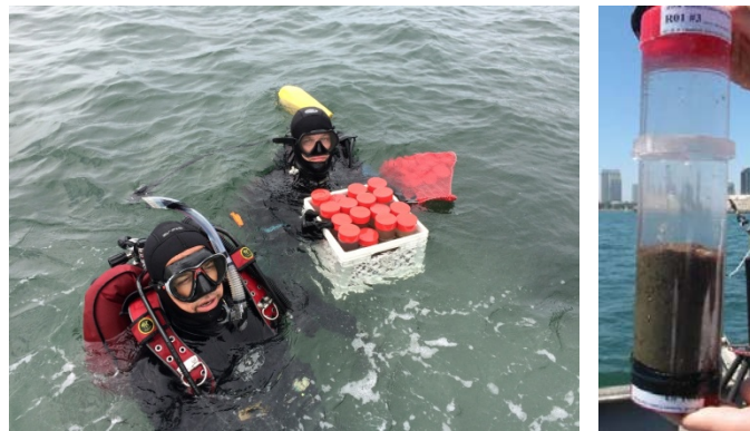
Figure 2-4. Divers returning to surface with hand-collected cores (left); example of diver collected intact sediment core (right).
