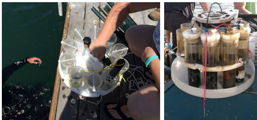
Figure 2-14. Version 1.0 (left) and Version 3.0 (right) SEA Rings that were deployed at Paleta Creek for in situ bioaccumulation studies.
