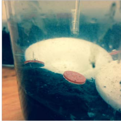
Figure 2-20. SPME and DGT deployment in Ex Situ bioavailability study.
