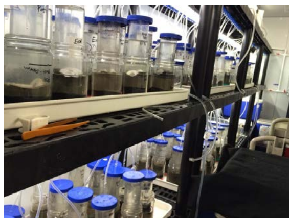
Figure 2-18. Experimental set up for ex situ exposures of intact sediment cores.
