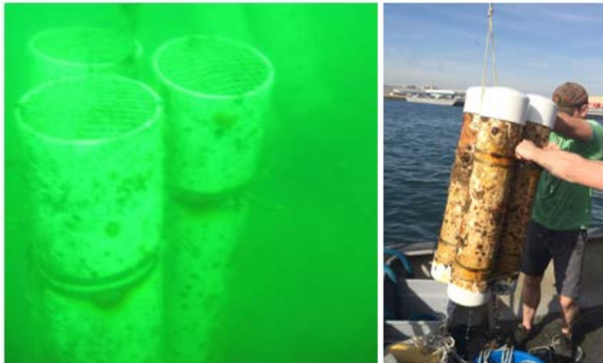
Figure 2-9. Bundled sediment traps were deployed at Paleta Creek to ensure sufficient material would be collected during the exposure period (left); recovery of the capped and bundled sediment traps by davit assistance (right).
