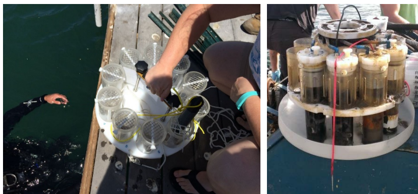
Figure 3-11. Version 1.0 (left) and Version 3.0 (right) SEA Rings that were deployed at Paleta Creek for in situ bioaccumulation studies.
