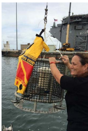
Figure 2-11. Deployment of ADCP and OBS sensor mounted within a protective cage at Paleta Creek, NBSD.
