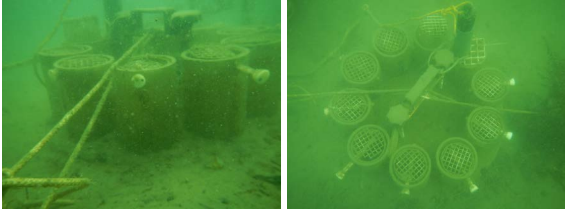
Figure 2-17. Observations made of the SEA Rings upon recovery show evidence of deposition on the device.
