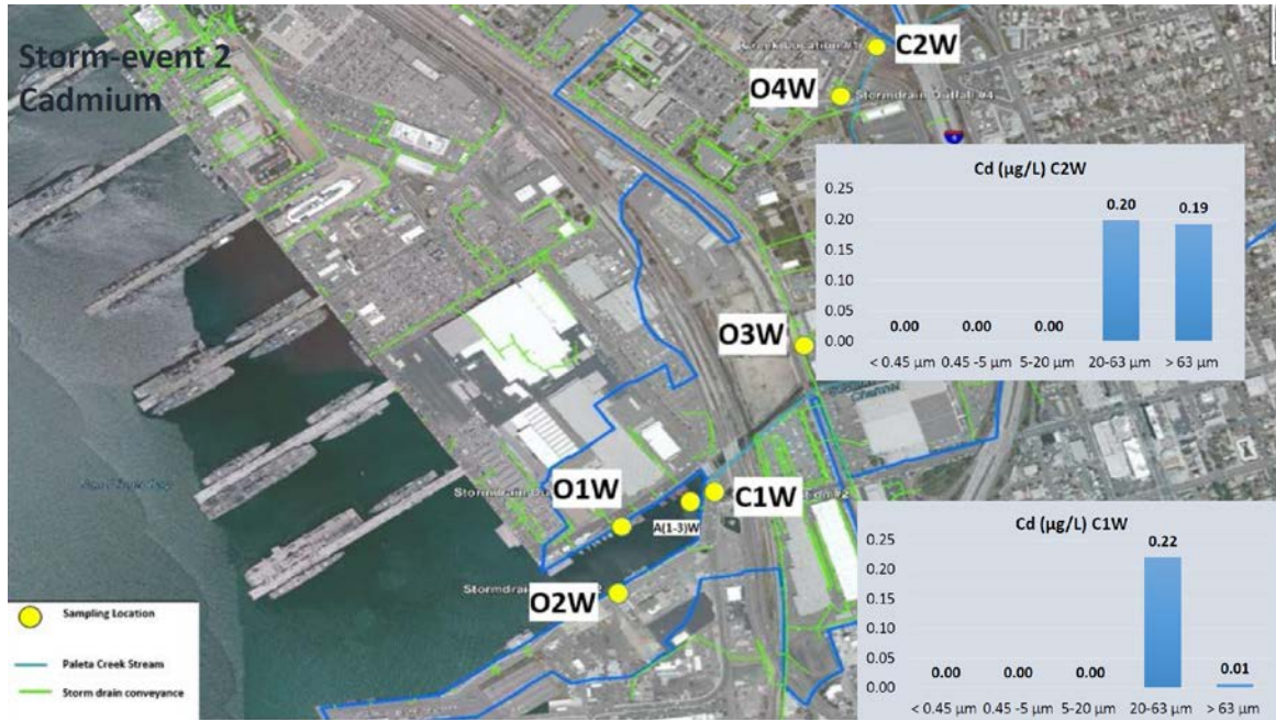
Figure 4-5 Cd loads in outfall and Paleta Creek locations – Storm event 2. Cd loads from outfalls O1W and O2W were not significant.
