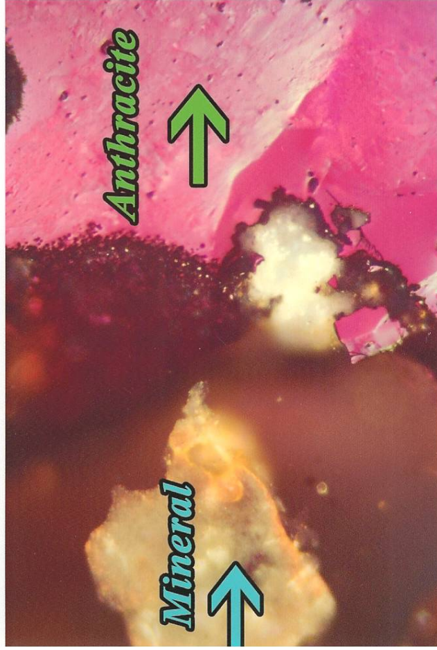
Figure A15 Photomicrographs of Materials in the UMBC Soil Sample AR-16 Showing: High and Medium Volatile Bituminous Coal, Anthracite Coal, Metallurgical Coke, Green Plant Material, Mineral Matter Coating and Other Mineral Matter. Reflected Light in Oil, 400X.
