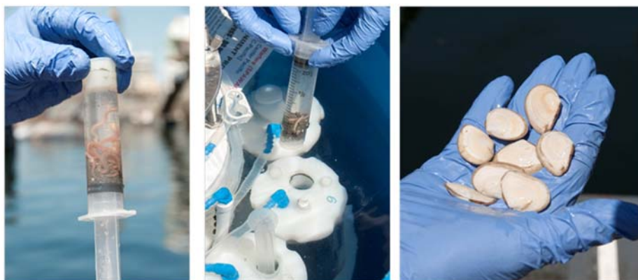
Figure 2.2. Smaller Organisms (e.g. Polychaetes and Amphipods) Are Delivered by Preloaded Syringes while Larger Organisms (e.g. Clams) Are Placed into Chambers Prior to Deployment.
