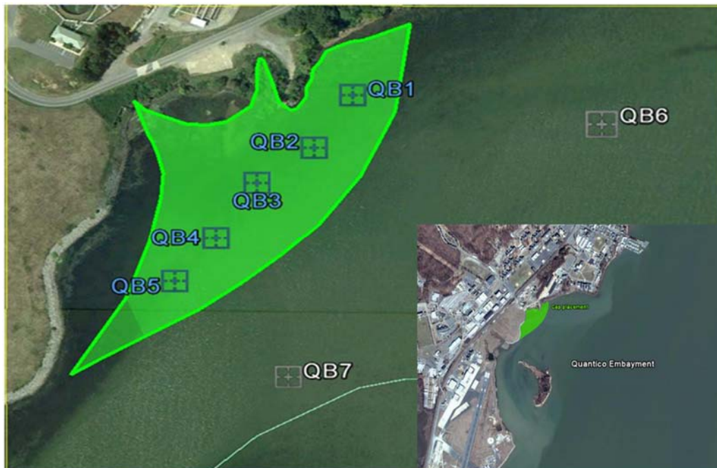
Figure 4.2. Sampling locations for MCB Quantico site. The area in green represents where a thin-layer sand cap was installed in April 2014.
