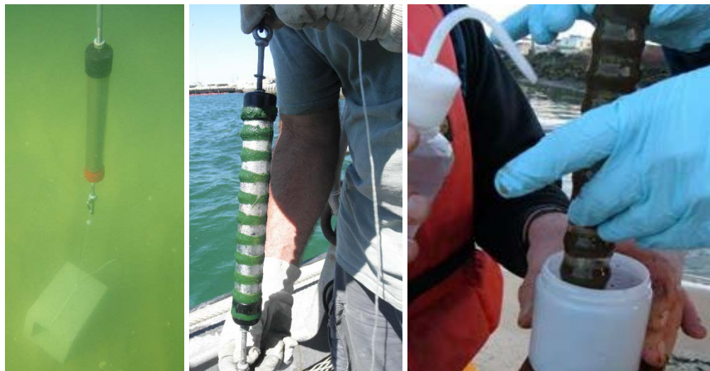
Figure 9. (Left) Magnets Deployed 1 Meter Above Sediment Surface with Pellet Buoy (just out of picture); (Center) Magnet Recovered with Green Tracer; (Right) Removal of Outer Sheath by Sliding off Magnet and then Washing Tracer into Sampling Jar.
