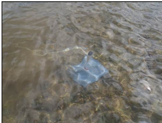
Figure 12. The Magnet and Sheath Assemblies Attached to Baseplates and Placed on the Seabed.
