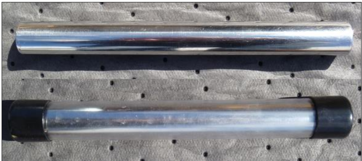
Figure 6. One of the powerful, permanent REE magnets used in this study (top) and housed in the sheath with endcaps (bottom).
