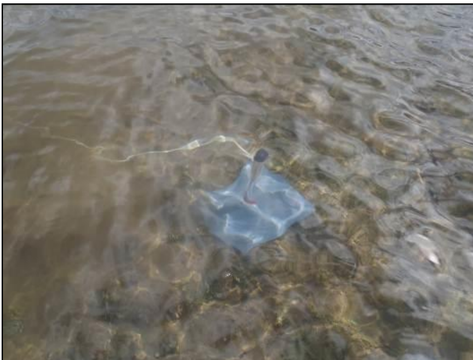
Figure 31. The magnet and sheath assemblies attached to baseplates and placed on the seabed.
