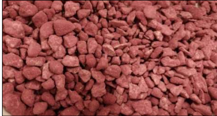
Figure 16. The pink tracer particles incorporated to AquaGate™ to create a tracer-AquaGate™ particle . Source: AquaBlok Ltd.
