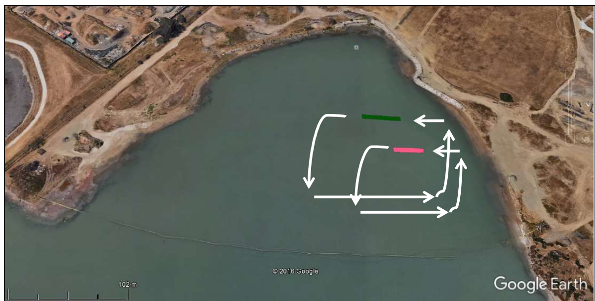
Figure 18. The approximate vessel tracks during deployment of the pink and green tracer. Note; the vessel tracks during the green tracer deployment do not cross the pink deployment zone so as to ensure no resuspension occurred due to propeller wash. Note; this diagram is not to scale. Source: Google Earth.
