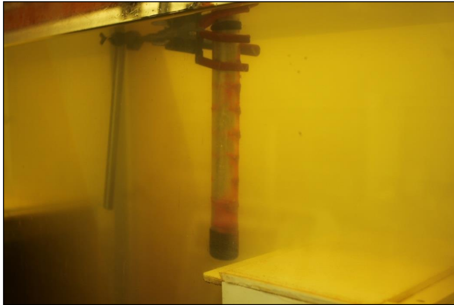
Figure 36. The magnet secured in position within the flume, with tracer retained. At the time of the photo the flow velocity in the flume was \sim 0.1 \text{ m s}^{-1} .
