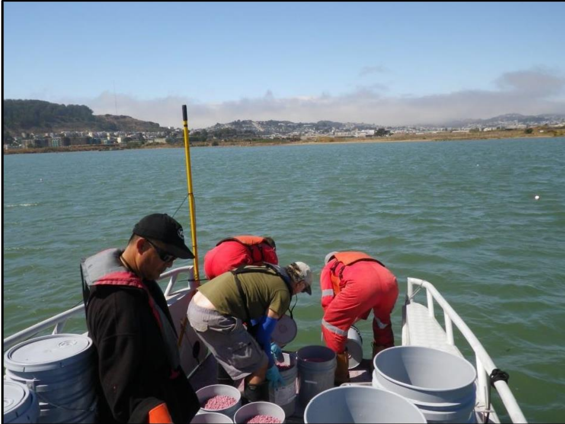
Figure 28. Manual release of pink tracer in AquaGate formulation from the bow of the landing craft style vessel (looking west with BZ02 buoy at right of vessel). Note yellow pole which held an in situ fluorimeter sensor 0.5 meters below the surface to check for tracer release in the water column.
