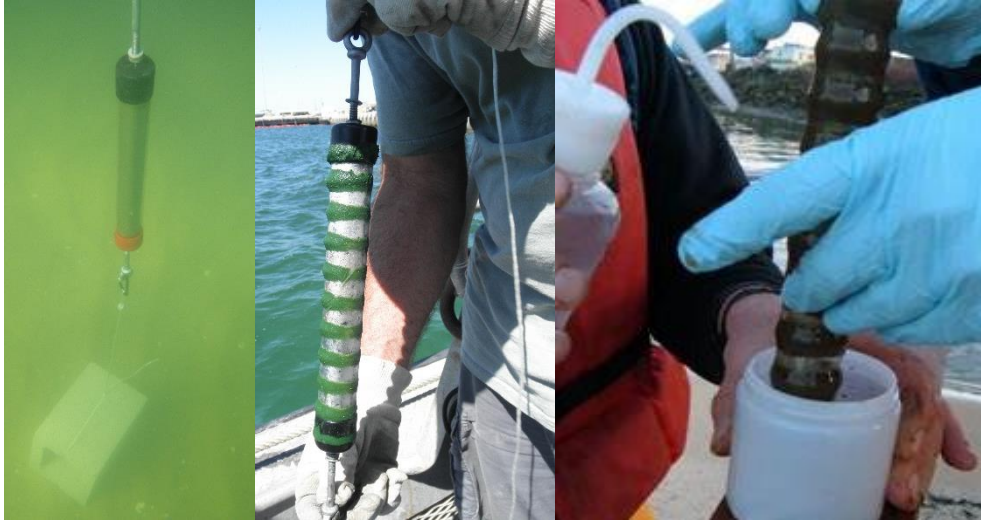
Figure 21. (Left) Magnets deployed 1 meter above sediment surface with pellet buoy (just out of picture); (Center) Magnet recovered with green tracer; (Right) Removal of outer sheath by sliding off magnet and then washing tracer into sampling jar.
