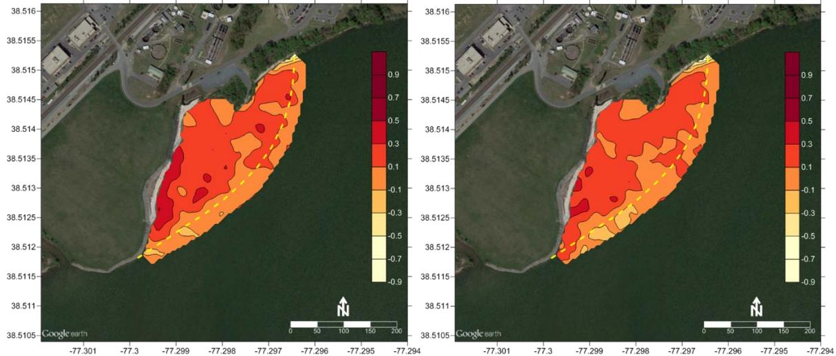
**Figure 6. Difference Map for the 2014 Pre-cap Baseline Compared to the 2015 Post-Cap Survey (left) and Difference Map for the 2014 Pre-cap Baseline Compared to the 2016 Post-cap Survey (right). The yellow dashed line indicates the offshore boundary of the area targeted for the thin-layer cap. Positive differences indicate 2015 elevations that are higher than 2014 elevations. Units are meters.**
