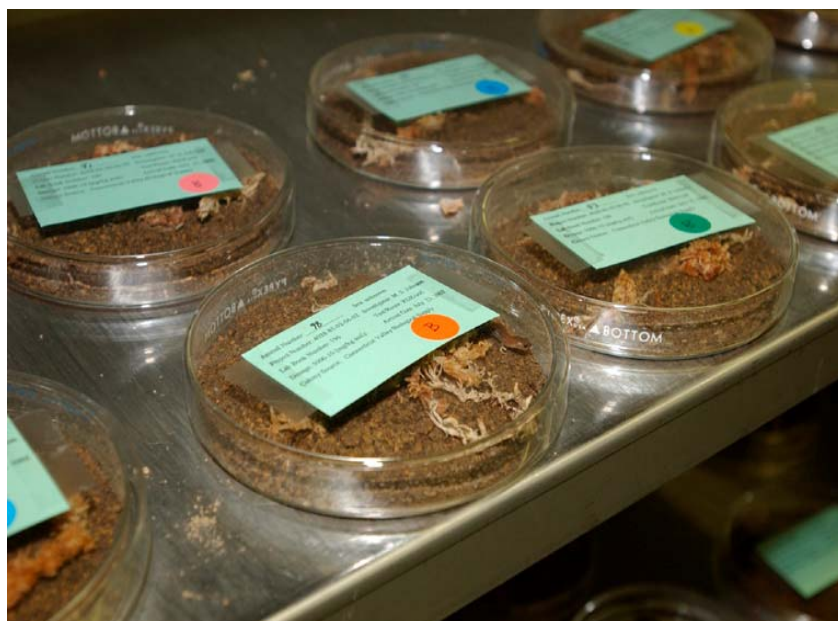
Figure 4-1 Soil Exposure Protocol Test Set-up
