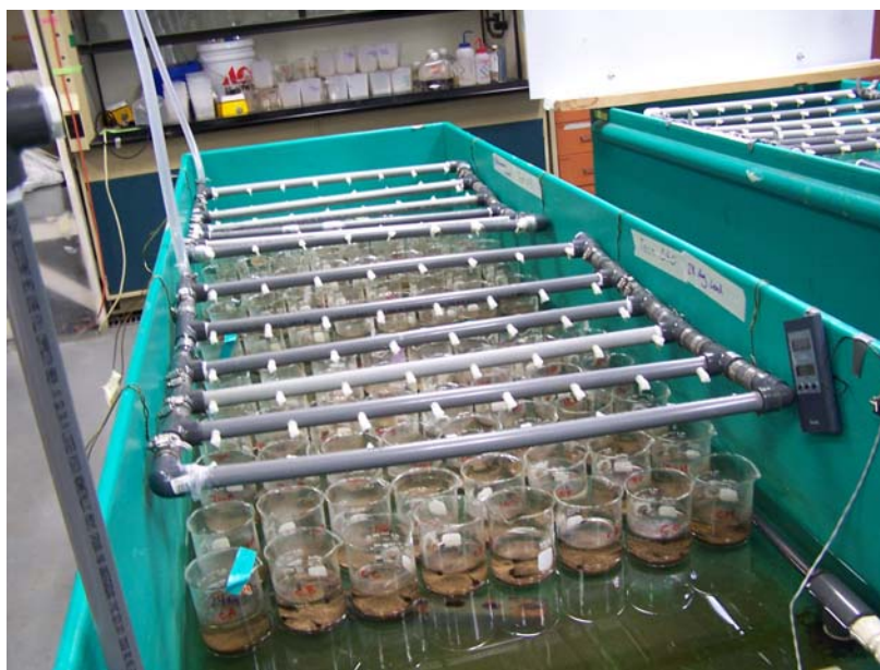
Figure 4-4 Sediment Exposure Protocol Test Set-up
