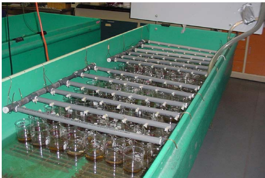
Flow-through test system in a temperature-controlled water bath.
