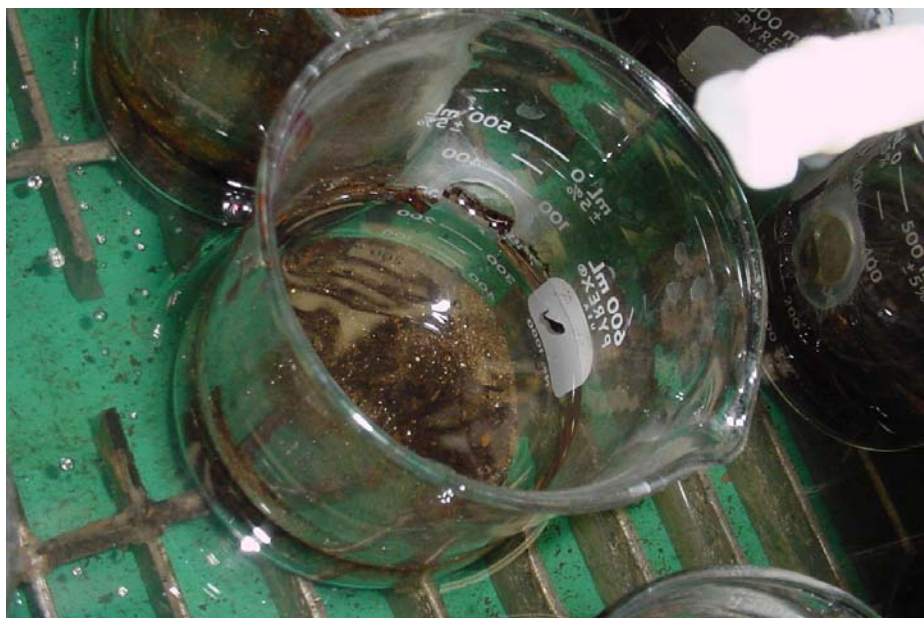
Test beaker in water bath. Test organism can be seen against the white beaker label.
