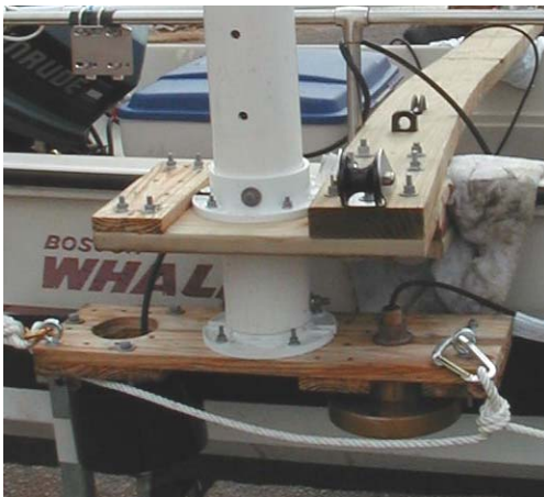
Figure 23 Over the side mounting for dual frequency depth sounder.
