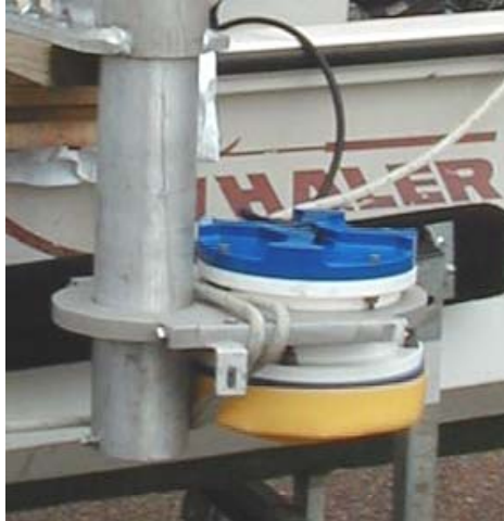
Figure 36 Over the side mounting for ADCP.
