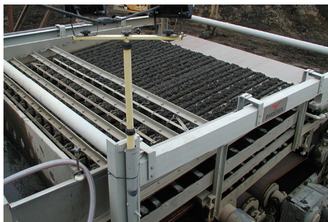
Figure 6. Belt filter press rakes in gravity drainage zone
