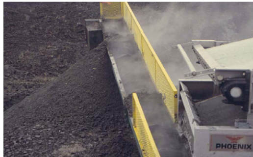
Figure 3. Dewatered solids at 45-50 percent solids content
