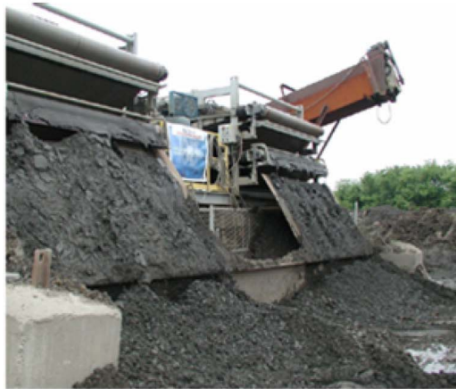
Figure 1. Dewatered cake from belt filter presses
