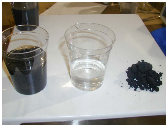
Figure 9. Flocculated slurry, supernatant and cake (Photo provided courtesy Centrisys)
