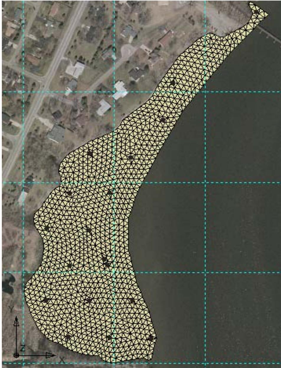
**Figure 2.1** Preliminary Surface TIN for Sub-area C. Positions of sampling stations (•) and grid lines spaced at 500 ft. (---) are also shown.
