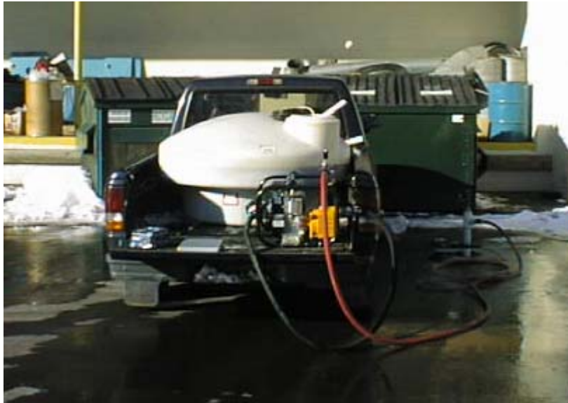
Figure 4-4. Vehicle Mounted Molasses Injection Rig
