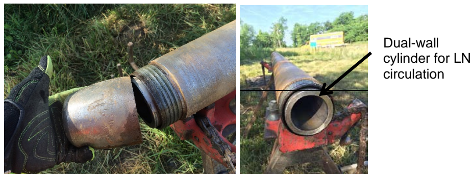
Figure 17. Photos of Core Barrel Sampler.
