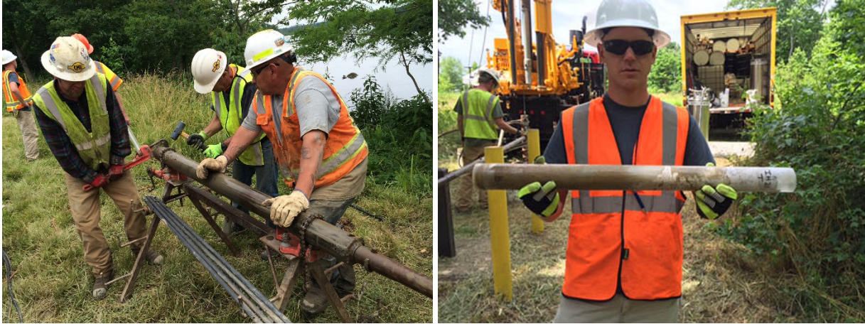
Figure 21. Photos of Frozen Core Removal from the Continuous Sampler.
