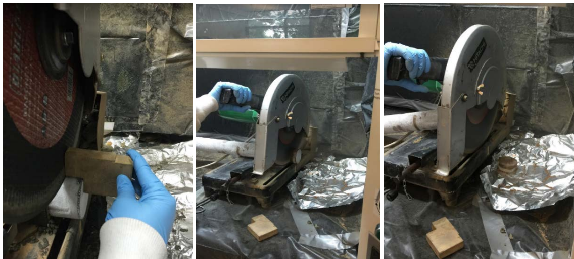
Figure 23. Photos of Cutting of Frozen Core into “Hockey Pucks.”
