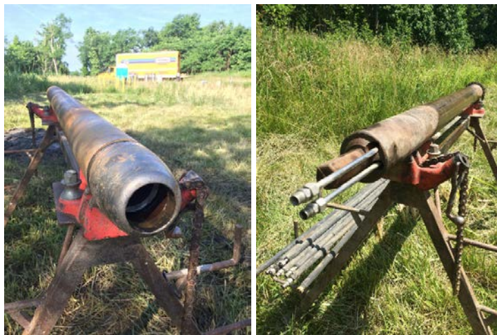
Figure 16. Core-barrel Sampler Photos.
