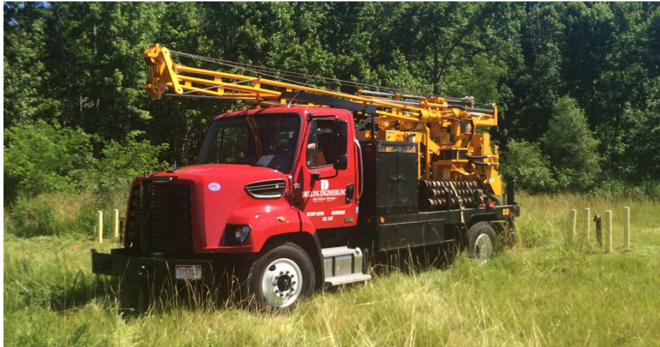
Figure 3. Hollow-stem Auger Drill Rig Used for C 3 .
