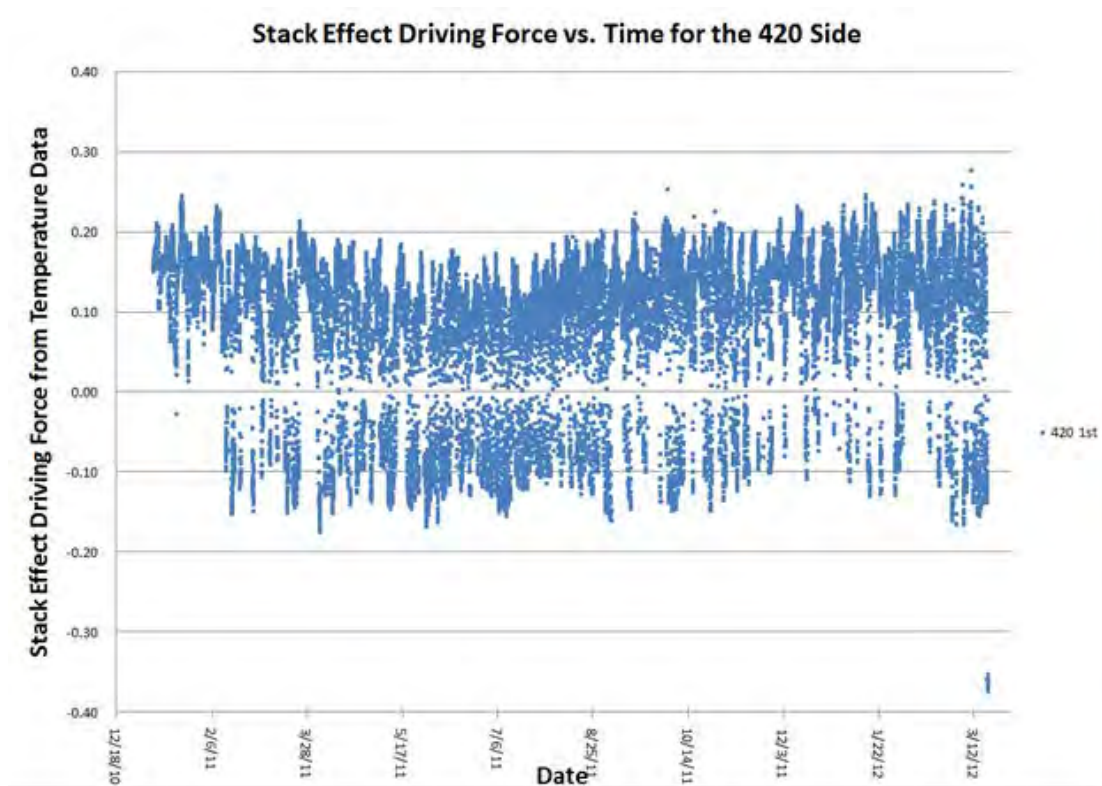
Figure 10-8. Stack effect driving force 420 (unheated) side over time.
