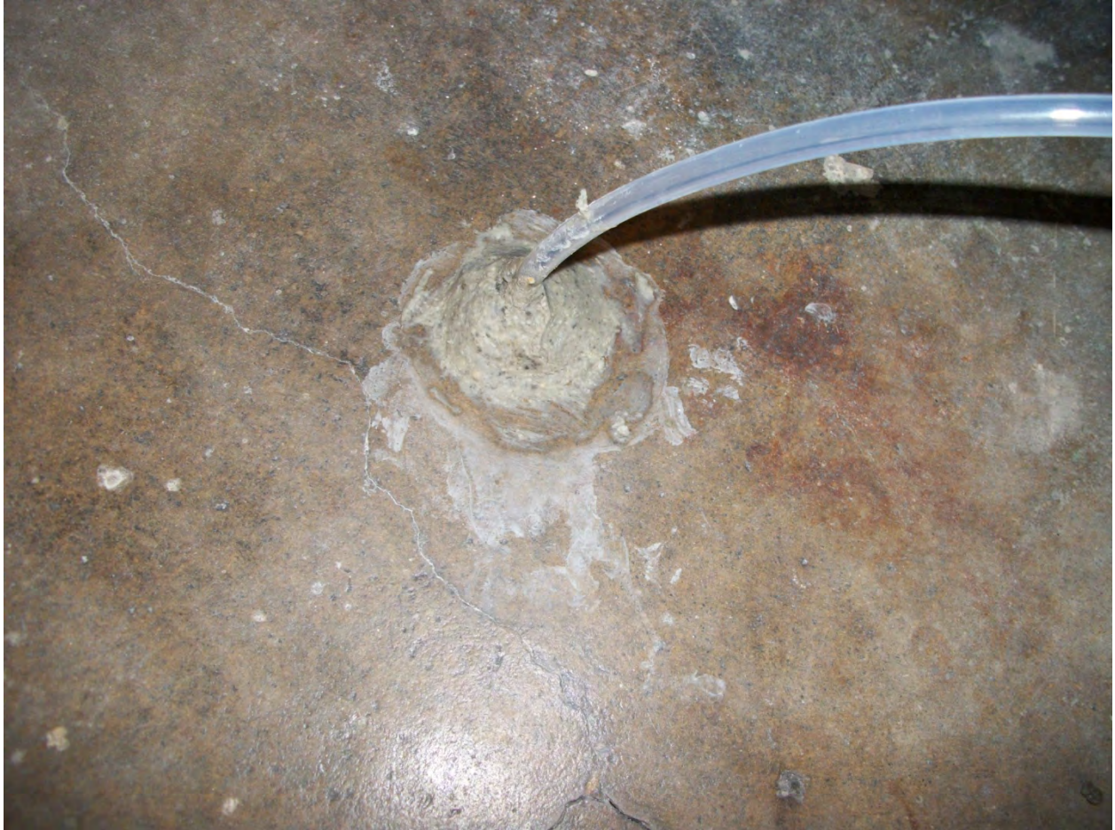
Typical Temporary Port Construction Before Sampling
