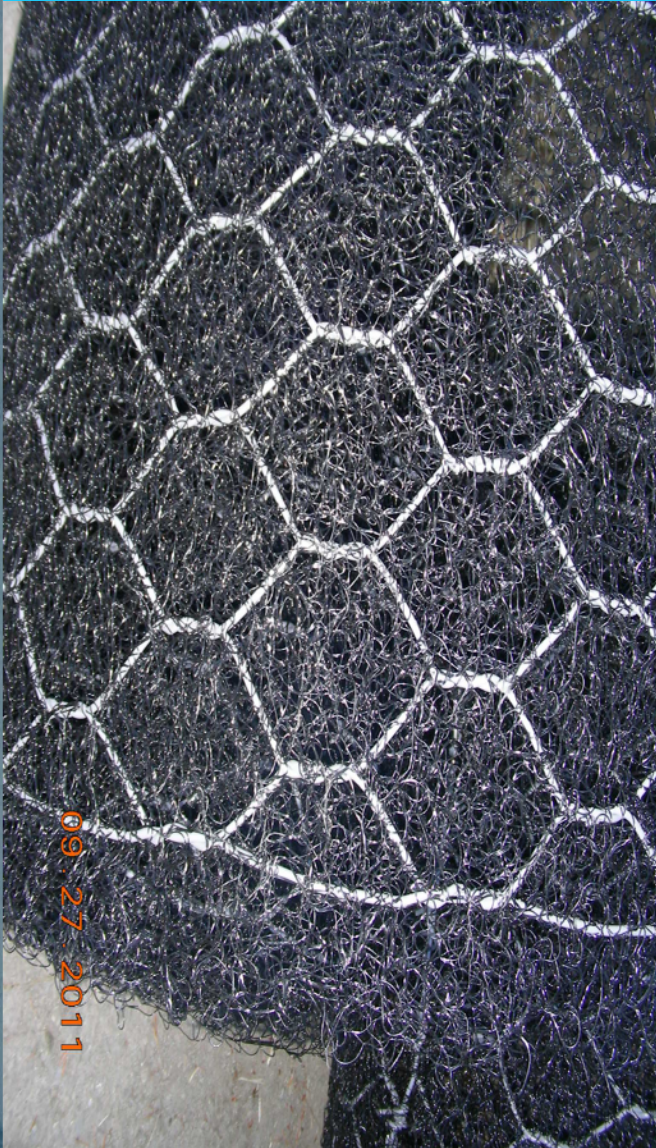
Double-Twisted PVC-Coated Steel Mesh With Lofted Polypropylene Netting
