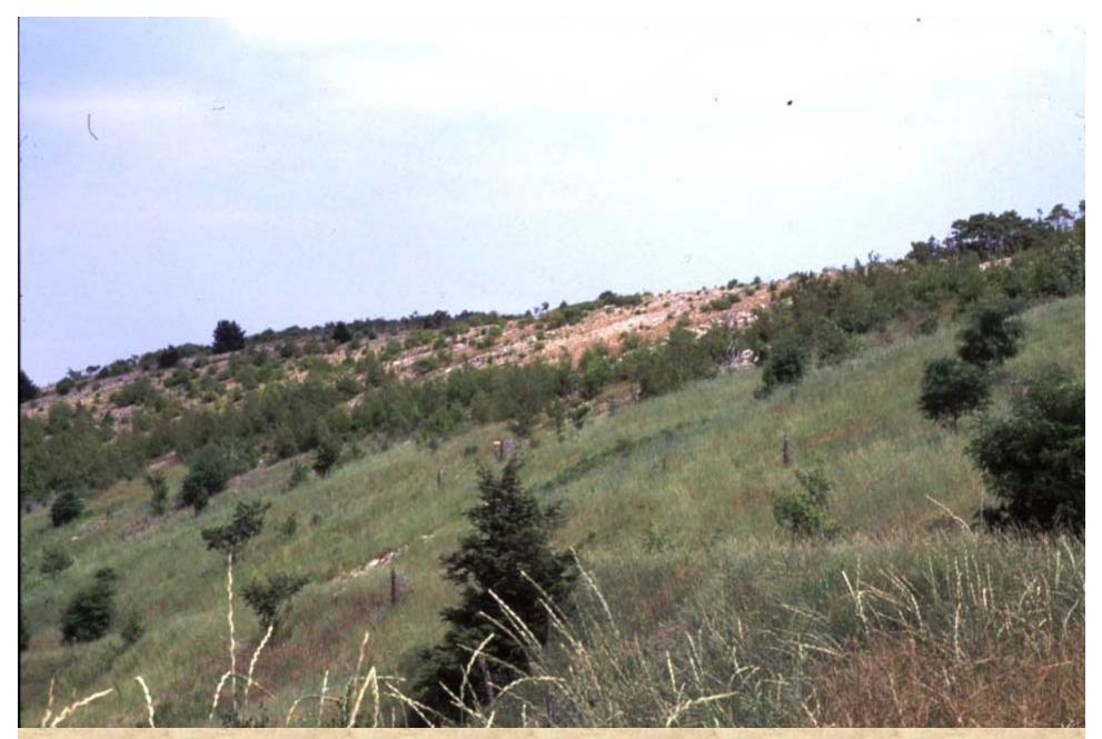
Palmerton, PA: Blue Mountain – 1999; Foreground = Biosolids+Limestone+FlyAsh; Background = untreated Control Mean total Zn, Cd and Pb, and DTPA-extractable Zn and Cd (at 100 mL extractant/2 g soil) in Palmerton "Revival Field" Test Plots Comparing Traditional and Biosolids Compost Remediation Treatments (Li et al., 2000).
