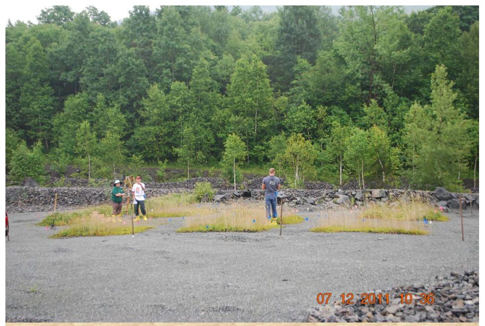
Vermont Asbestos Group Field plots in July, 2011 showing effective remediation using compost plus gypsum & NPK.
