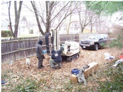
Soil gas sampling on the NWIRP eastern border in January 2008. Sampling indicated elevated levels of volatile chemicals at the facility boundary.
