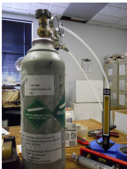
Figure 6. SF 6 Tracer Gas Delivery System as Deployed at Moffett Field Building 107.
