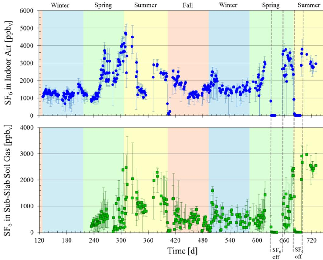
Figure 4.30. Daily 24-h average SF<sub>6</sub> concentrations in indoor air and sub-slab soil gas at location 3 from with error bars spanning the daily maximum and minimum values.
