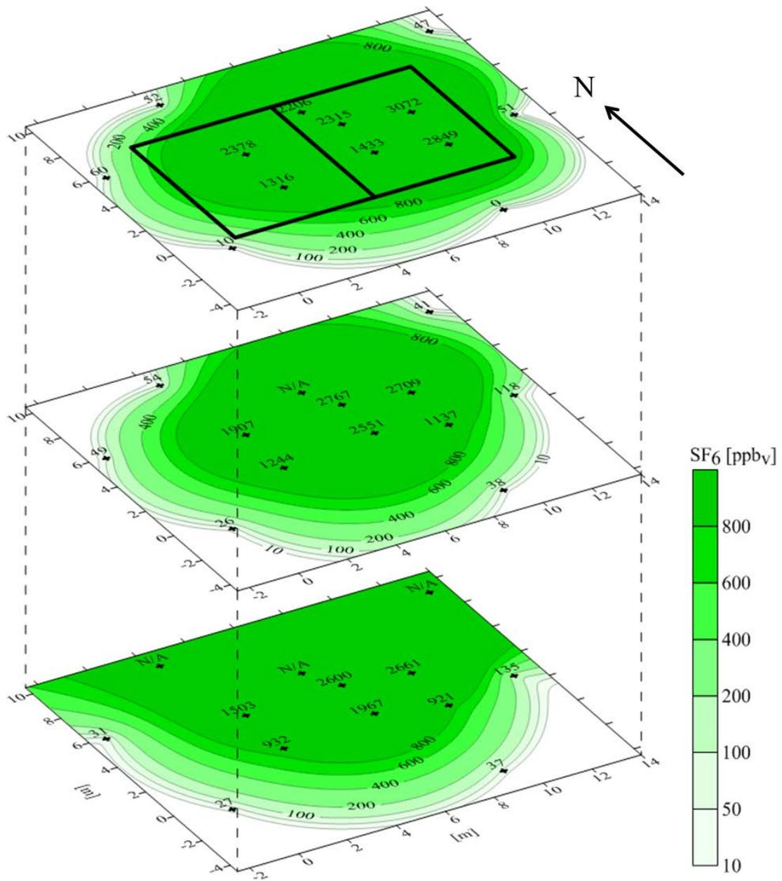
Figure A.38. Contour plots of SF<sub>6</sub> concentrations in soil gas at depths of SS, 0.9 BS, and 1.8 m BS from synoptic soil gas survey in August 2012.
