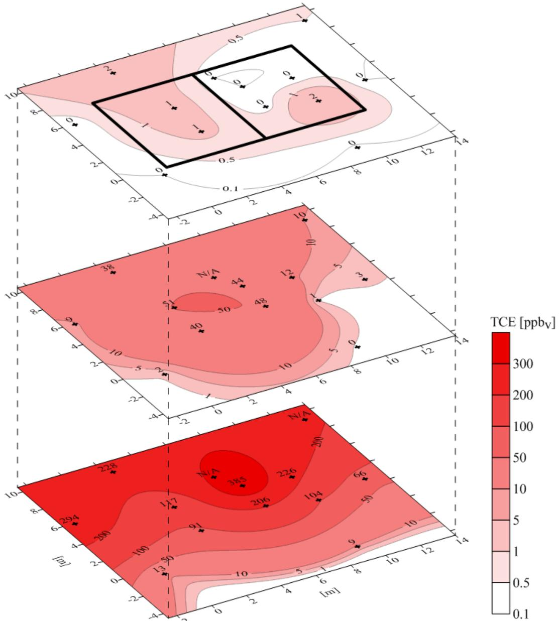
Figure A.3. Multi-depth contour plot of TCE in soil gas for samples collected and analyzed from August 7<sup>th</sup> to August 10<sup>th</sup>, 2010.
