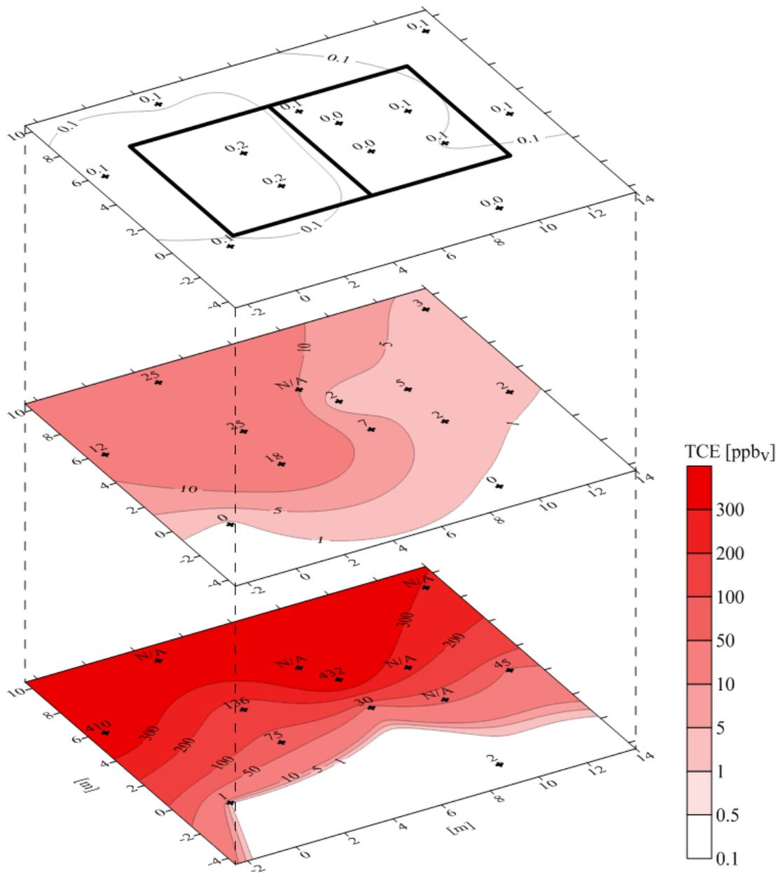
Figure A.8. Multi-depth contour plot of TCE in soil gas for samples collected and analyzed from May 18<sup>th</sup> to May 20<sup>th</sup>, 2011.
