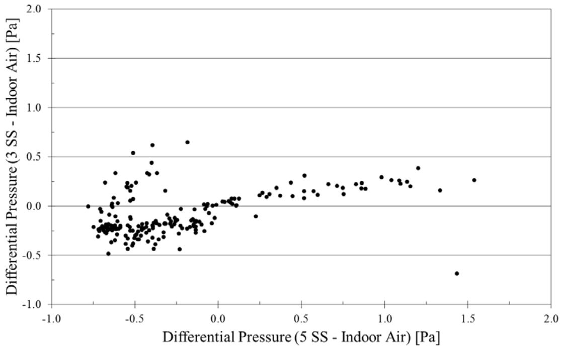
Figure A. 57. Comparison of time-matched 24-h average sub-slab to indoor air differential pressure values from location 3 and location 5.
