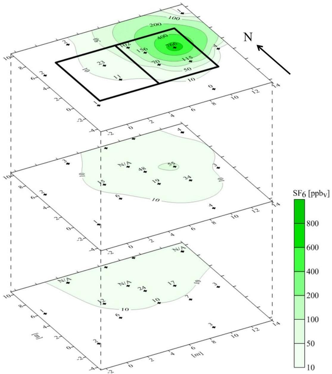
Figure A.28. Contour plots of SF<sub>6</sub> concentrations in soil gas at depths of SS, 0.9 BS, and 1.8 m BS from synoptic soil gas survey in March 2011.
