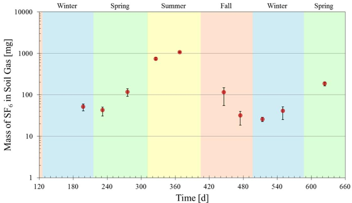
Figure 4.31. Average estimate mass of SF<sub>6</sub> in soil gas below the study house from synoptic soil gas survey data with error bars spanning the range of estimated values for each event.
