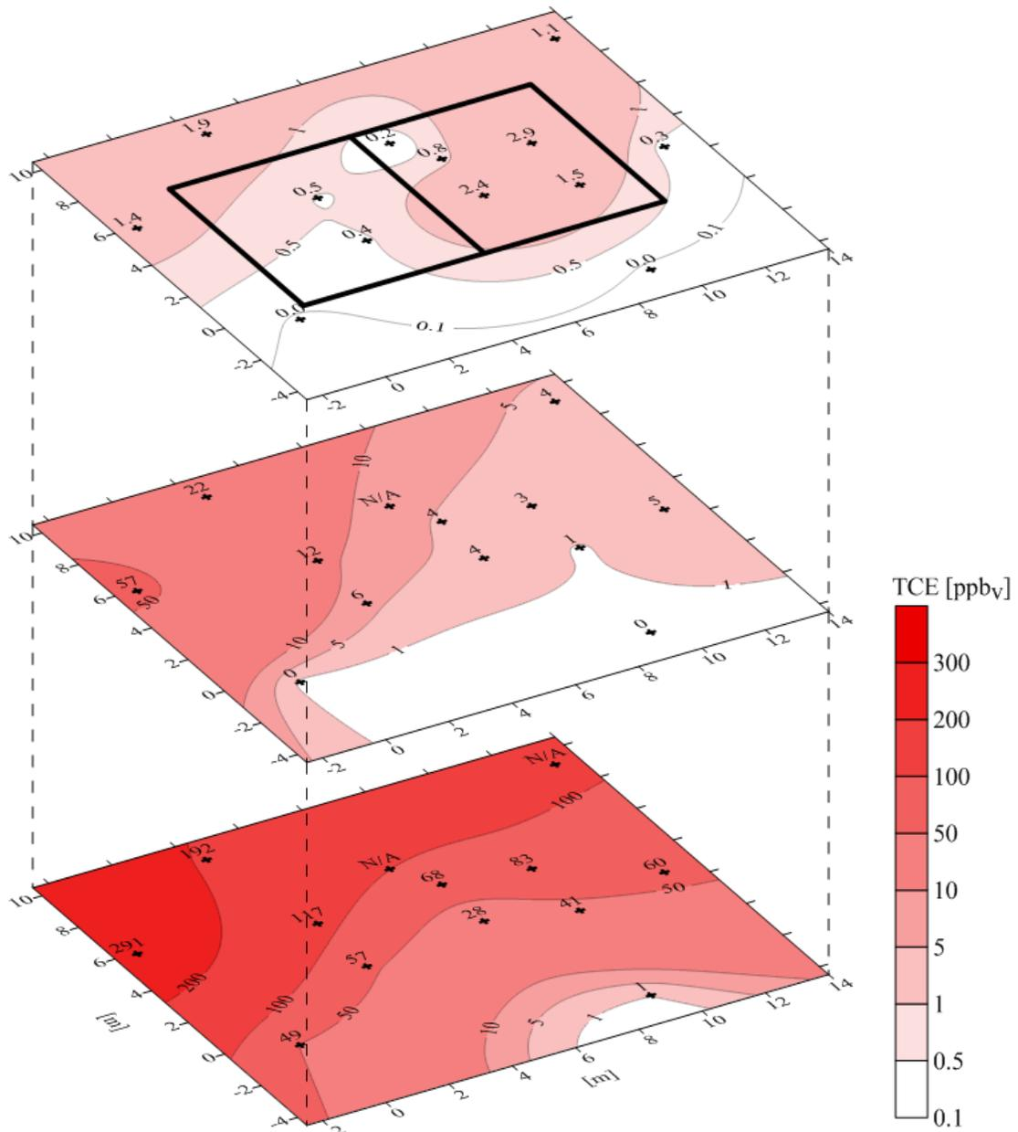
Figure A.13. Multi-depth contour plot of TCE in soil gas for samples collected and analyzed from December 3<sup>rd</sup> to December 4<sup>th</sup>, 2011.
