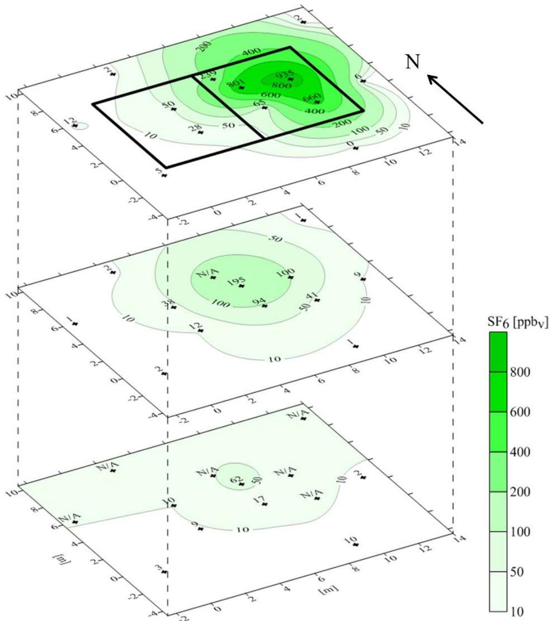
Figure A.30. Contour plots of SF<sub>6</sub> concentrations in soil gas at depths of SS, 0.9 BS, and 1.8 m BS from synoptic soil gas survey in May 2011.
