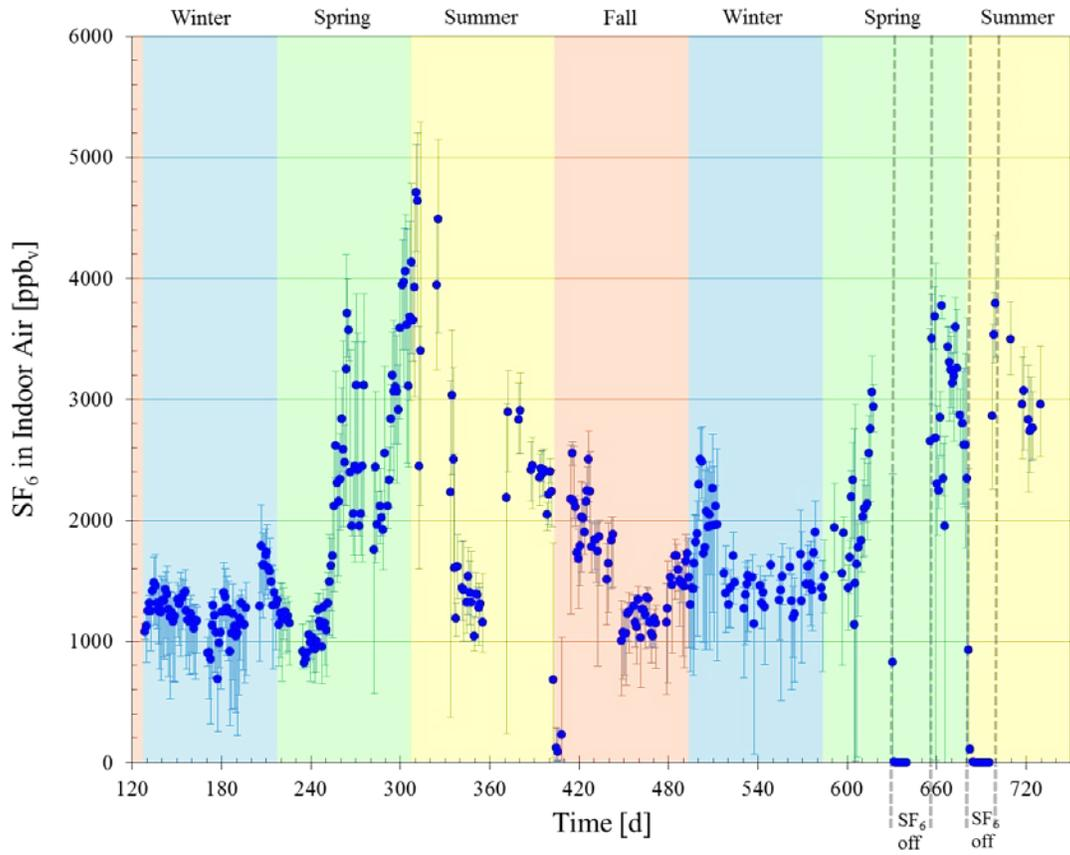
Figure A.22. 24-h averaged SF<sub>6</sub> concentrations in indoor air from winter 2010 through summer 2012 with error bars spanning the daily maximum and minimum values.
