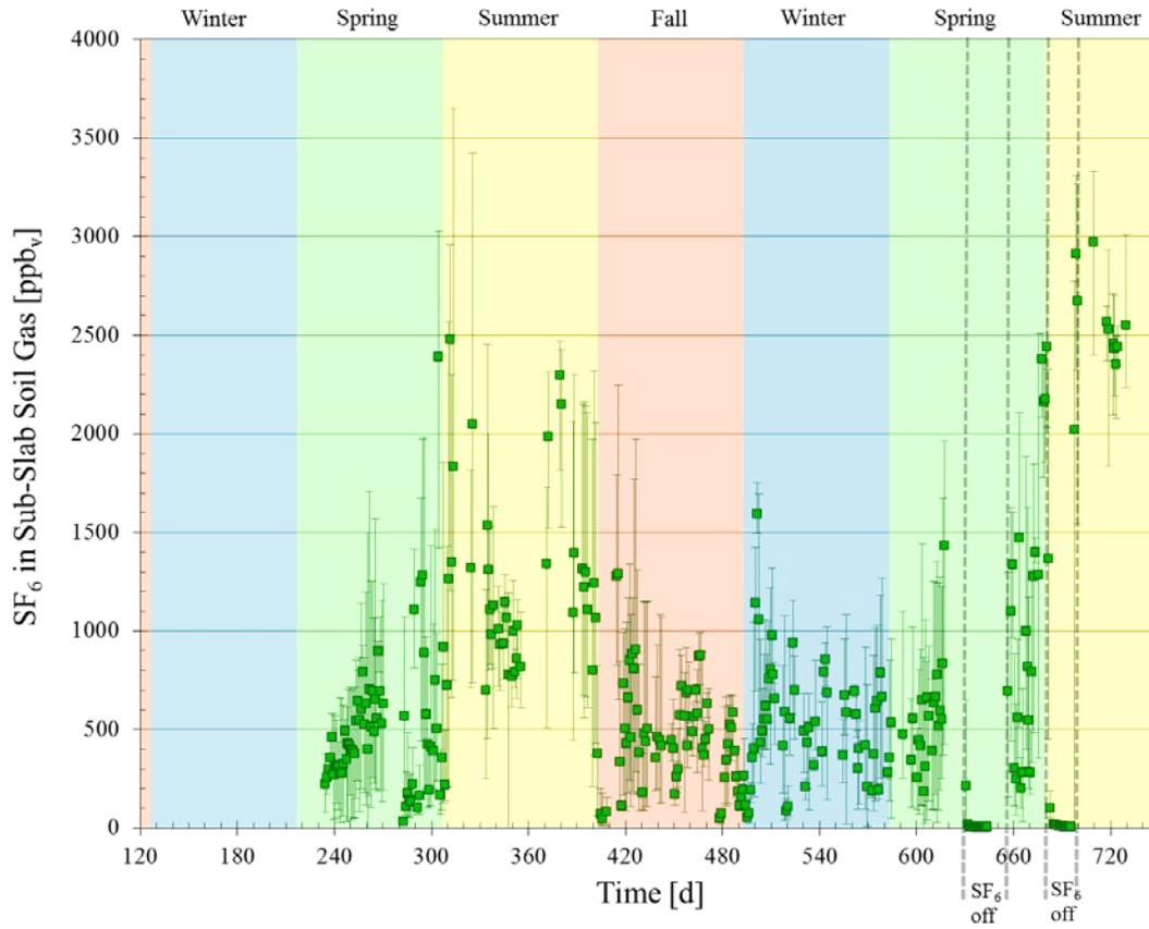
Figure A.24. 24-h averaged SF<sub>6</sub> concentrations sub-slab soil gas at location 3 from winter 2010 through summer 2012 with error bars spanning the daily maximum and minimum values.
