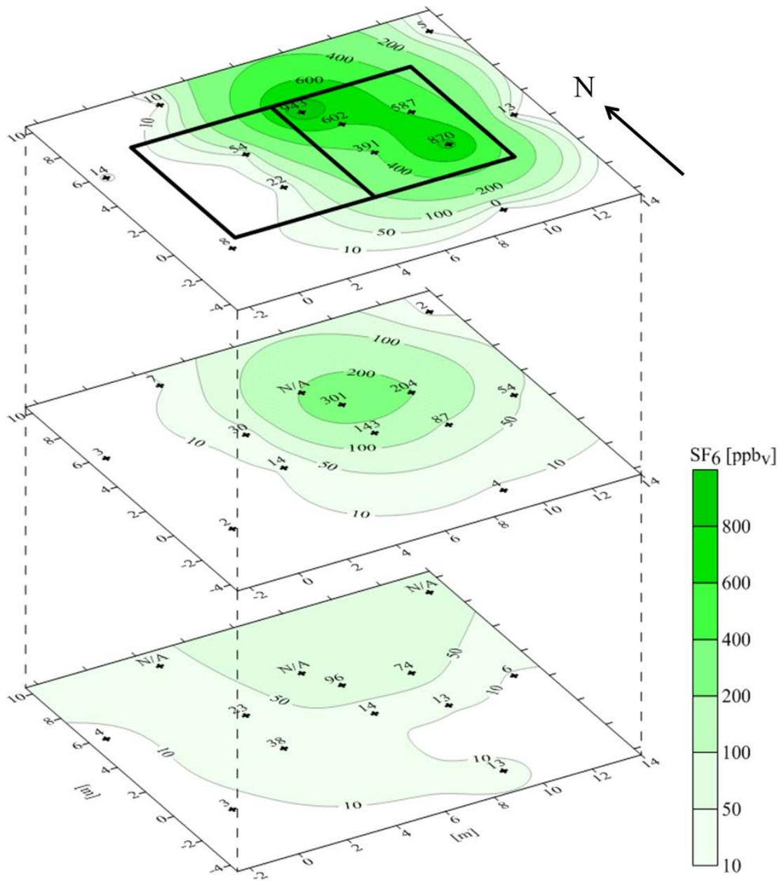
Figure A.37. Contour plots of SF<sub>6</sub> concentrations in soil gas at depths of SS, 0.9 BS, and 1.8 m BS from synoptic soil gas survey in April 2012.
