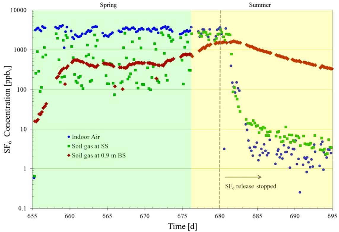
Figure A.42. Instantaneous SF<sub>6</sub> concentrations in indoor air and SS and 0.9 m BS soil gas at location 2 from late May to mid-July 2012 (655 < t < 695 d) showing the results of introduction and removal of an indoor source.
