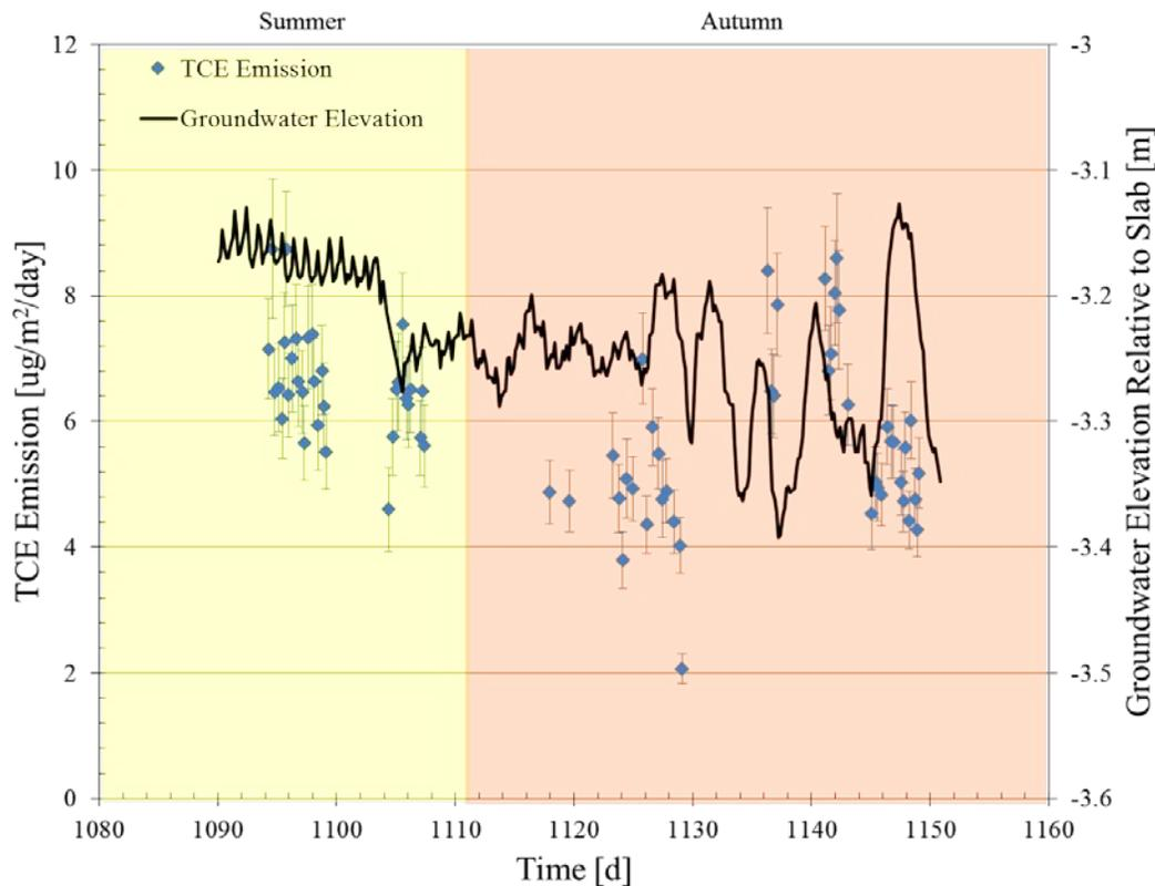
Figure 4.51. Real-time TCE emission rate per unit area ( $F_2$ ) vs. groundwater table elevation during CPM test conditions when the lateral drain valve was closed. Error bars span the uncertainty in each  $F_2$  value calculation.
