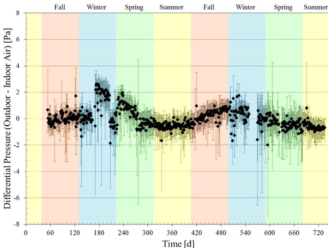
Figure A.51. 24-h average differential pressure values between outdoor air and indoor air with error bars spanning the 10<sup>th</sup> and 90<sup>th</sup> percentiles of the real-time data within each 24-h period.
