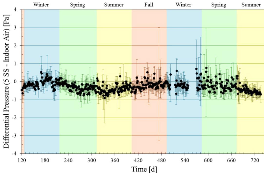
Figure 4.29. Daily 24-h average differential pressures measured between soil gas and indoor air at location 5 with error bars spanning the 10<sup>th</sup> and 90<sup>th</sup> percentile of the real-time data.
