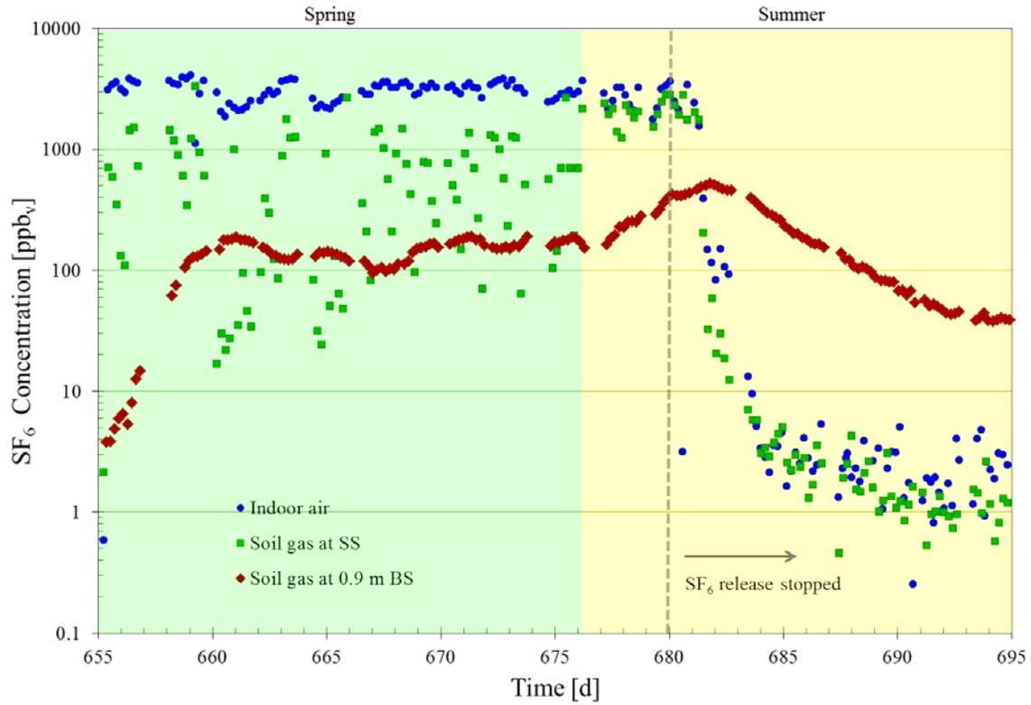
Figure A.44. Instantaneous SF<sub>6</sub> concentrations in indoor air and SS and 0.9 m BS soil gas at location 6 from late May to mid-July 2012 (655 < t < 695 d) showing the results of introduction and removal of an indoor source.
