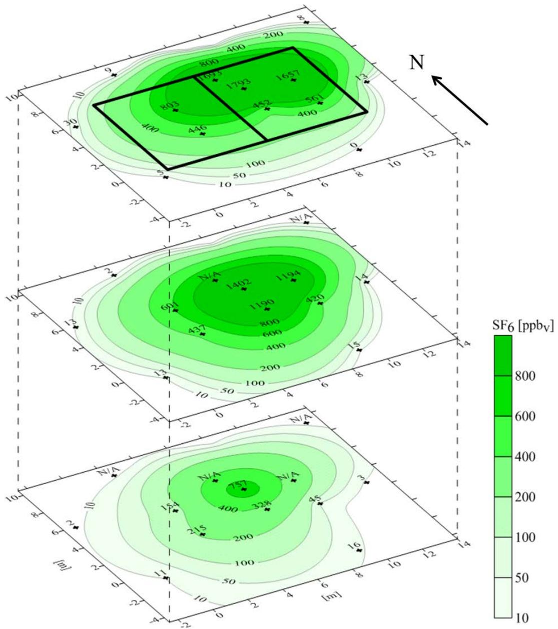
Figure A.31. Contour plots of SF<sub>6</sub> concentrations in soil gas at depths of SS, 0.9 BS, and 1.8 m BS from synoptic soil gas survey in July 2011.
