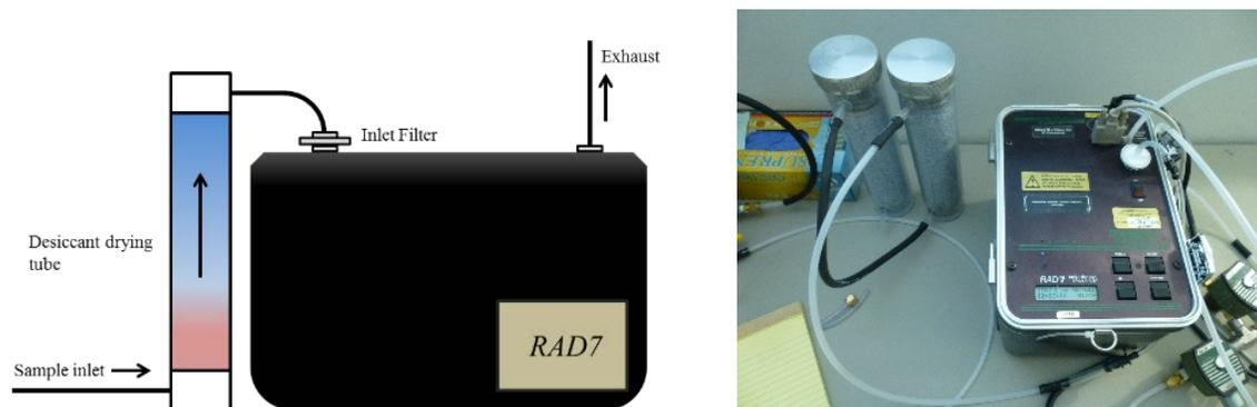
Figure 3.9. Schematic and picture of DurrIDGE RAD7 sampling assembly used for analysis of indoor air and soil gas for radon.
