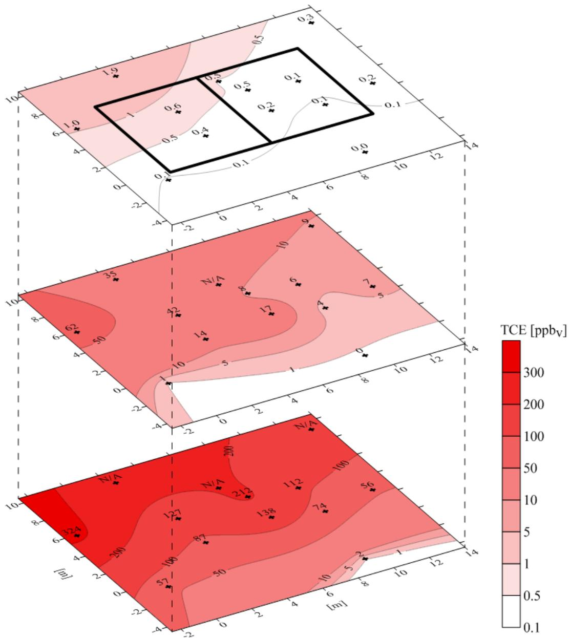
Figure A.17. Multi-depth contour plot of TCE in soil gas for samples collected and analyzed from May 27<sup>th</sup> to May 28<sup>th</sup>, 2012.
