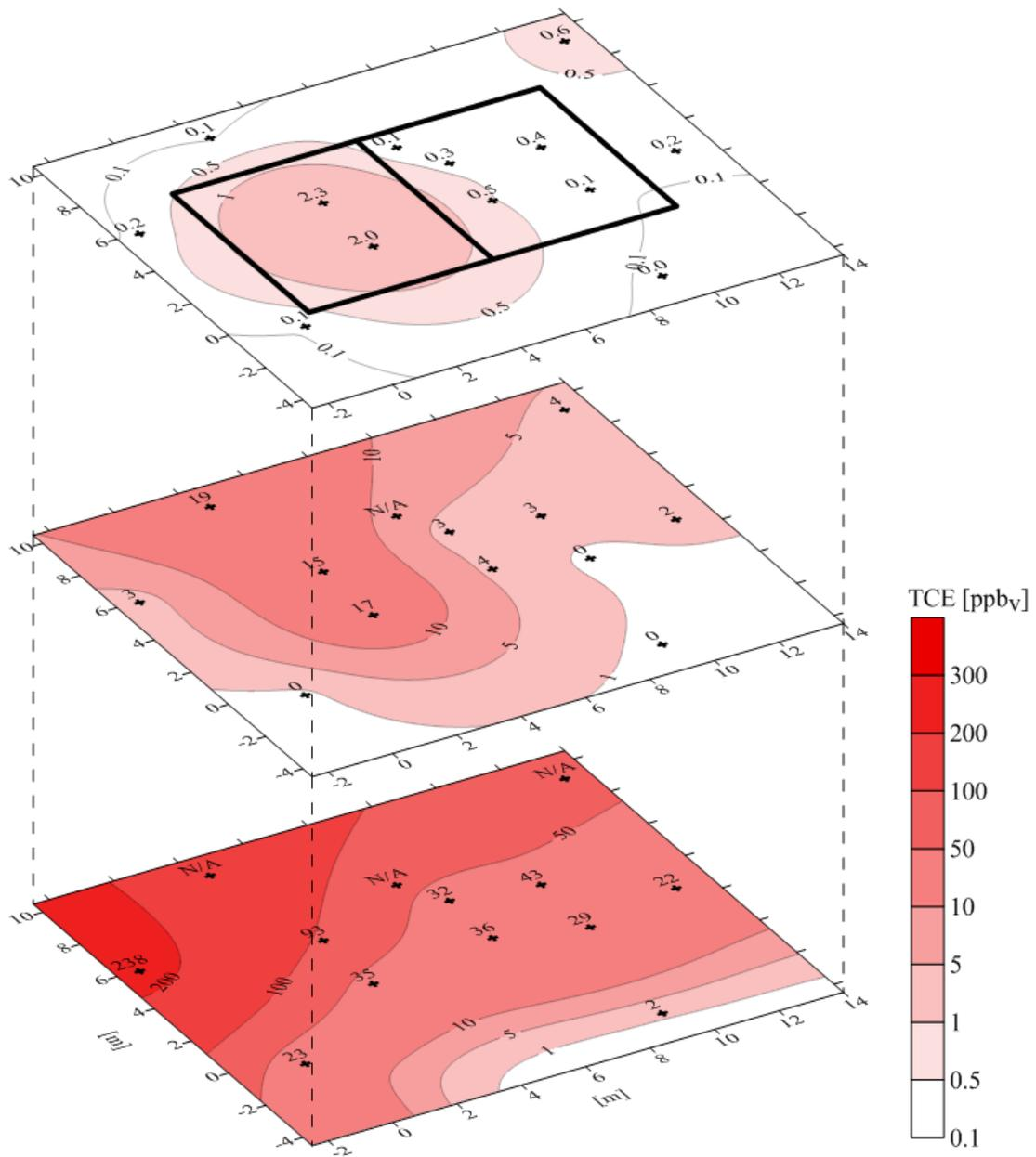
Figure A.5. Multi-depth contour plot of TCE in soil gas for samples collected and analyzed from December 17<sup>th</sup> to December 20<sup>th</sup>, 2010.
