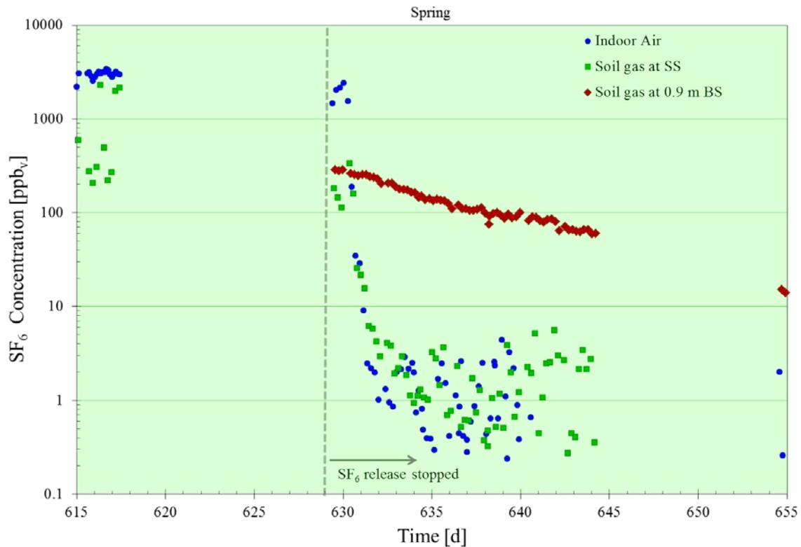
Figure A.39. Instantaneous SF<sub>6</sub> concentrations in indoor air and SS and 0.9 m BS soil gas at location 2 from early to late May 2012 ( $630 < t < 655$  d) showing the results of introduction and removal of an indoor source.
