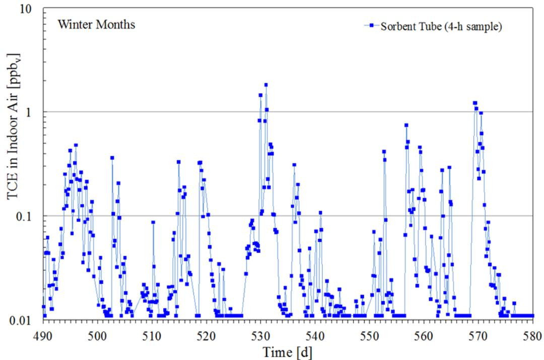
Figure 4.3. Temporal behavior of TCE in indoor air during a VI-active period (values  $\leq 0.011$  ppb<sub>v</sub> are plotted as 0.011 ppb<sub>v</sub>); reproduced from Holton et al. (2013)
