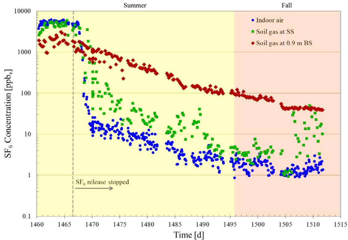
Figure 4.37. Instantaneous SF<sub>6</sub> concentrations in indoor air and soil gas at sub-slab and 0.9 m BS depths at location 6 showing the results of indoor source removal with the land drain lateral pipe valve closed.
