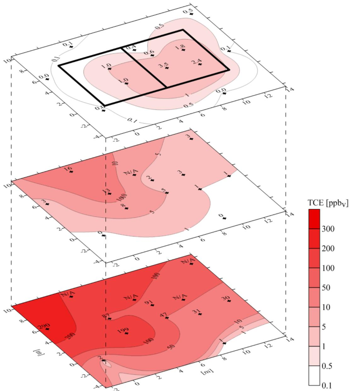
Figure A.7. Multi-depth contour plot of TCE in soil gas for samples collected and analyzed from March 31<sup>st</sup> to April 3<sup>rd</sup>, 2011.
