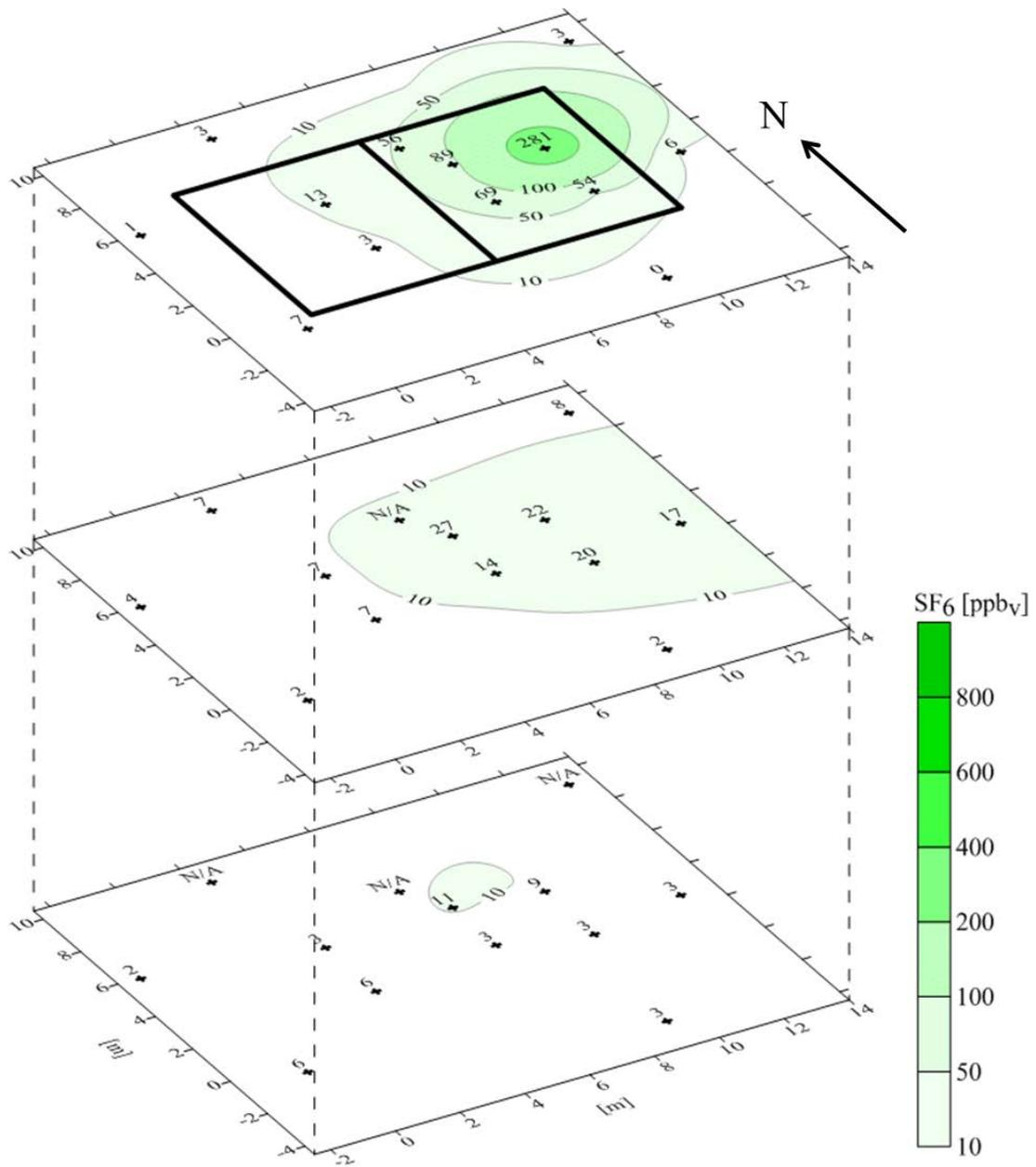
Figure A.35. Contour plots of SF<sub>6</sub> concentrations in soil gas at depths of SS, 0.9 BS, and 1.8 m BS from synoptic soil gas survey in January 2012.
