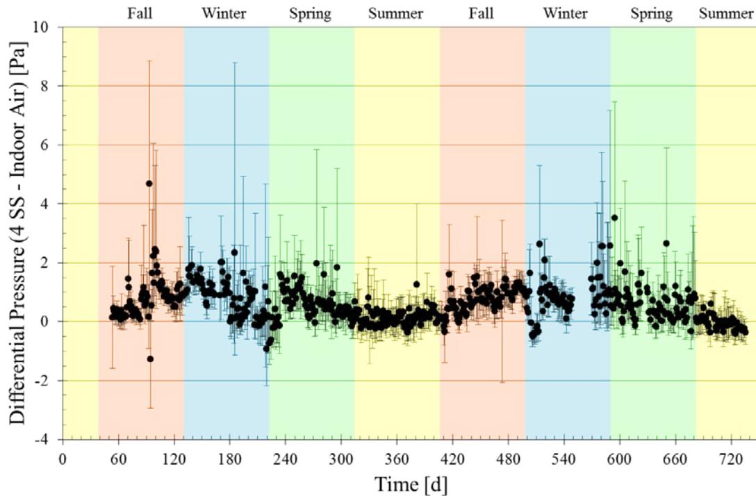
Figure A.52. 24-h average differential pressure values between sub-slab soil gas at location 4 and indoor air with error bars spanning the 90<sup>th</sup> and 10<sup>th</sup> percentile of the daily data sets.
