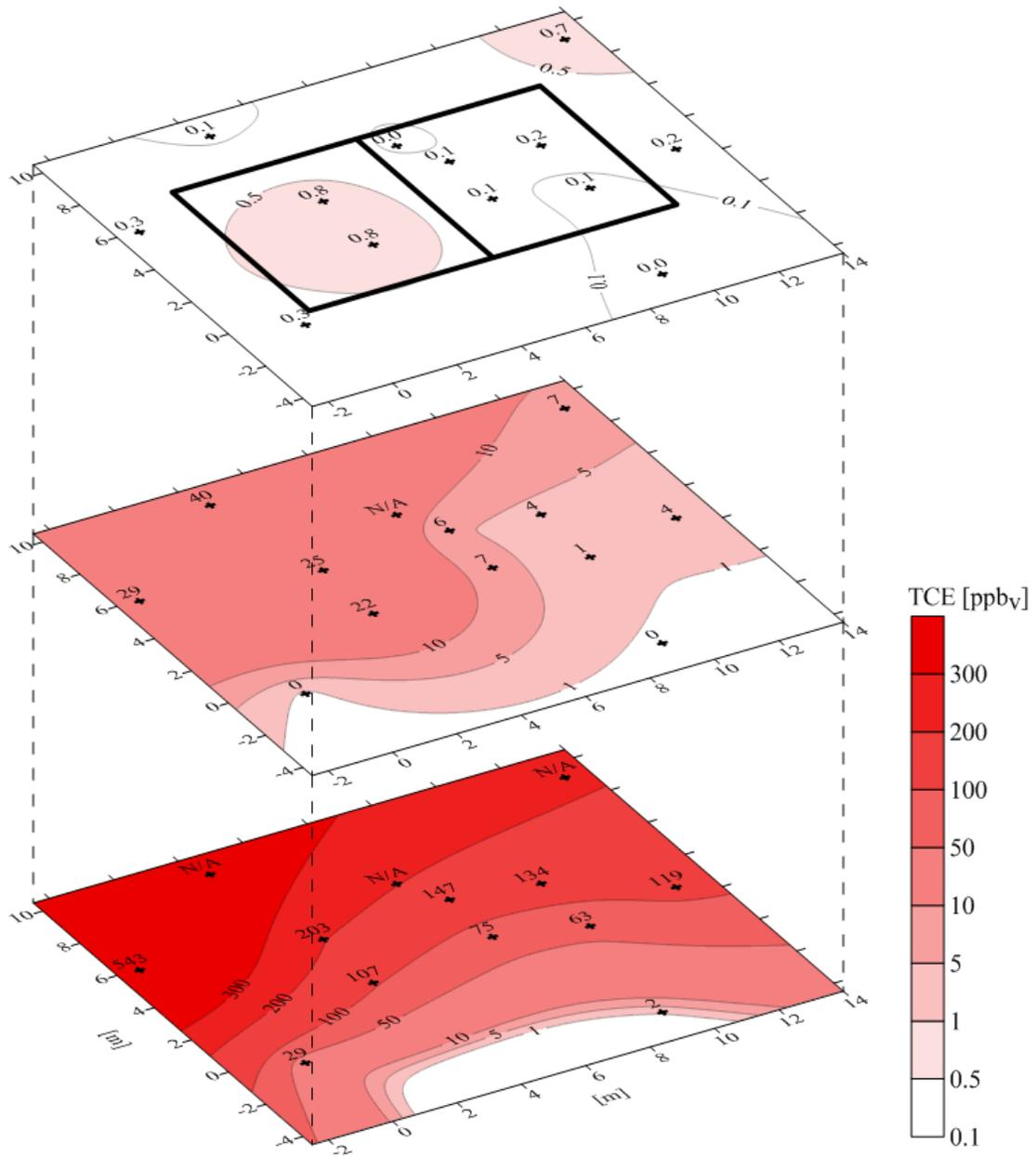
Figure A.4. Multi-depth contour plot of TCE in soil gas for samples collected and analyzed from November 13<sup>th</sup> to November 15<sup>th</sup>, 2010.
