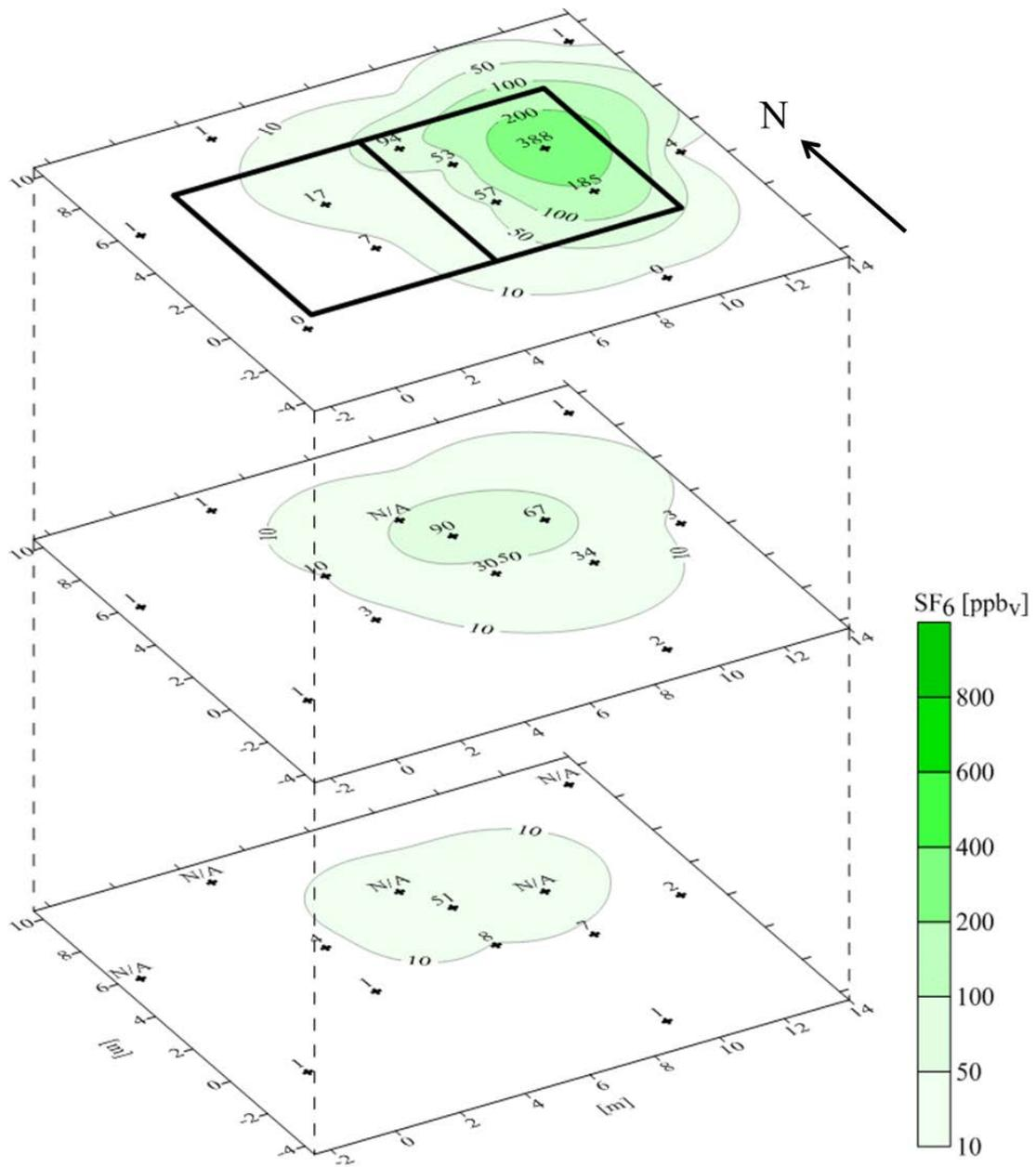
Figure A.29. Contour plots of SF<sub>6</sub> concentrations in soil gas at depths of SS, 0.9 BS, and 1.8 m BS from synoptic soil gas survey in April 2011.
