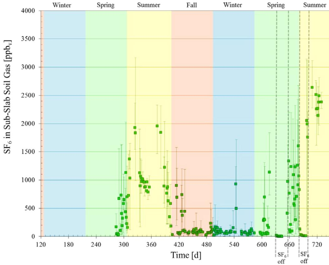
Figure A.25. 24-h averaged SF<sub>6</sub> concentrations sub-slab soil gas at location 5 from winter 2010 through summer 2012 with error bars spanning the daily maximum and minimum values.
