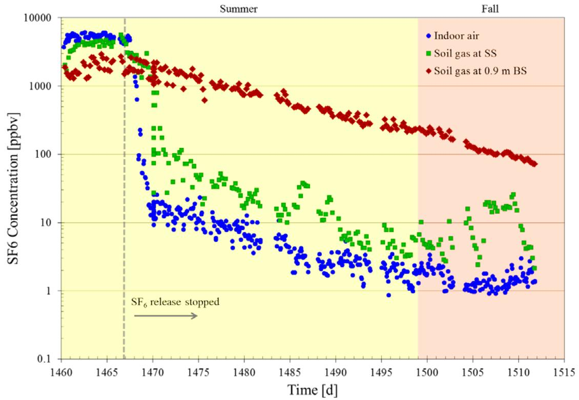
Figure 4.35. Instantaneous SF<sub>6</sub> concentrations in indoor air and soil gas at sub-slab and 0.9 m BS depths at location 3 showing the results of indoor source removal with the land drain lateral pipe valve closed.
