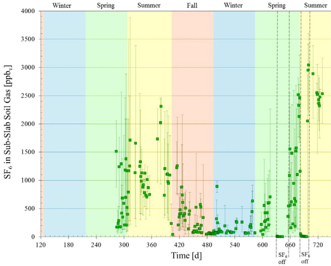
Figure A.23. 24-h averaged SF<sub>6</sub> concentrations sub-slab soil gas at location 2 from winter 2010 through summer 2012 with error bars spanning the daily maximum and minimum values.
