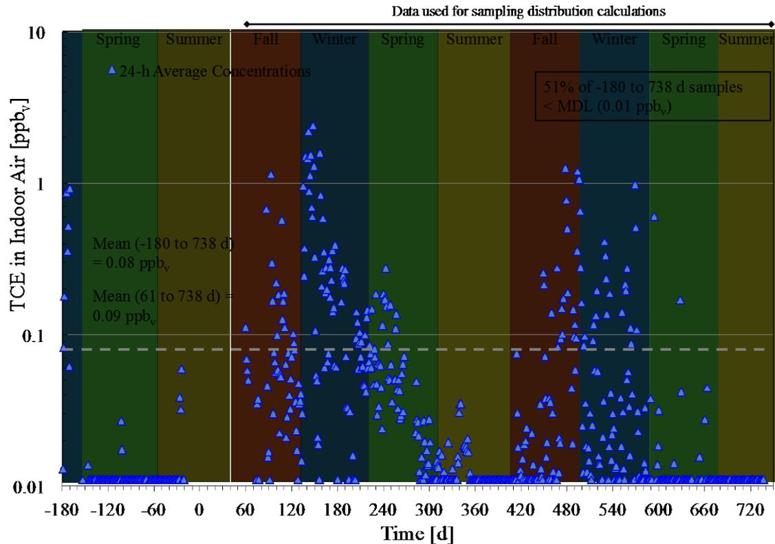
Figure 4.5. Synthetic 24-h sample data set derived from data in Figure 4.1, with the exception that data from  $0 \text{ d} \leq t \leq 60 \text{ days}$  were excluded as they were collected during pressure testing and when a TCE source was present within the house. Note that values  $\leq 0.011 \text{ ppbv}$  are plotted as  $0.011 \text{ ppbv}$ ; plot reproduced from Holton et al. (2013).
