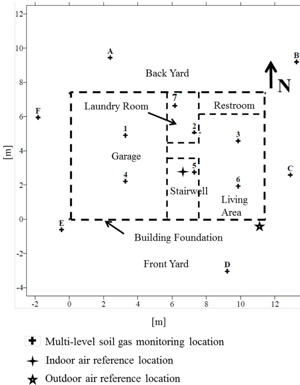
Figure A.50. Schematic of building footprint and monitoring locations.
