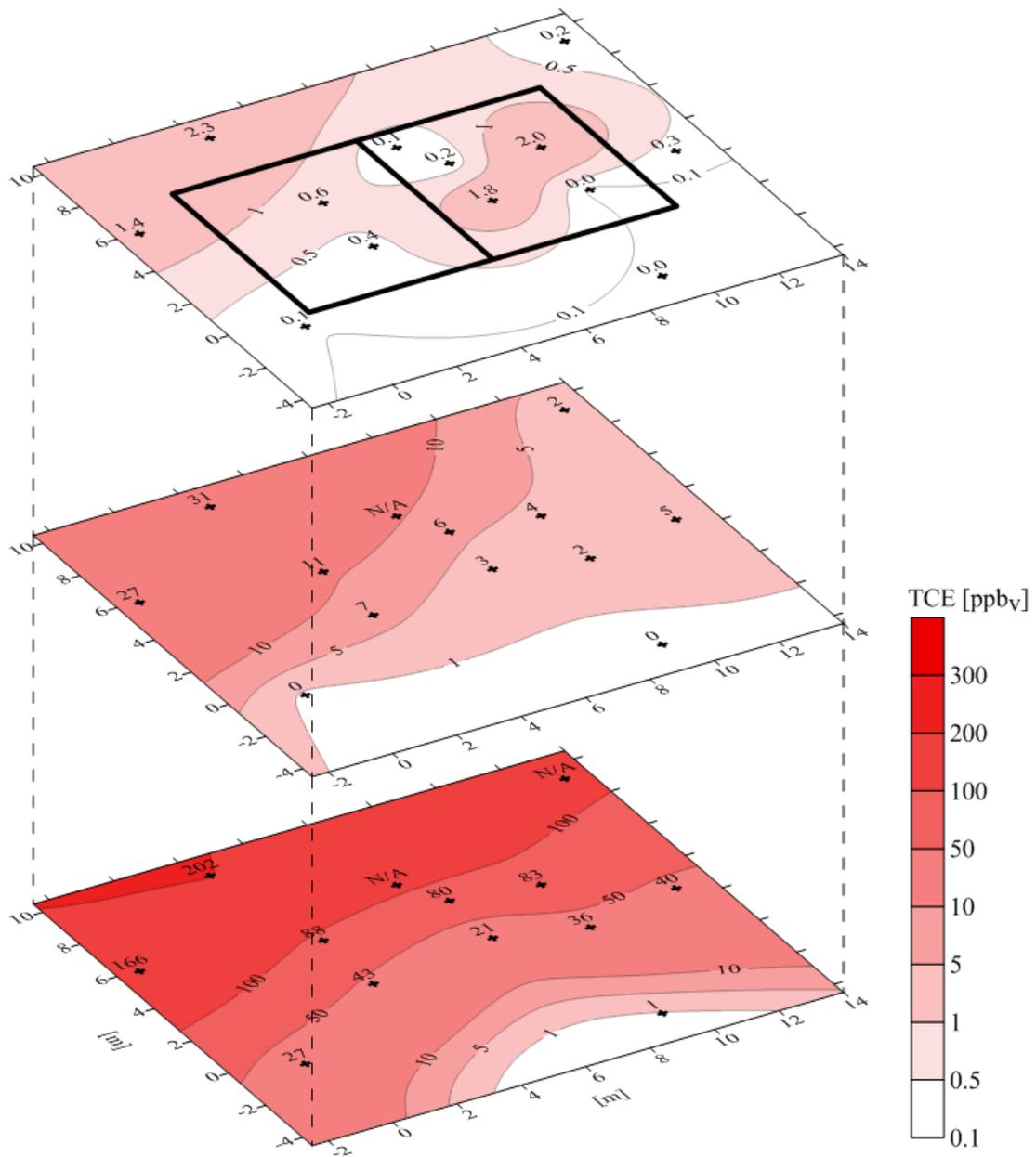
Figure A.14. Multi-depth contour plot of TCE in soil gas for samples collected and analyzed from January 11<sup>th</sup> to January 13<sup>th</sup>, 2012.
