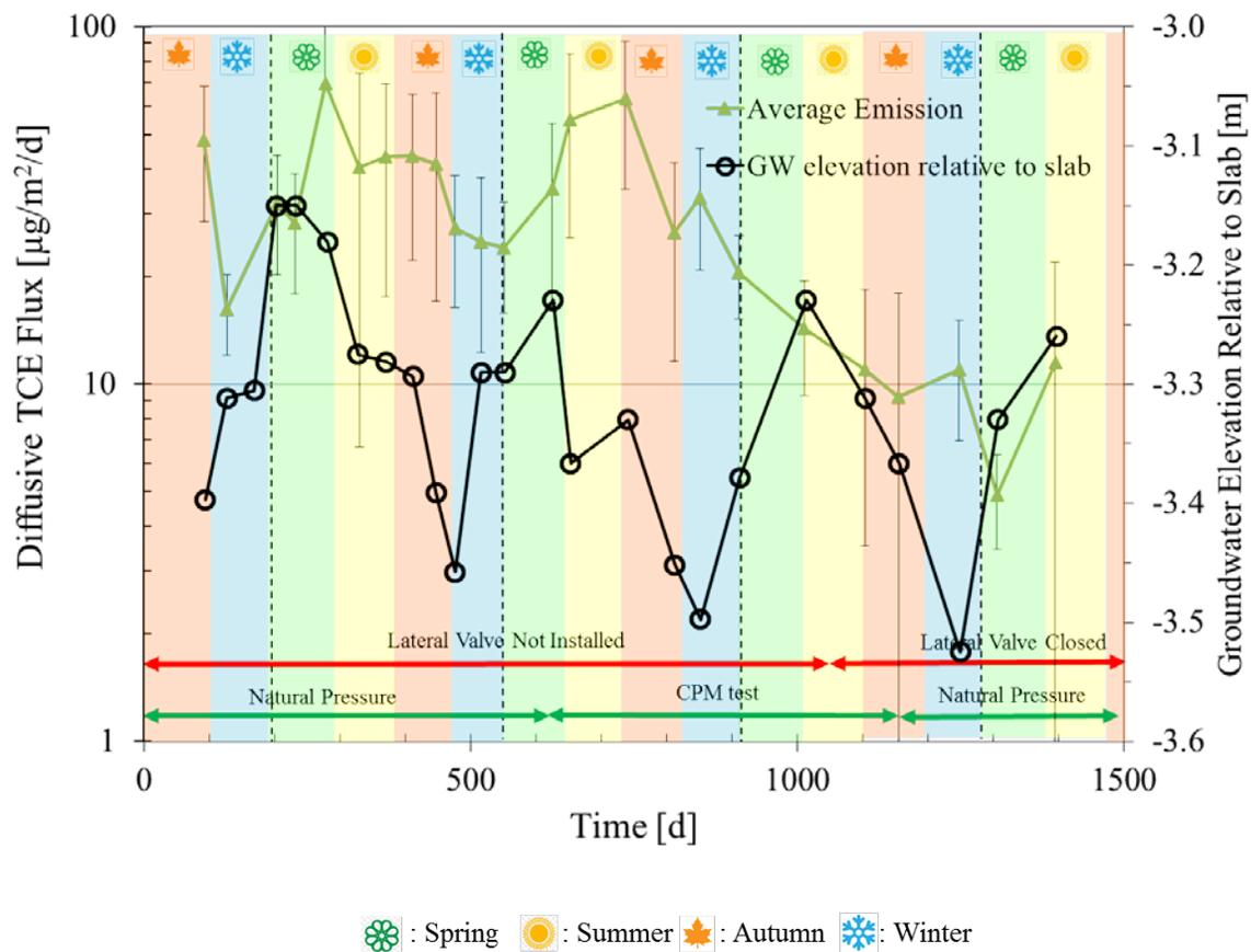
Figure 4.49. Averages of diffusive TCE flux  $F_1$  values (emissions per unit area) for monitoring locations within the building footprint. Error bars span the standard deviation of each average value.
