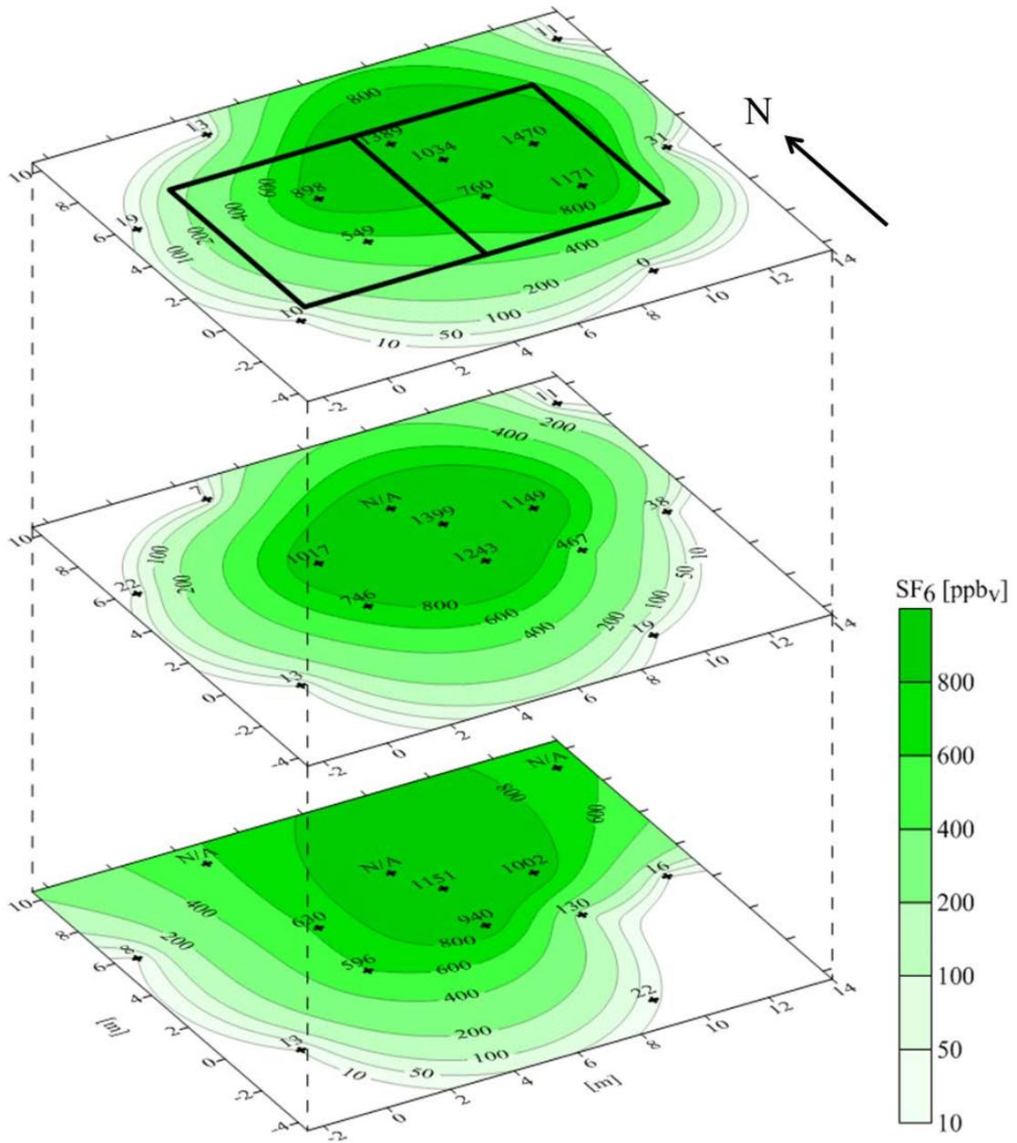
Figure A.32. Contour plots of SF<sub>6</sub> concentrations in soil gas at depths of SS, 0.9 BS, and 1.8 m BS from synoptic soil gas survey in August 2011.
