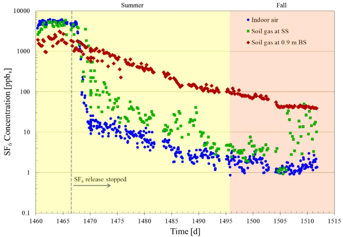
Figure A.46. Instantaneous SF<sub>6</sub> concentrations in indoor air and SS and 0.9 m BS soil gas at location 6 from mid-August to early October 2014 (1460 < t < 1512 d) showing the results of indoor source removal after modification of subsurface pathway.
