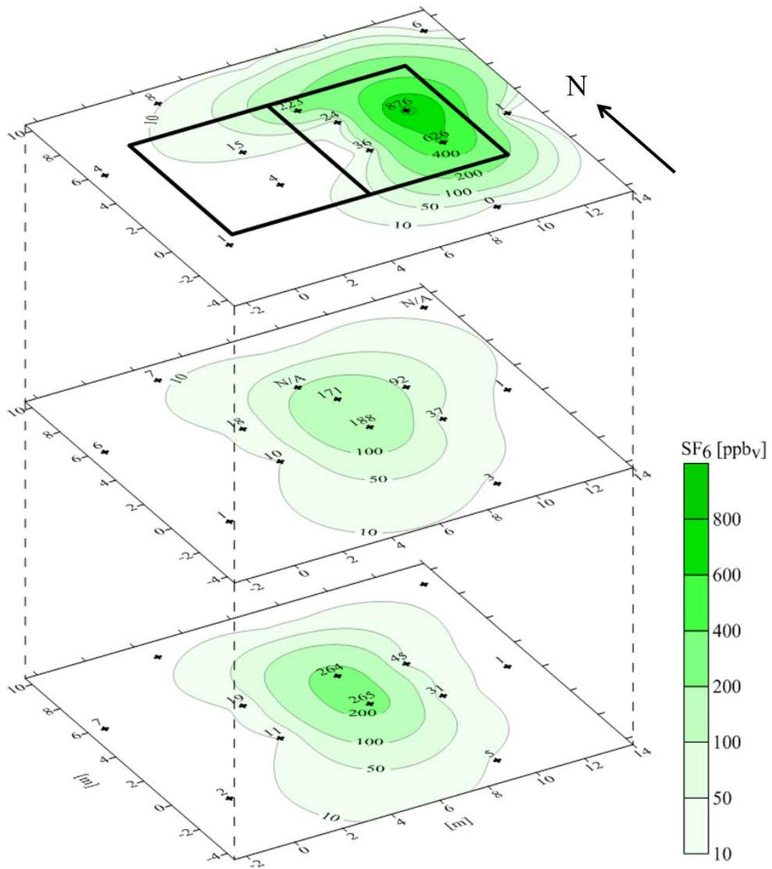
Figure A.33. Contour plots of SF<sub>6</sub> concentrations in soil gas at depths of SS, 0.9 BS, and 1.8 m BS from synoptic soil gas survey in November 2011.
