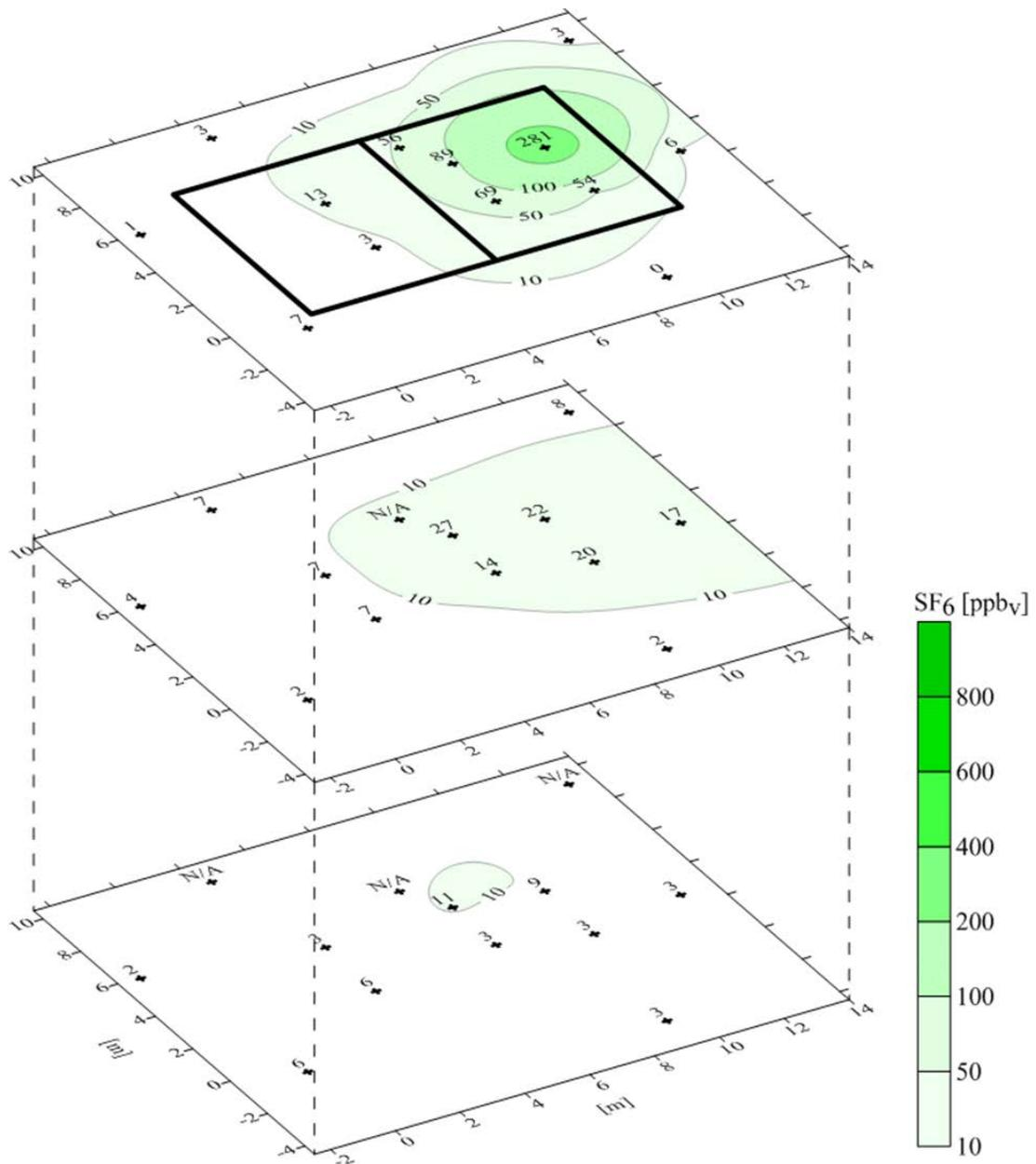
Figure 4.33. SF<sub>6</sub> concentration contour plots for soil gas at sub-slab, 0.9 m BS, and 1.8 m BS depths from t = 515 d.
