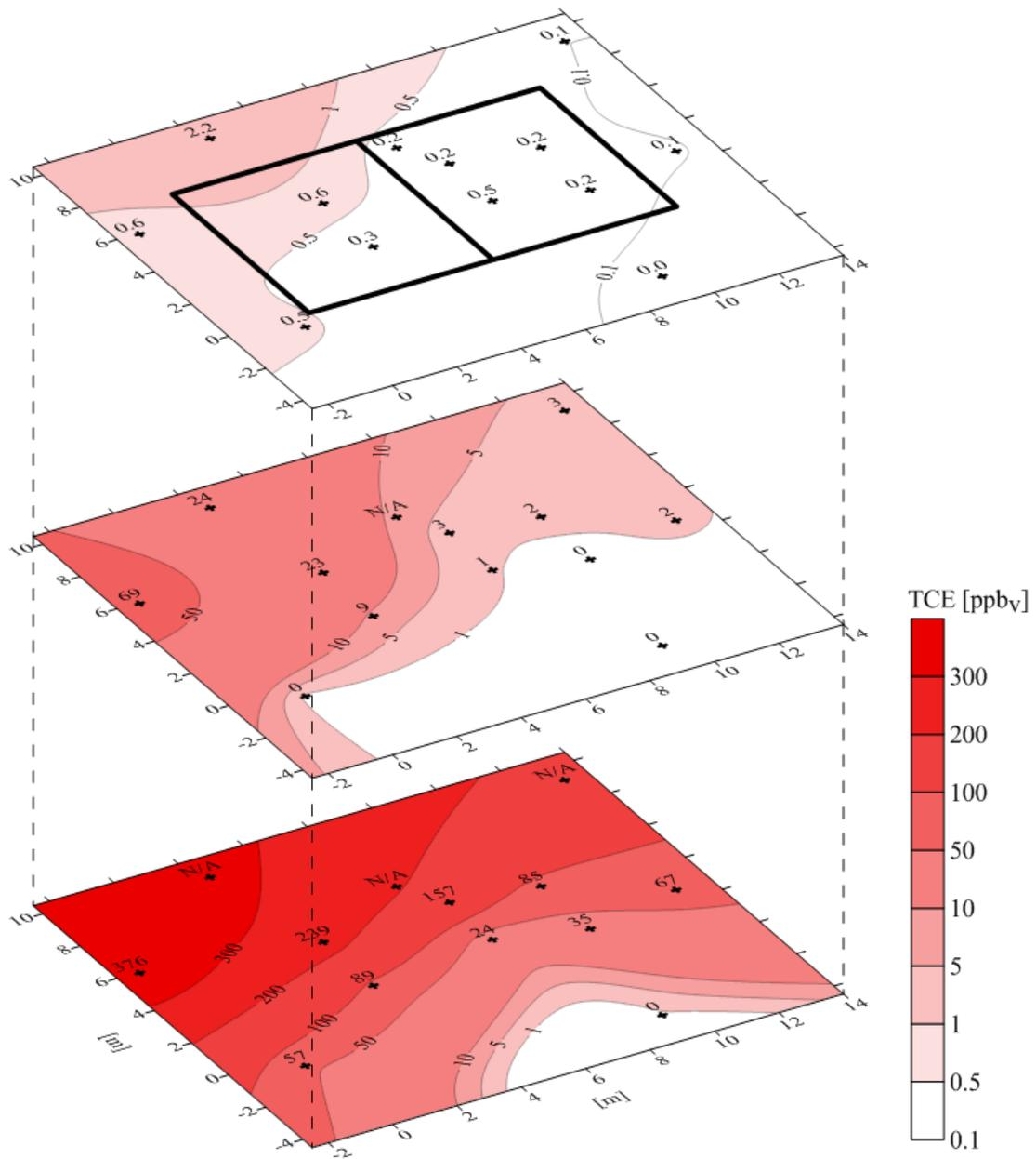
Figure A.12. Multi-depth contour plot of TCE in soil gas for samples collected and analyzed from November 4<sup>th</sup> to November 5<sup>th</sup>, 2011.
