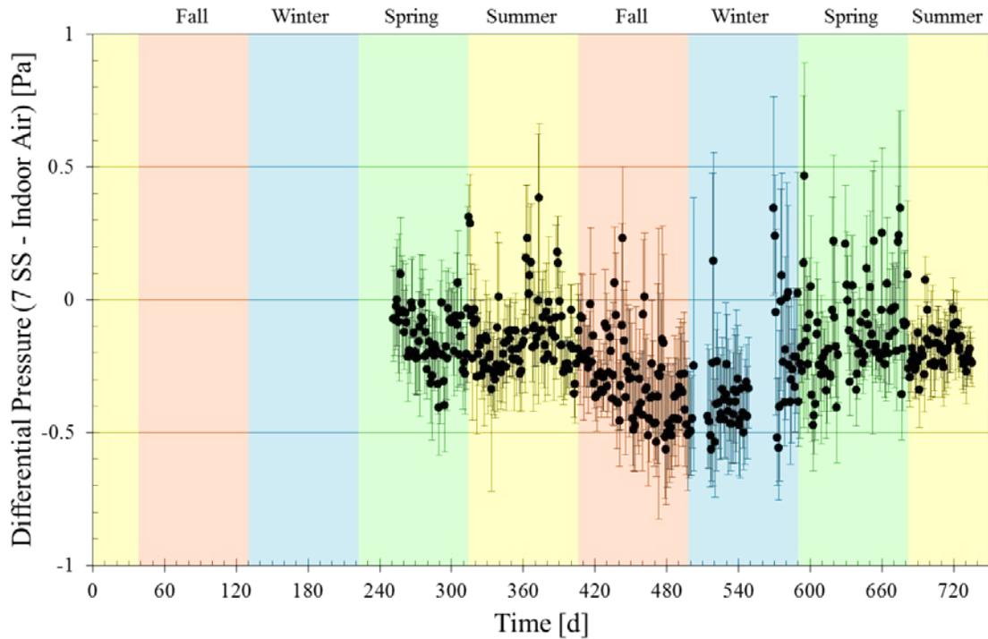
Figure A.54. 24-h average differential pressure values between sub-slab soil gas at location 7 and indoor air with error bars spanning the 90<sup>th</sup> and 10<sup>th</sup> percentile of the daily data sets.
