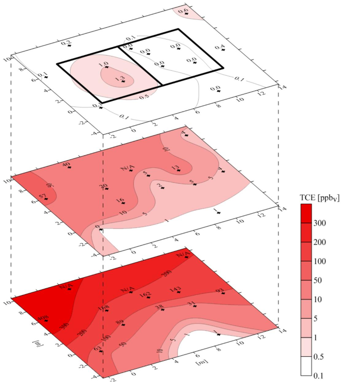
Figure A.10. Multi-depth contour plot of TCE in soil gas for samples collected and analyzed from August 18<sup>th</sup> to August 20<sup>th</sup>, 2011.
