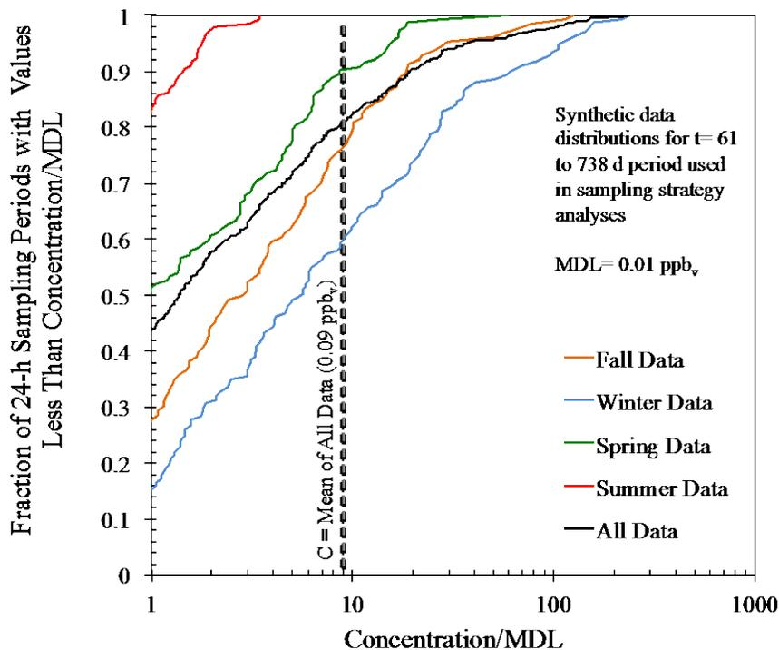
Figure 4.7. Seasonal and aggregate synthetic indoor air concentration distributions derived from the  $t = 61$  d to 738 d synthetic data in Figure 4.4, with concentrations normalized to the MDL assigned to the synthetic data set (0.01 ppb<sub>v</sub>); reproduced from Holton et al. (2013)
