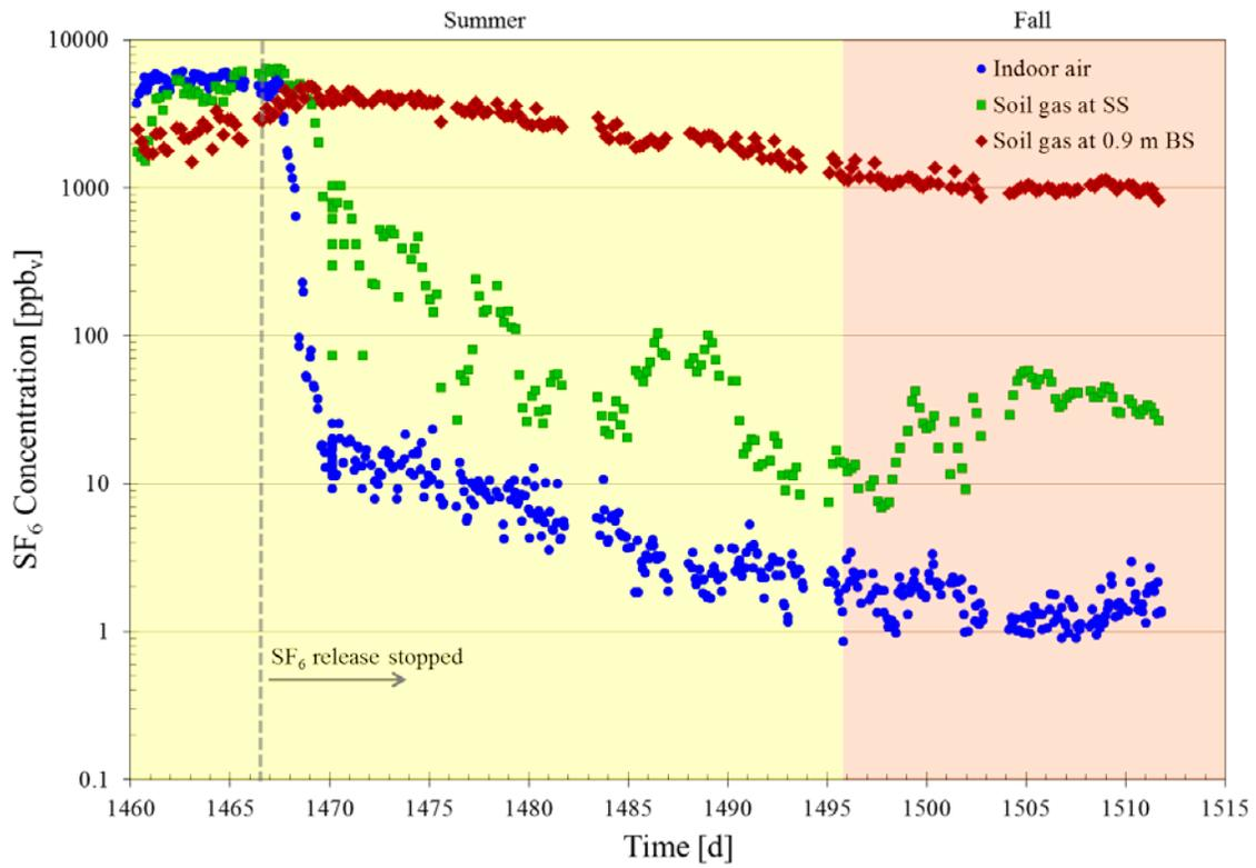
Figure A.45. Instantaneous SF<sub>6</sub> concentrations in indoor air and SS and 0.9 m BS soil gas at location 2 from mid-August to early October 2014 (1460 < t < 1512 d) showing the results of indoor source removal after modification of subsurface pathway.
