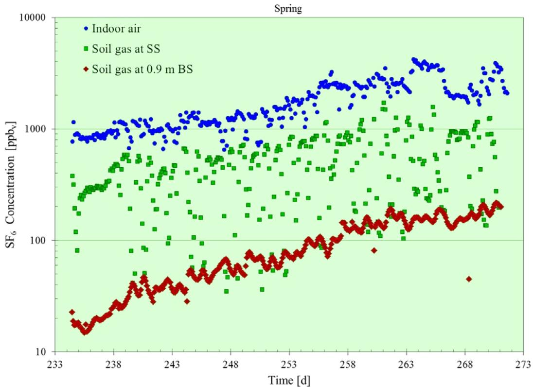
Figure A.27. Instantaneous SS soil gas, 0.9 m BS soil gas, and indoor air SF<sub>6</sub> concentrations at location 3 during spring 2011 for the period  $232 < t < 271$  d.
