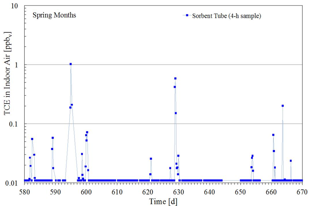
Figure 4.4. Temporal behavior of TCE in indoor air during a VI-dormant period (values  $\leq 0.011$  ppb<sub>v</sub> are plotted as 0.011 ppb<sub>v</sub>); reproduced from Holton et al. (2013)
