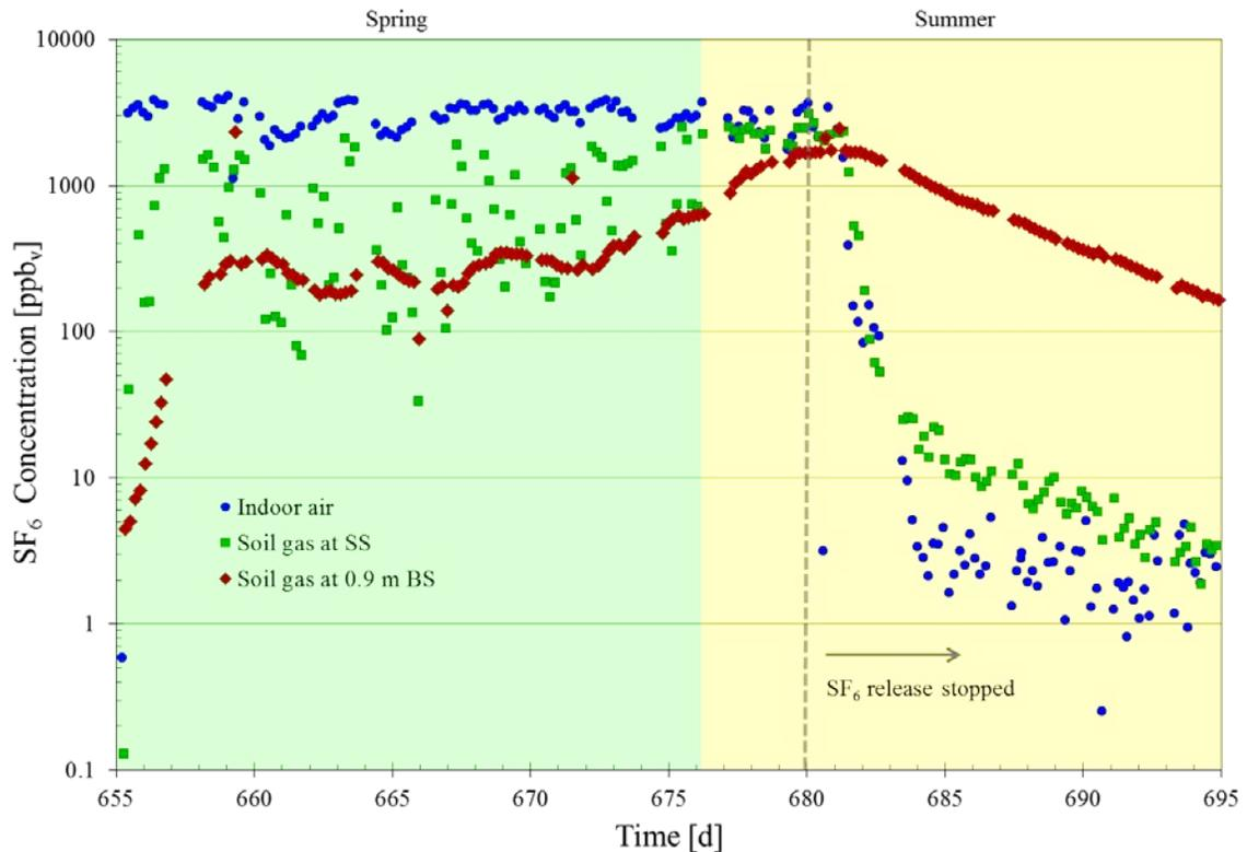
Figure 4.34. Instantaneous SF<sub>6</sub> concentrations in indoor air and sub-slab and 0.9 m BS soil gas at location 3 showing the results of introduction and removal of an indoor source.
