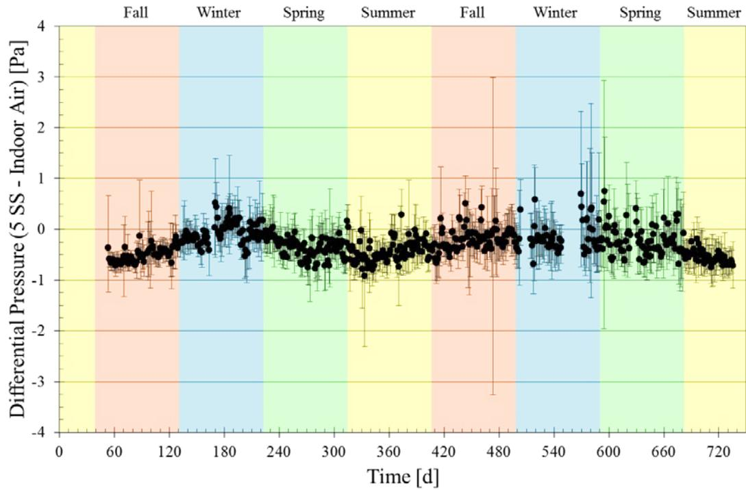
Figure A.53. 24-h average differential pressure values between sub-slab soil gas at location 5 and indoor air with error bars spanning the 90<sup>th</sup> and 10<sup>th</sup> percentile of the daily data sets.
