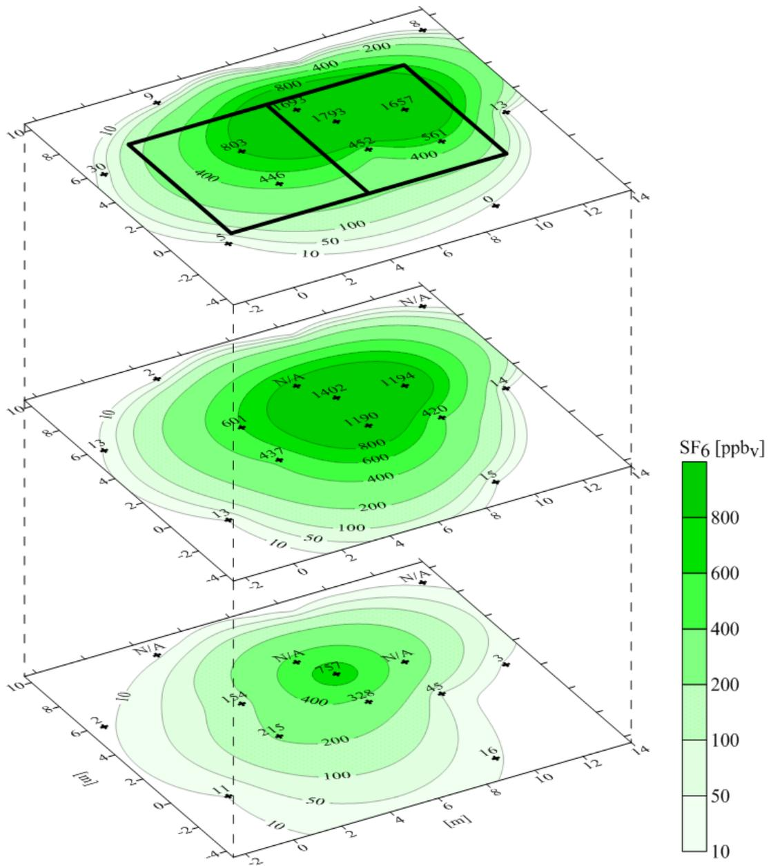
Figure 4.32. SF<sub>6</sub> concentration contour plots for soil gas at sub-slab, 0.9 m BS, and 1.8 m BS depths from t = 329 d.
