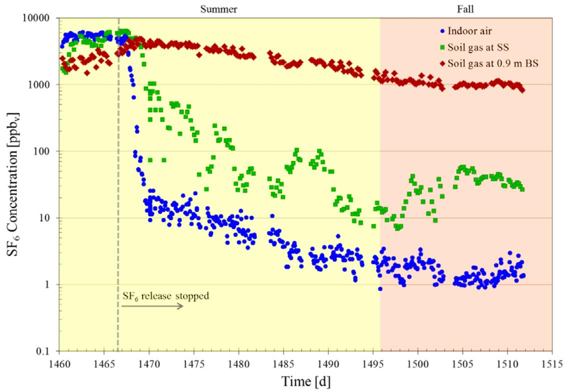
Figure 4.36. Instantaneous SF<sub>6</sub> concentrations in indoor air and soil gas at sub-slab and 0.9 m BS depths at location 2 showing the results of indoor source removal with the land drain lateral pipe valve closed.
