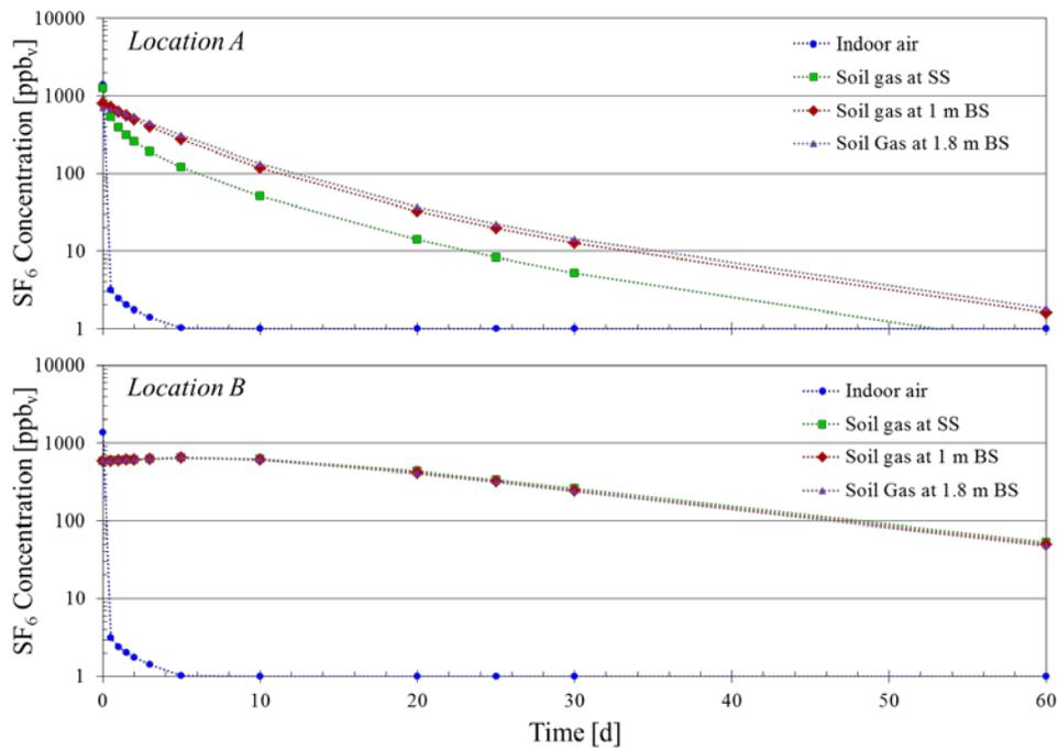
Figure 4.41. Simulation 4 (under-pressurization following indoor source release stop) results showing SF<sub>6</sub> concentrations in indoor air and soil gas at sub-slab (SS) and 1 m BS depths at locations A and B following indoor source removal.
