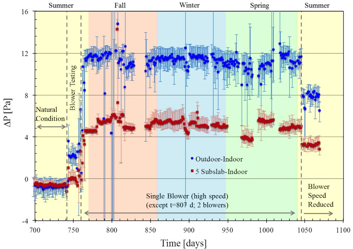
Figure 4.42. 24-h average differential pressure values between indoor air and outdoor air, and indoor air and sub-slab soil gas at location 5 (see Figure 3.2), with error bars spanning the 90<sup>th</sup> and 10<sup>th</sup> percentile of the daily data sets.
