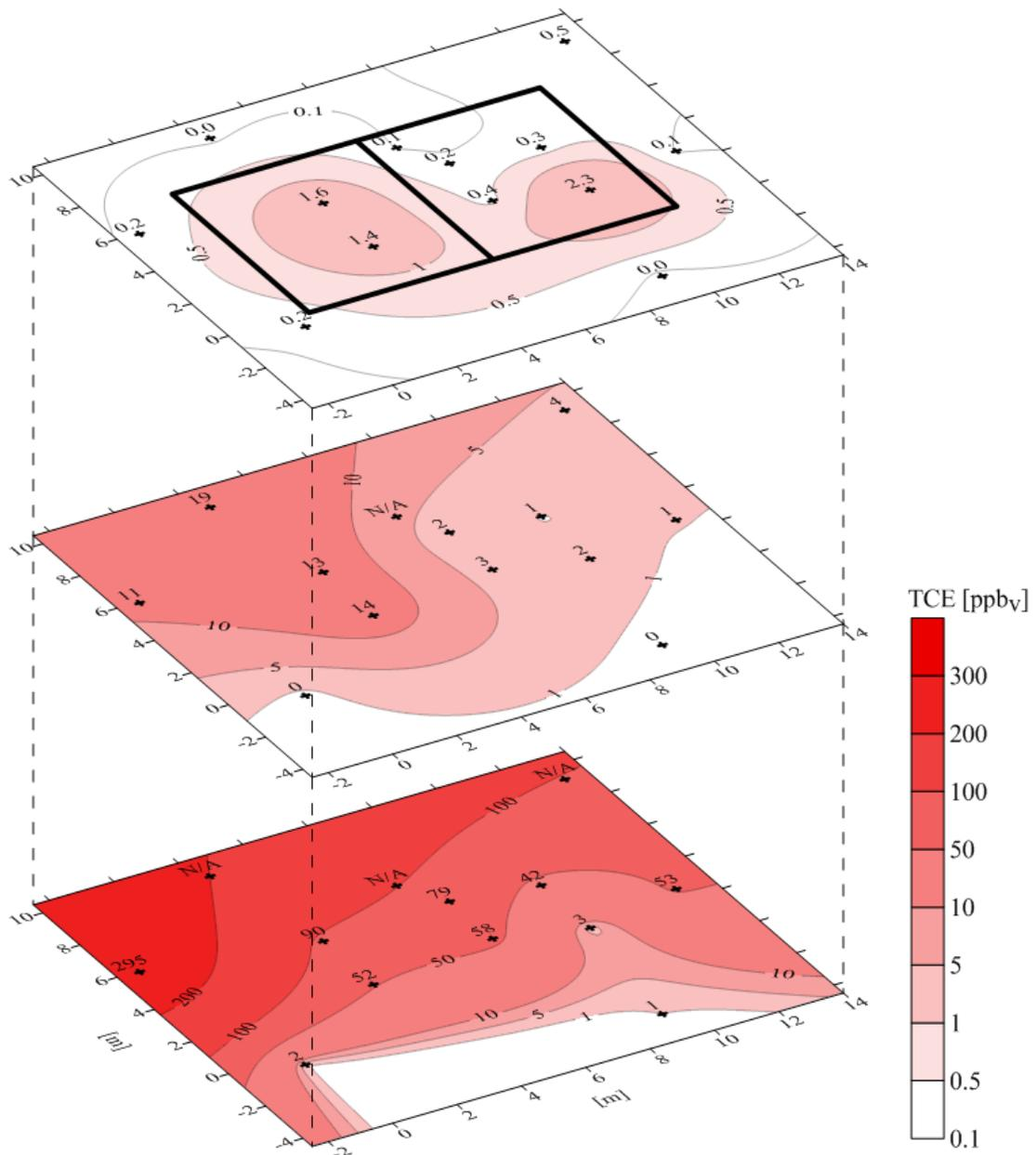
Figure A.6. Multi-depth contour plot of TCE in soil gas for samples collected and analyzed from March 1<sup>st</sup> to March 4<sup>th</sup>, 2011.
