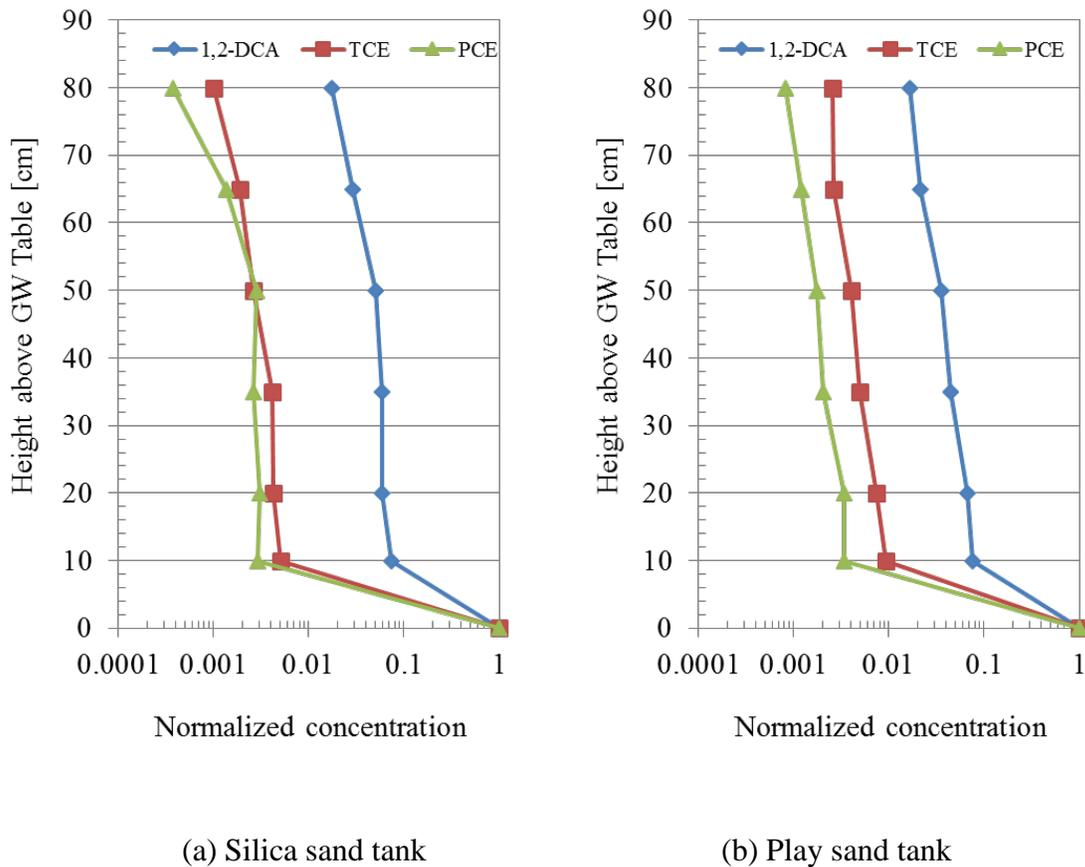
Figure 4.52. Normalized steady-state soil gas profiles for the (a) silica sand tank and (b) play sand tank. Normalized concentrations were obtained by dividing soil gas concentrations at sampling locations by the equivalent gas phase concentrations at the water table.
