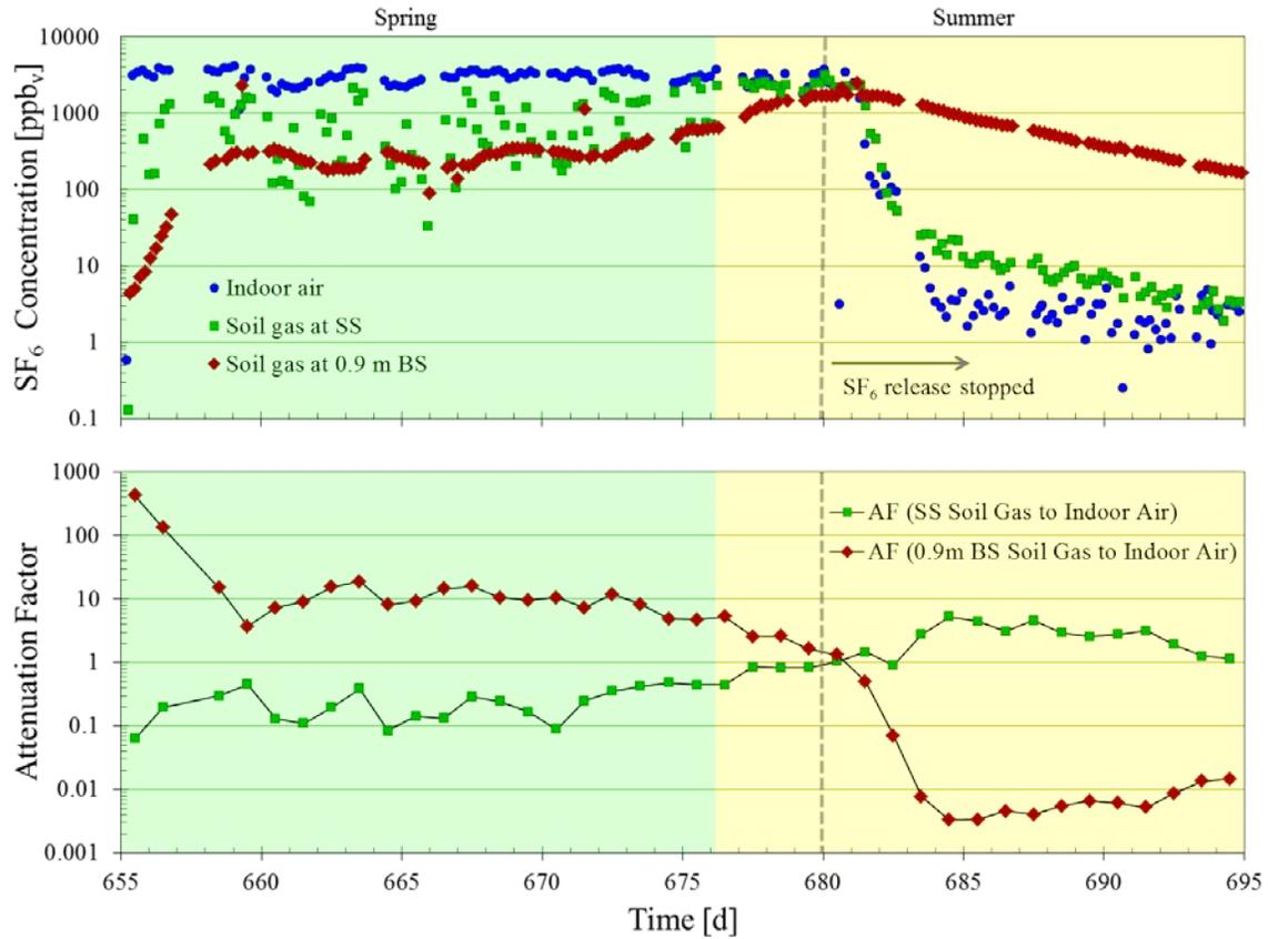
Figure A.43. Instantaneous SF<sub>6</sub> concentrations in indoor air and SS and 0.9 BS soil gas at location 3 from late May to mid-July 2012 (655 < t < 695 d) along with corresponding attenuation factors calculated from 24-h averaged indoor air and soil gas concentrations showing the results of introduction and removal of an indoor source.
