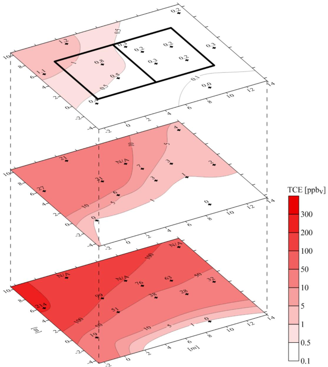
Figure A.15. Multi-depth contour plot of TCE in soil gas for samples collected and analyzed from February 16<sup>th</sup> to February 17<sup>th</sup>, 2012.
