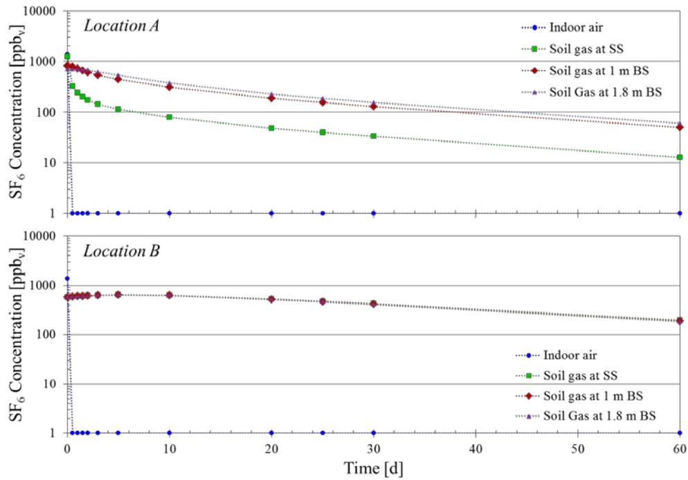
Figure 4.40. Simulation 1 (over-pressurization following indoor source release stop) results showing SF<sub>6</sub> concentrations in indoor air and soil gas at sub-slab (SS) and 1 m BS depths at locations A and B following indoor source removal.
