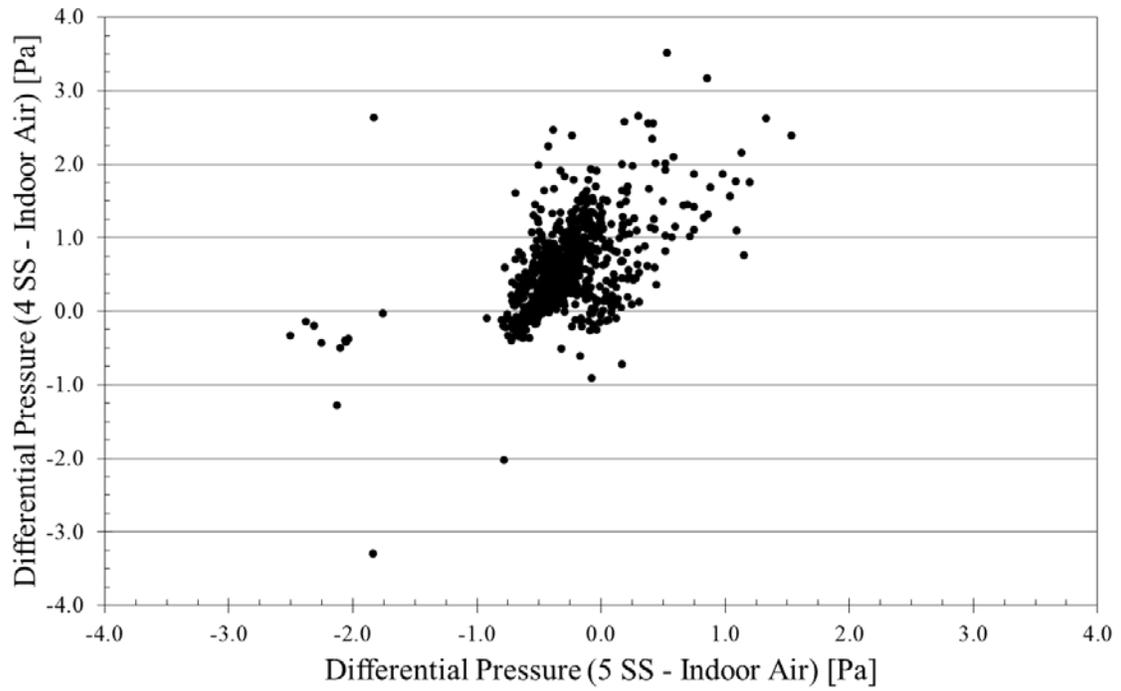
Figure A.58. Comparison of time-matched 24-h average sub-slab to indoor air differential pressure values from location 4 and location 5.
