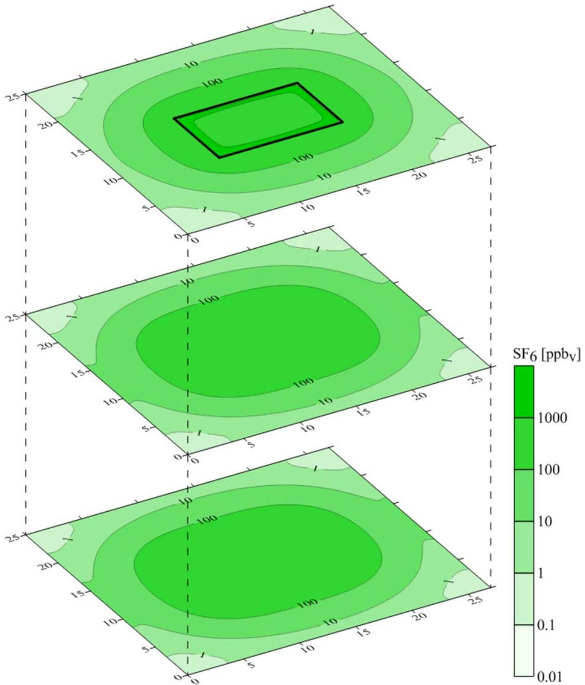
Figure 4.39. Contour plots of simulated SF<sub>6</sub> soil gas concentrations at depths of sub-slab (SS), 1 m BS, and 1.8 m BS following 30 d of indoor source release with a -2 Pa over-pressurization condition.
