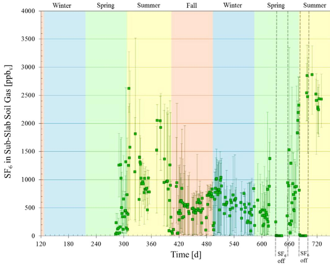
Figure A.26. 24-h averaged SF<sub>6</sub> concentrations sub-slab soil gas at location 6 from winter 2010 through summer 2012 with error bars spanning the daily maximum and minimum values.
