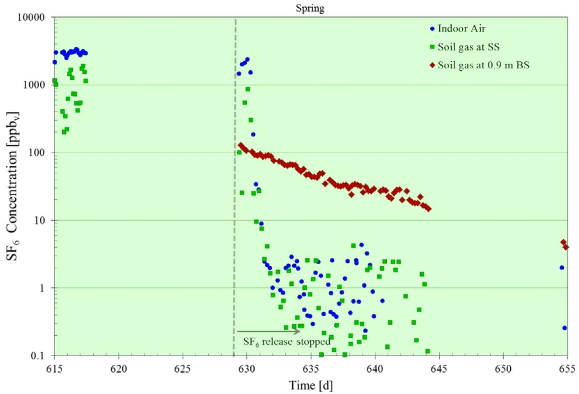
Figure A.41. Instantaneous SF<sub>6</sub> concentrations in indoor air and SS and 0.9 m BS soil gas at location 6 from early to late May 2012 (630 < t < 655 d) showing the results of introduction and removal of an indoor source.
