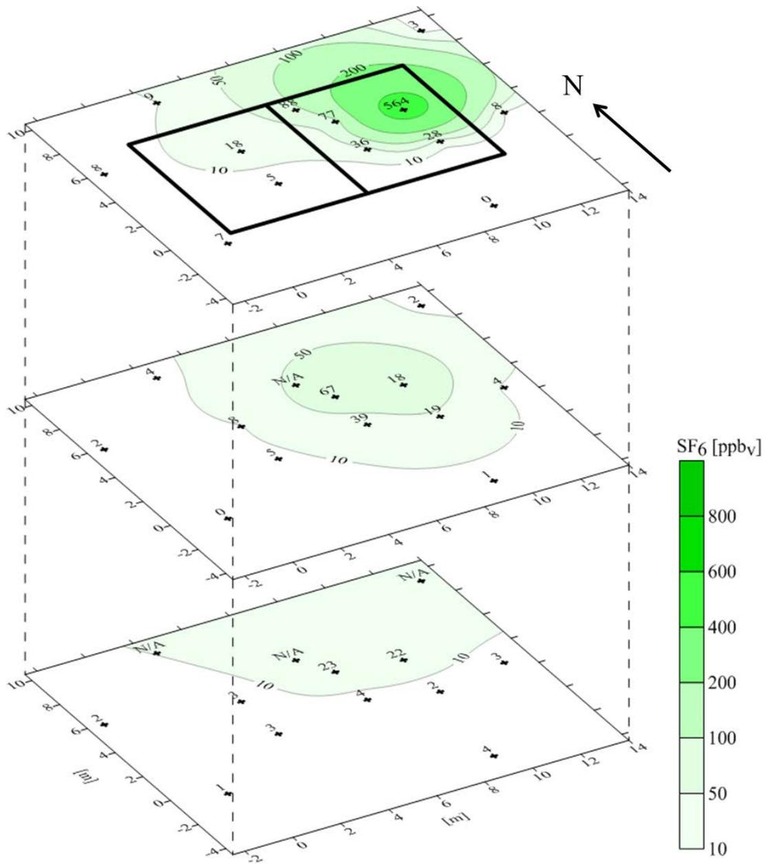
Figure A.36. Contour plots of SF<sub>6</sub> concentrations in soil gas at depths of SS, 0.9 BS, and 1.8 m BS from synoptic soil gas survey in February 2012.
