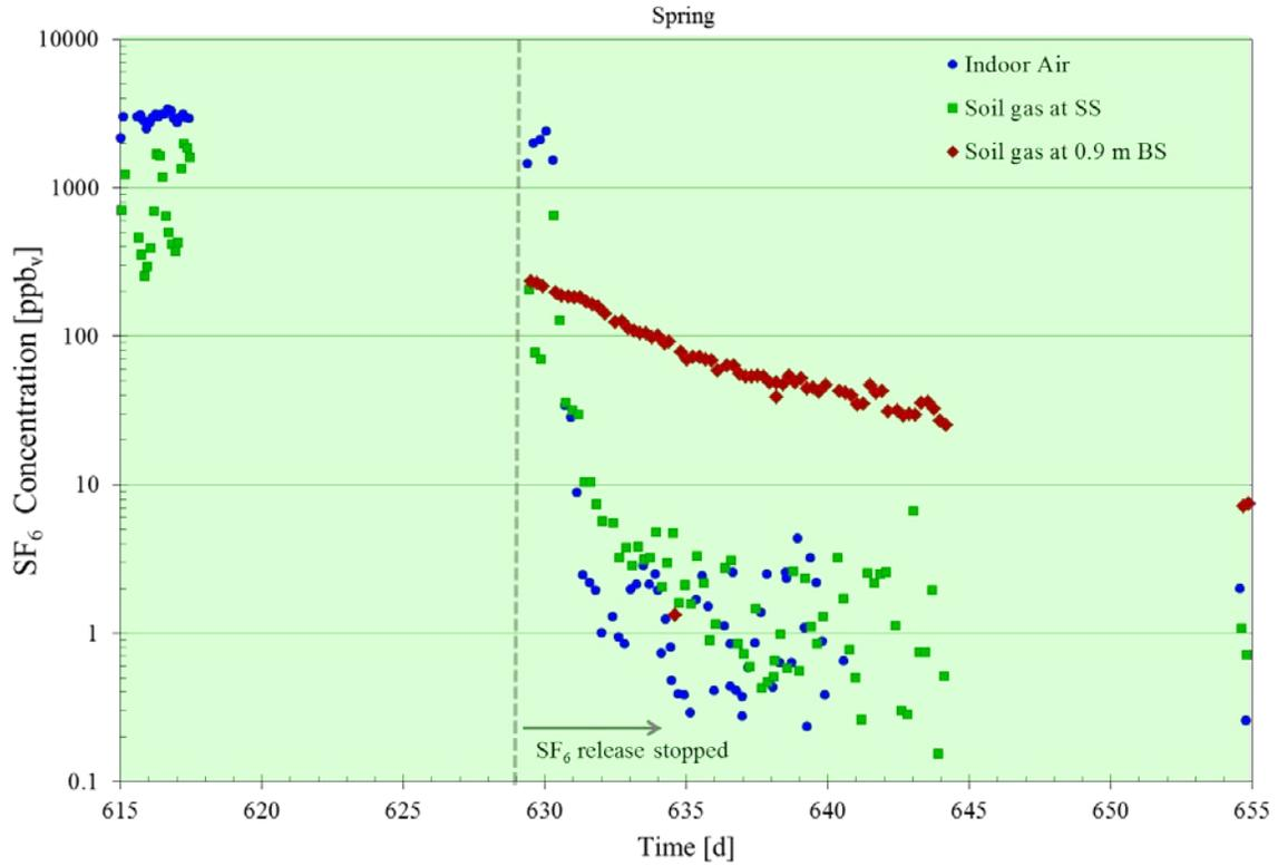
Figure A.40. Instantaneous SF<sub>6</sub> concentrations in indoor air and SS and 0.9 m BS soil gas at location 3 from early to late May 2012 (630 < t < 655 d) showing the results of introduction and removal of an indoor source.
