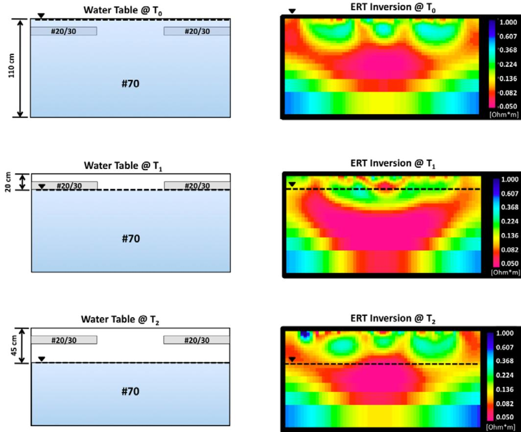
**Figure 5.41:** Schematic of packing configuration #2 and the ERT inversions with the water table set at the upper, mid and lower elevations ( $T_0$ ,  $T_1$ , and  $T_3$ , respectively). The ERT inversion color gradients represent resistivity values with ranges from 0.05  $\text{Ohm}\cdot\text{m}$  to 1.00  $\text{Ohm}\cdot\text{m}$ .
