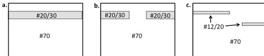
**Figure 4.13 (a-c).** Schematic of geophysical sand tank packing configurations: (a) *Configuration #1* – Fine matrix (#70 sand) with coarse continuous horizontal layer (#20/30 sand, 10 cm. thick). (b) *Configuration #2* – Fine matrix (#70 sand) with coarse discontinuous horizontal layer (#20/30 sand, 10 cm. thick). (c) *Configuration #3* - Fine matrix (#70 sand) with shallow and deep thin discontinuous horizontal layers (#12/20, 4 cm. thick). Figures not drawn to scale.
