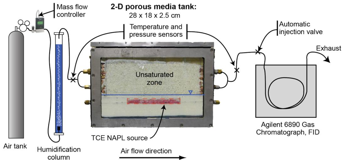
**Figure 4.2:** Experimental Apparatus and Tank Packing for NAPL volatilization experiments. Case 1 presents the occluded NAPL experiment (see section 4.3.3) and case 2 presents the exposed NAPL experiment (see section 4.3.4). The free surface elevation relative to the bottom of the tank is presented in the figures, and in both cases is below the tank bottom (under suction).
