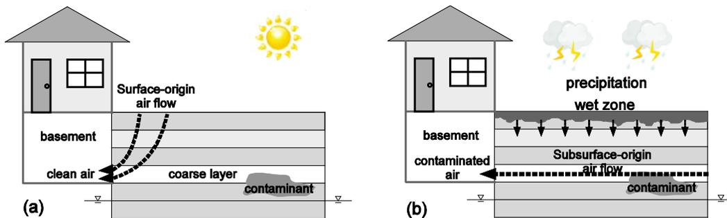
**Figure 5.16.** Schematic images of air flow pathway dynamics under different climatic conditions at the soil surface; (a) surface-origin air flow with small area of influence under no rainfall conditions, (b) subsurface-origin air flow with larger area of influence under rainfall conditions.
