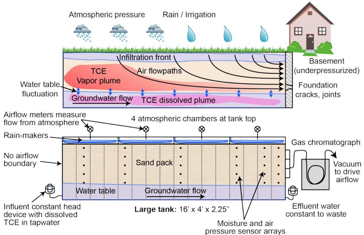
**Figure 4.9:** Conceptual model for intermediate scale tank for integrated dynamic flow and vapor transport experiments with tank schematic.
