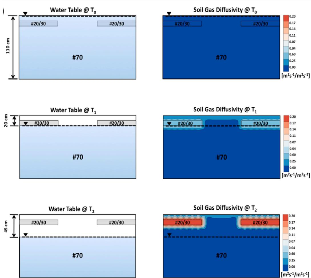
**Figure 5.38:** Schematic of packing configuration #2 and the soil gas diffusivity simulations (Moldrup et al., 2000) with the water table set at the upper, mid and lower elevations ( $T_0$ ,  $T_1$ , and  $T_2$ , respectively).
