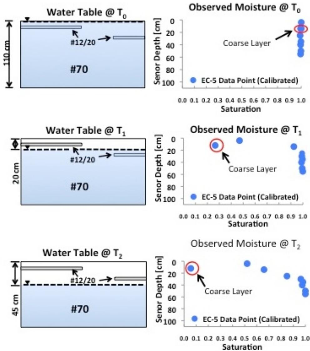
**Figure 5.36:** Schematic of packing configuration #3 and the calibrated volumetric moisture content data (e.g. Sakaki et al., 2011) with the water table set at the upper, mid and lower elevations ( $T_0$ ,  $T_1$ , and  $T_2$ , respectively).
