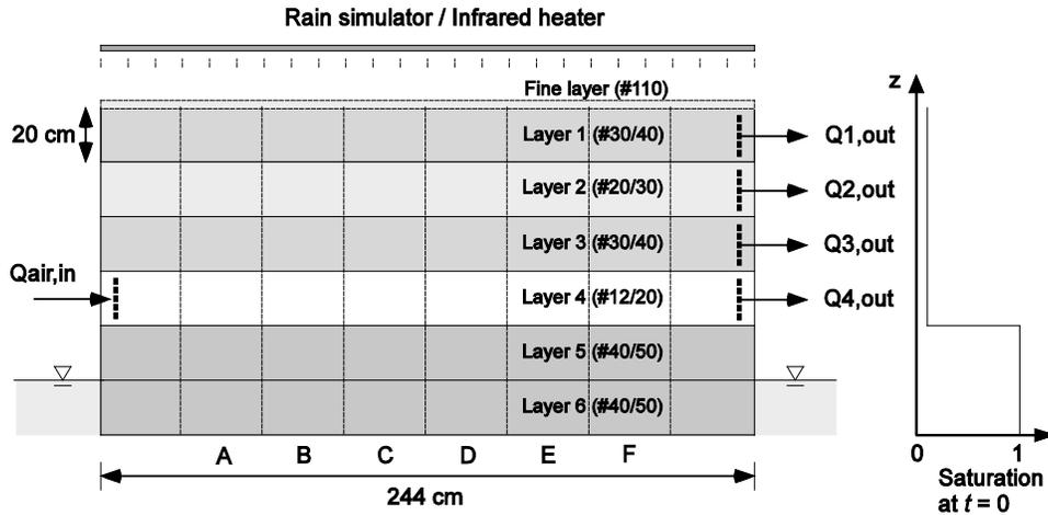
**Figure 4.7:** Schematic view of the two-dimensional tank for dynamic soil moisture experiments. Saturation profile is only schematic. Note that the air flow is reversed in the rainfall and heat experiments.
