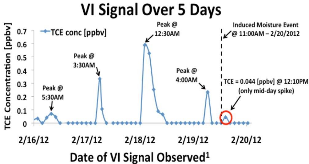
**Figure 5.46:** Graph of the VI signal (TCE in ppbv) entering study site building over a five-day window that included our field demonstration and simulated precipitation event. [Ongoing VI site study by Johnson et al., 2010-2012].
