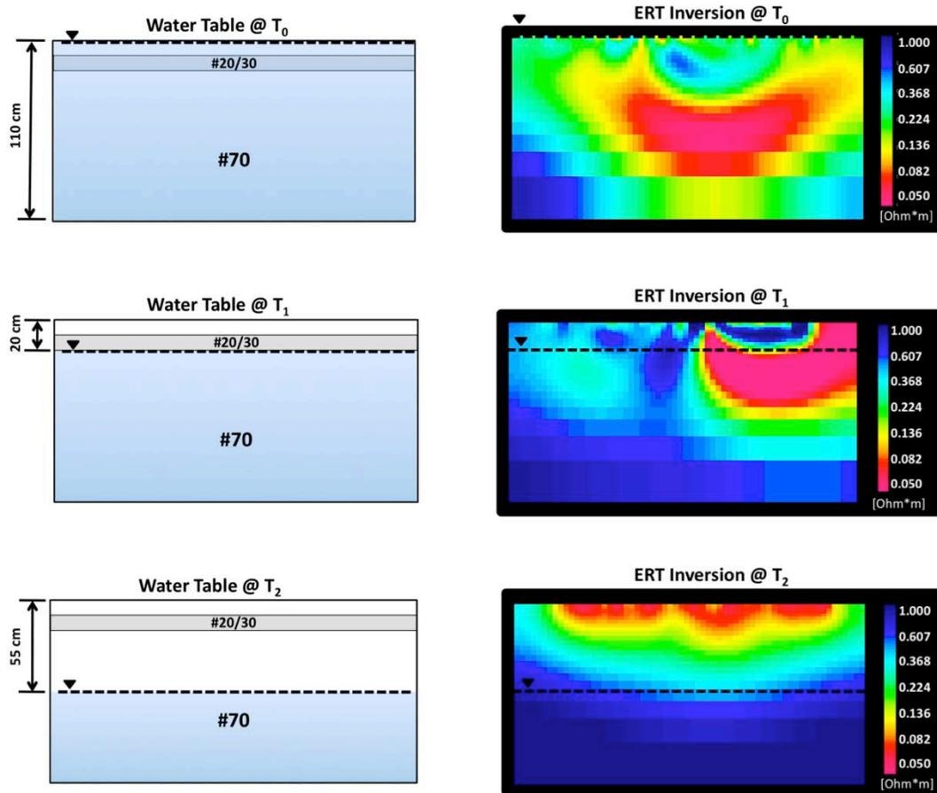
**Figure 5.40:** Schematic of packing configuration #1 and the ERT inversions with the water table set at the upper, mid and lower elevations ( $T_0$ ,  $T_1$ , and  $T_3$ , respectively). The ERT inversion color gradients represent resistivity values with ranges from 0.05  $\text{Ohm}\cdot\text{m}$  to 1.00  $\text{Ohm}\cdot\text{m}$ .
