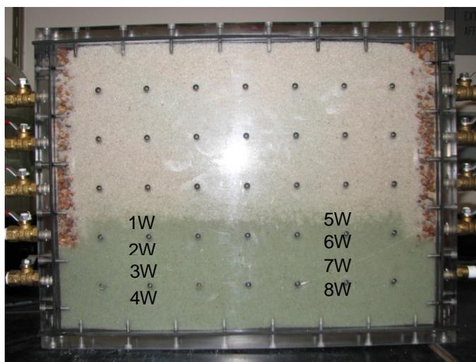
**Figure 4.6:** Aqueous phase sampling locations within the tank. Green color of the liquid indicates the groundwater zone and the clear sand shows the unsaturated zone where airflow occurs.
