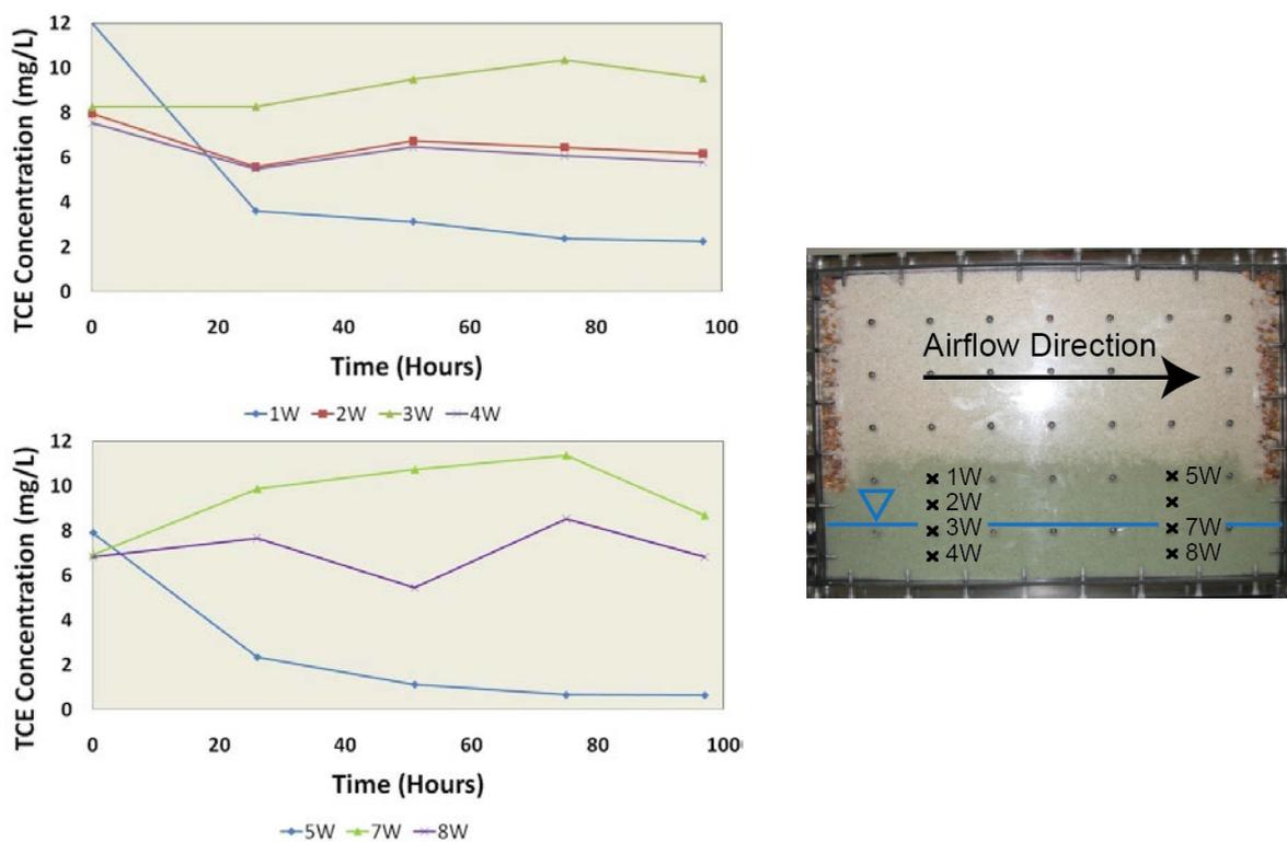
**Figure 5.7:** Aqueous TCE concentrations in the capillary fringe from experiment 3. Tank diagram at right shows locations of sample points. Water phase is dyed green for ease of viewing, while the vadose zone above the fringe appears as clean sand.
