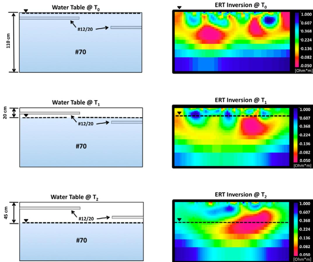
**Figure 5.42:** Schematic of packing configuration #3 and the ERT inversions with the water table set at the upper, mid and lower elevations (T<sub>0</sub>, T<sub>1</sub>, and T<sub>3</sub>, respectively). The ERT inversion color gradients represent resistivity values with ranges from 0.05 Ohm\*m to 1.00 Ohm\*m.
