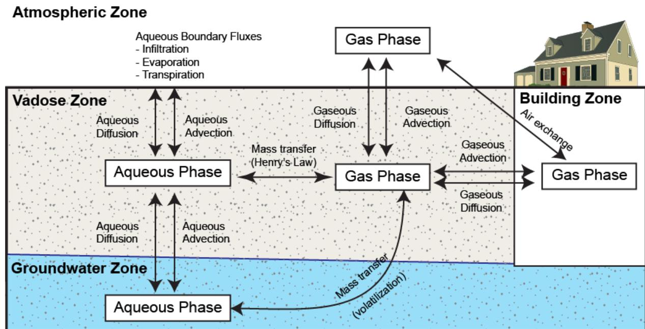
Figure 2.1: Process based conceptual model of the vapor intrusion pathway.
