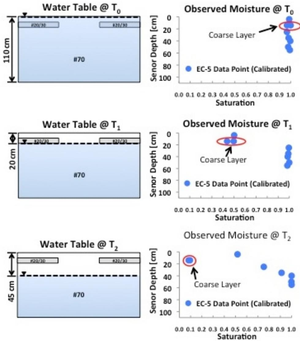
**Figure 5.35:** Schematic of packing configuration #2 and the calibrated volumetric moisture content data (e.g. Sakaki et al., 2011) with the water table set at the upper, mid and lower elevations ( $T_0$ ,  $T_1$ , and  $T_2$ , respectively).
