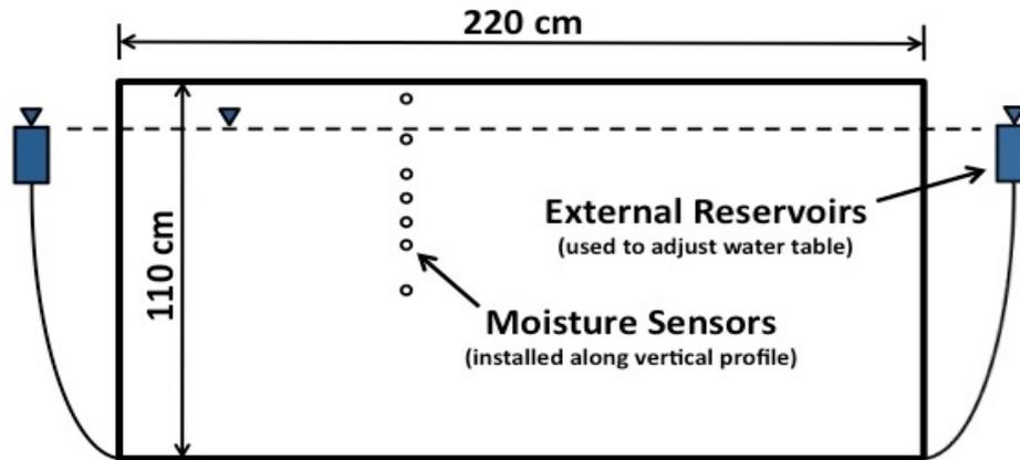
**Figure 4.12:** Schematic of the geophysical tank experiment apparatus with reservoirs used to control water table elevation and moisture sensors installed along a vertical profile. Moisture sensors were installed at vertical elevations of 4, 14, 25, 30, 35, 40, and 55 cm bgs (below ground surface). Total volume of sand tank apparatus is  $163,350 \text{ cm}^3$ .
