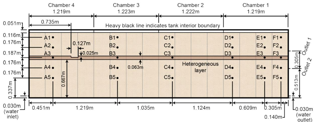
**Figure 4.10:** Detailed schematic of tank design and configuration.
