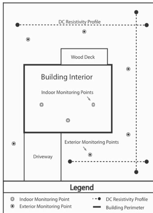
**Figure 4.15:** Schematic of VI monitoring locations with exterior and interior monitoring points indicated by concentric circles (oxygen concentrations, pressure potential, and soil gas sampling ports) and ERT profiles indicated by dashed lines with solid circular ends.
