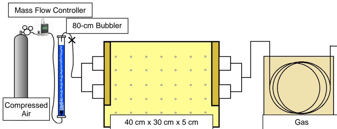
**Figure 4.3:** Schematic of capillary fringe volatilization experimental apparatus
