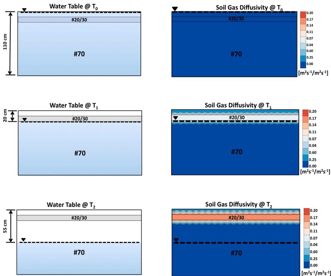
**Figure 5.37:** Schematic of packing configuration #1 and the soil gas diffusivity simulations (Moldrup et al., 2000) with the water table set at the upper, mid and lower elevations (T<sub>0</sub>, T<sub>1</sub>, and T<sub>3</sub>, respectively).
