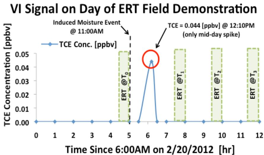
**Figure 5.47:** Graph of the VI signal (TCE in ppbv) entering study site building over 1-day window during our ERT field demonstration with ERT time-series snapshots overlaid on the VI signal timeline [Ongoing VI site study by Johnson et al., 2010-2012].
