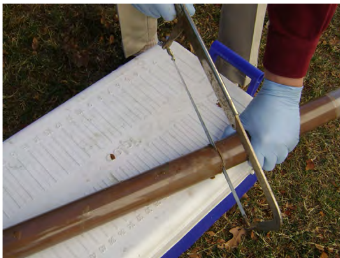
Figure A-3. A core sample acquired in a plastic sleeve is cut to access the core for sub sampling.
