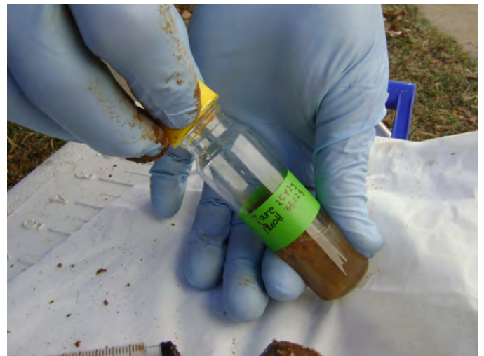
Figure A-8. The vial was sealed and shaken to disperse the subsample and began the extraction. Note that the empty weight of the vial and cap and the weight of the vial and cap plus methanol were recorded in the laboratory when the vials were made up. When the vial is returned to laboratory it is weighted again to determine the wet weight of the subsample.
