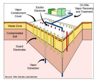
Figure 5. Radio-Frequency Heating with Electrodes
