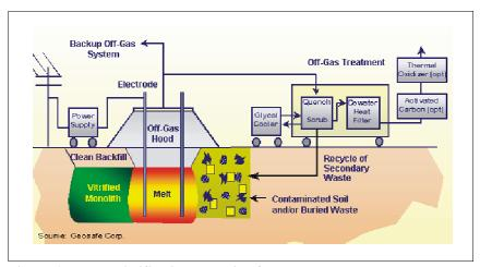
Figure 6. Planar Vitrification—Melting from the Bottom
