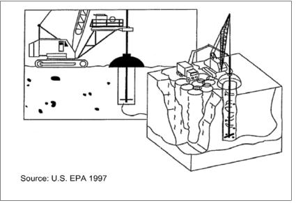
Figure 2. MecTool<sup>TM</sup> for Solidification and Stabilization of Contaminated Soils and Sludges
