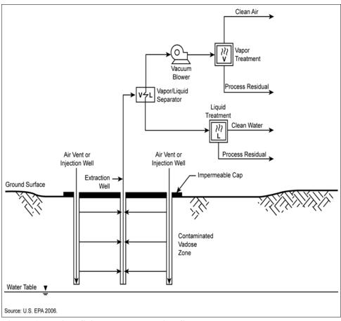
high preferential flow Figure 1. Typical Soil Vapor Extraction System
