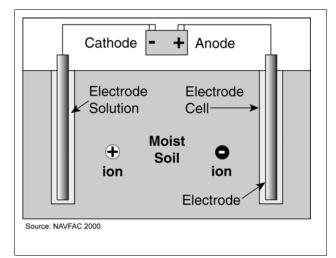
Figure 3. Simple Electrokinetic Separation System
