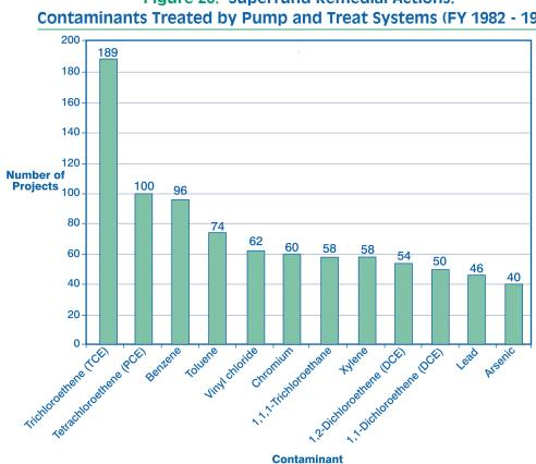
Figure 26: Superfund Remedial Actions: Contaminants Treated by Pump and Treat Systems (FY 1982 - 1997)
