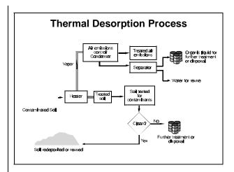
soil. The vaporized organics are then collected by condensation or carbon adsorption. Please note, however, that TD systems that vaporize and then burn organic contaminants are considered incinerators for the purpose of RCRA regulation—thermal desorbers may well meet RCRA definitions for incinerator, boiler, industrial furnace, or miscellaneous unit regardless of the operator's intentions.
