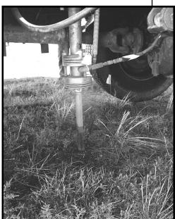
The SCAPS system deploys various subsurface diagnostic technologies using CPT tools to provide indirect characterization of subsurface petroleum hydrocarbons.
