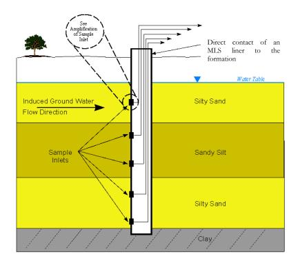
Cross-Section of a Multi-level Sampler Installation
