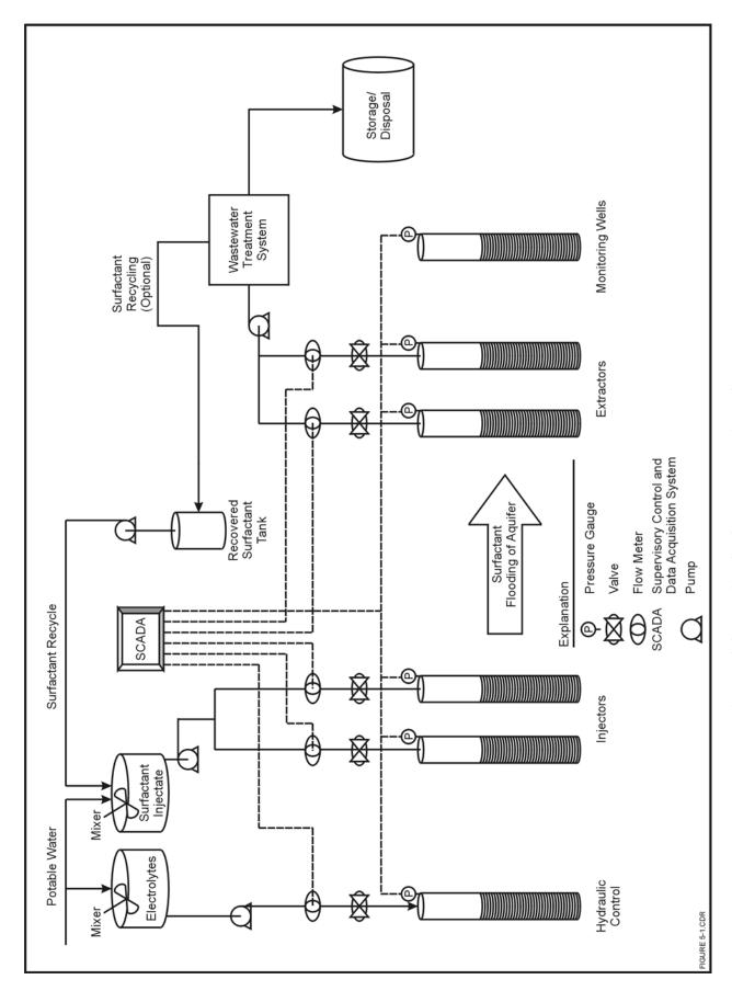
Figure 3-2. Basic Surfactant Flooding Components
