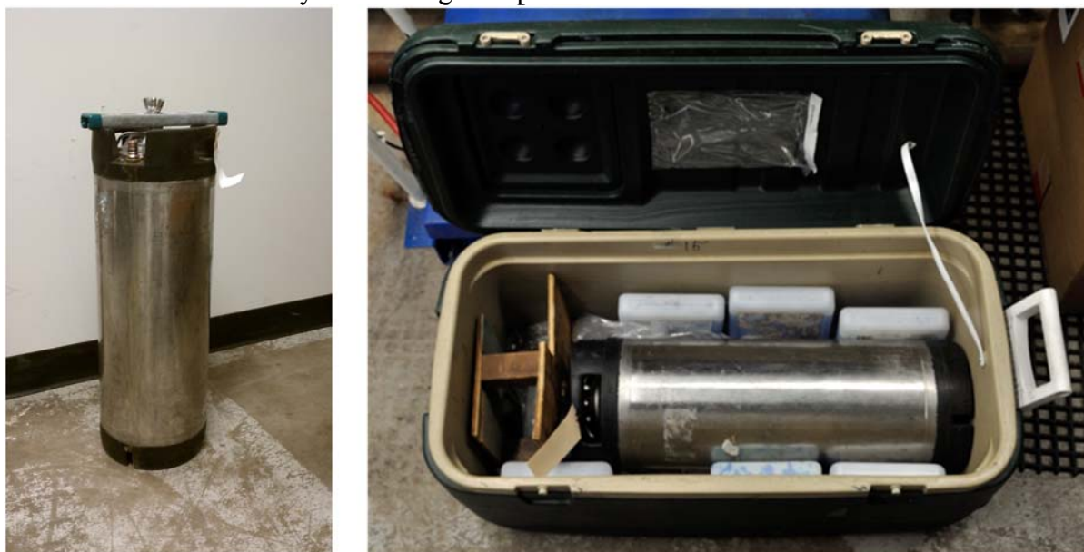
Figure 5.22. Photographs of 20-L soda keg used for culture starvation and shipping. The kegs were packed in ice prior to overnight shipment to the field in coolers.
