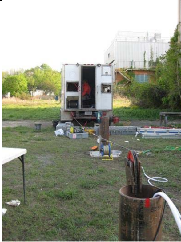
Figure 2. 5: USGS cross-borehole flowmeter logging at the NAWC site. Vertical flow in one borehole is measured during pumping from another borehole.
