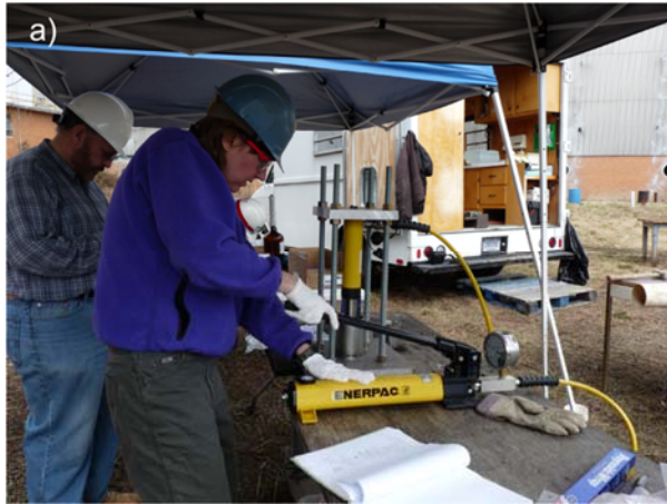
Figure 5.2.1. 6: a) Crushing of selected core samples and b) preservation of crushed samples in methanol for VOC analysis.
