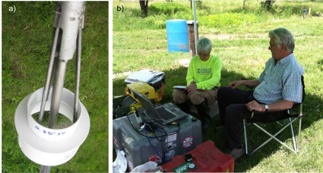
Figure 5.2.3.1: a) Caliper borehole tool b) Borehole geophysical data collection. All logs calibrated according to ASTM standards and USGS protocols.
