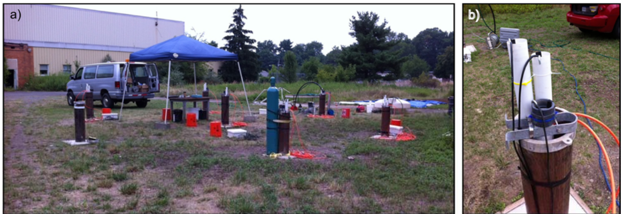
Figure 5.2.4. 1: a) Field setup for crosshole aquifer test on wells 83BR-89BR. Blue tank is nitrogen gas used to inflate the packers. b) Typical well setup where the three PVC pipes inside the wellhead give access for pumping and monitoring different isolated intervals.
