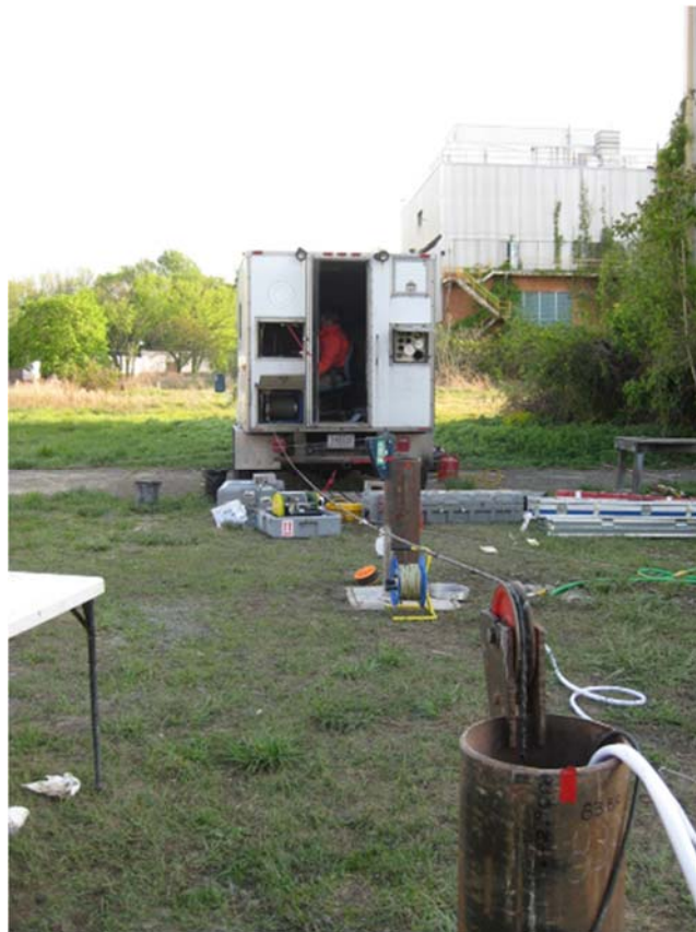
Figure 5.2.3.2: Cross-hole flowmeter logging whereby a single borehole is stressed with an injection while monitoring the down-hole response of three nearby boreholes with flowmeters. A metal casing extends above the ground surface at each borehole. This top of casing (TOC) was used as the datum for all geophysical logs.
