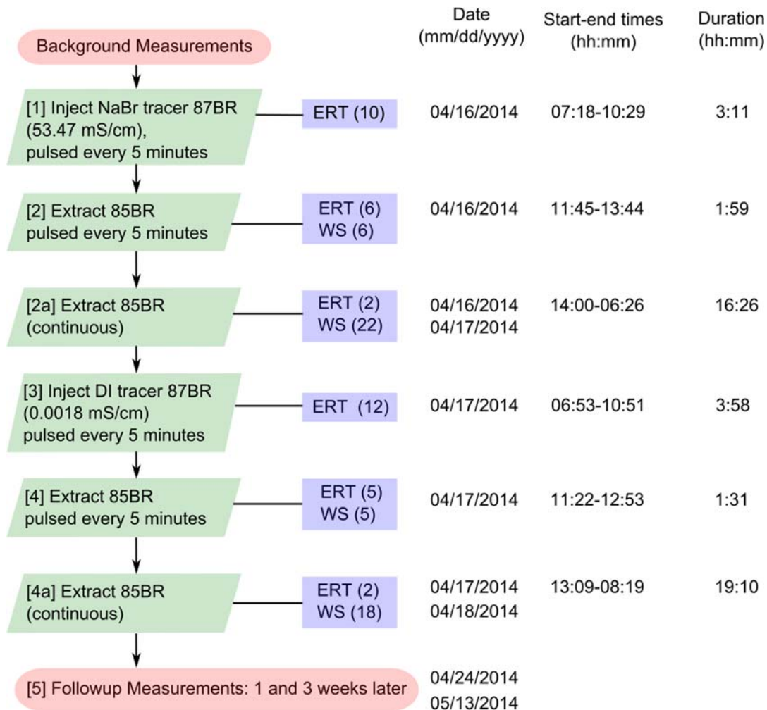
Figure 5.5.3 5: Flow chart of tracer test where numbers of ERT data acquisitions and water samples (WS) are indicated in parentheses ( ).
