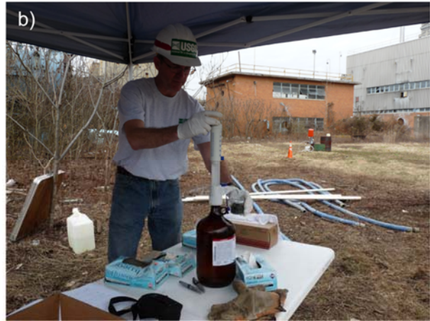
Figure 5.2.1. 6: a) Crushing of selected core samples and b) preservation of crushed samples in methanol for VOC analysis.
