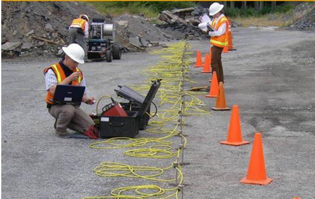
Figure 2.1-1. Field setup of ERI equipment. Metal stakes extend approximately 6 inches into the ground and are connected to an acquisition instrument via cables. Photo courtesy of Aestus, LLC.
