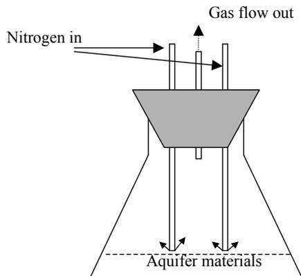
Figure 4: Anaerobic setup for drying aquifer materials.
