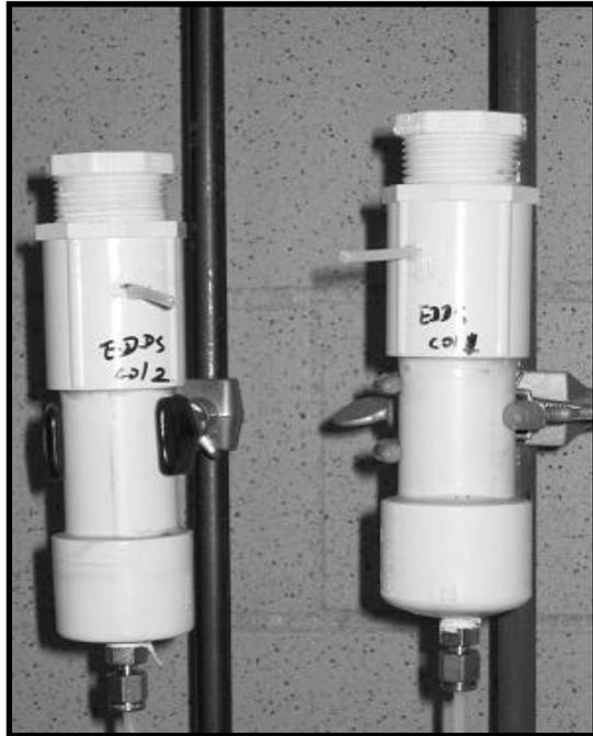
Figure 39: Typical setup for hydrogen peroxide column experiments.
